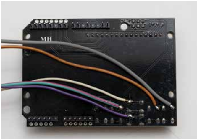
⑥ These wires connect the switches on the throttle's case with the LCD/keypad shield.
