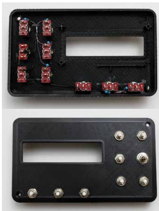
8 Add the switches to the case, and make the wire connections on the back.
