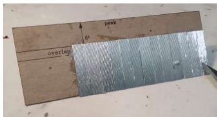
6 Cardboard and cardstock can be used as a subbase for siding.
