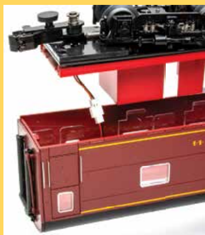
Lifting the frame from the body reveals the plugged wire for the LED lighting system.
