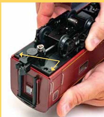
Two Phillips round-head body screws can be found on the under-frame at each end of the car.
