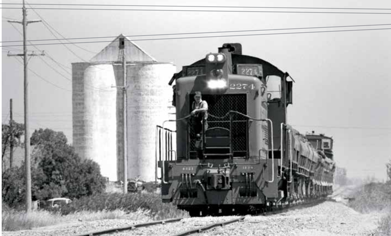
Head brakeman H. T. Hastings prepares to flag the SP lone Branch crossing at Herald as borrowed SP SW1200 2274 charges up to the diamond with a trainload of earth fill for the bridge 21b renovation project. Right: Engineer Jackson has the 1200-horse EMD in the company notch as the southbound work extra clears the SP crossing and recaptures its 25 mph gait.
