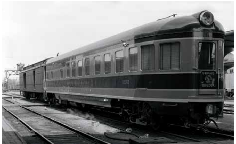
The Mountain series observation cars of the 1951 Builder featured high windows in the rear and interior decor that included solid drapes, hidden valance lighting, and carved glass partitions featuring the official flowers of the states and Canadian provinces served by the GN.
