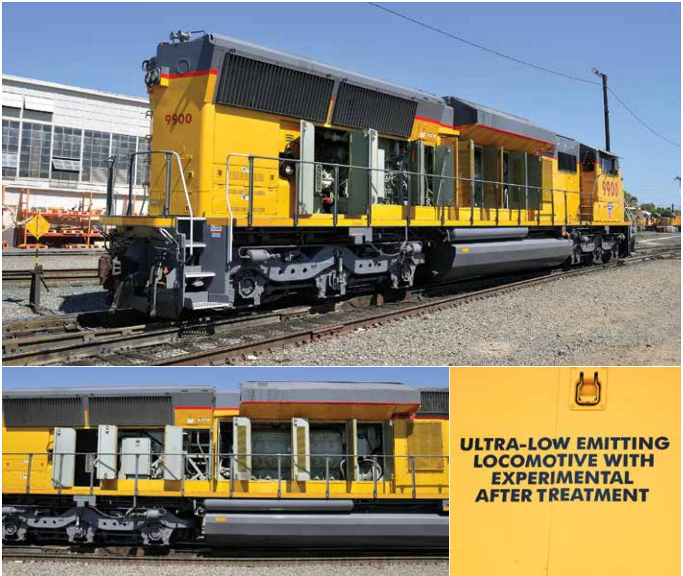
Delivered to Union Pacific in 2012 by Progress Rail's EMD subsidiary, the No. 9900 testbed locomotive was equipped with three different experimental emission-reduction technologies. The distinctive hump midway along the roof provided the space needed to install the equipment inside the body of the locomotive. The results of the 18-month test program were encouraging.
