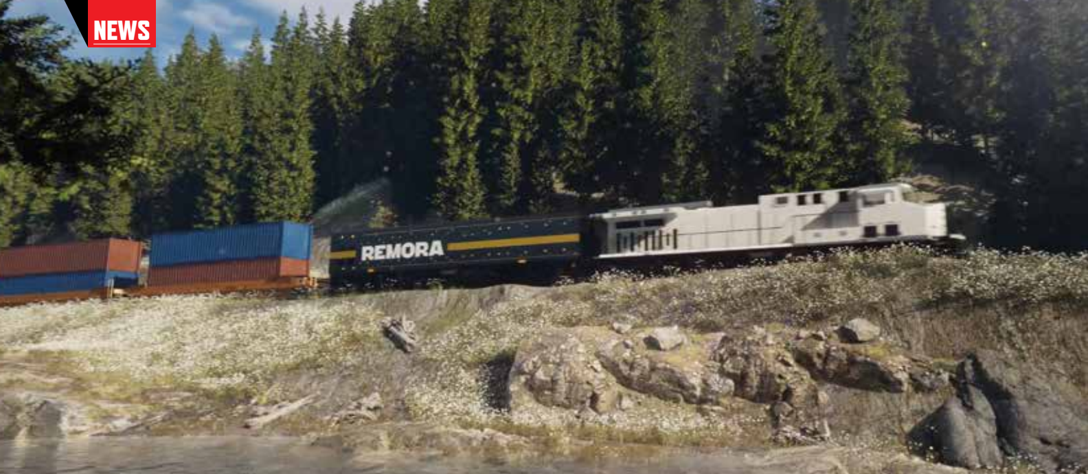
A rendering of a Remora carbon-capture tender, which would convert exhaust gases to liquefied carbon dioxide. Remora
