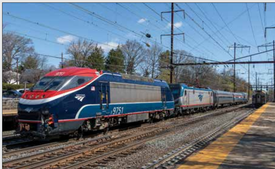
AN AMTRAK CREW-FAMILIARIZATION EXTRA featuring HHP8C cab cars, converted from Bombardier-Alstom electric locomotives retired in 2015, passes through Metuchen, N.J., on April 8, 2025. The former locomotives are nearing deployment in revenue service, allowing Amtrak to retire or bolster its fleet of ex-Metroliner cab cars for its increased push-pull operations on the Northeast Corridor. Adam Reich
