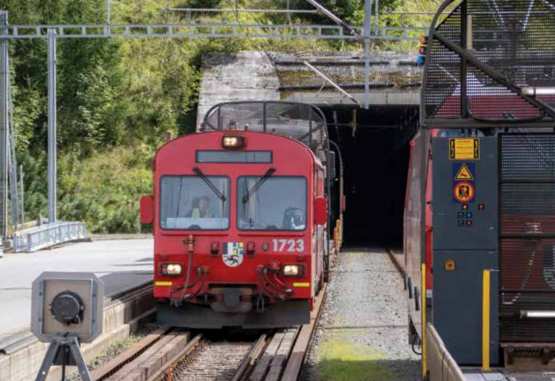
A cab car leads one of the transporter trains into the Selfranga terminal; immediately behind is the open flat car for large vehicles (with a truck onboard barely visible). Plans are replace the cab car with a locomotive, and to add more open cars to meet the demand for truck movements.
