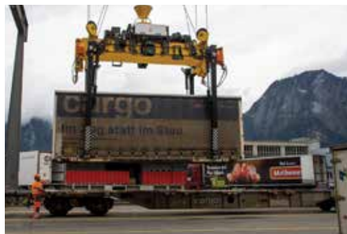
The largest Bündler Güterbahn terminal, at Landquart, includes one lift crane and one forklift-like restacker, here lifting a container tank for road salt. Only Landquart and Samedan have these large-capacity cranes.
