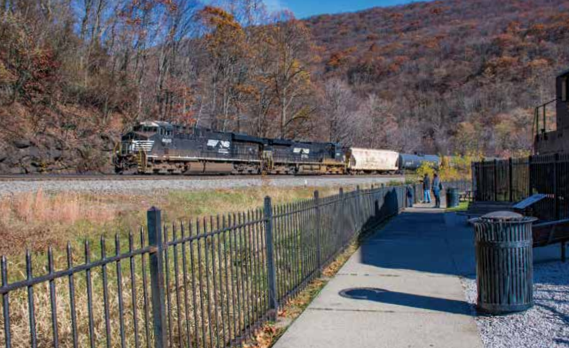
A westbound Norfolk Southern train of empty tank cars climbs the grade at Horseshoe Curve, kept to 1.86% thanks to the lengthy curve. Just visible at the right is former Pennsylvania Railroad GP9 No. 7048, on display at the trackside viewing site.
