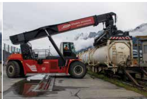
The largest Bündler Güterbahn terminal, at Landquart, includes one lift crane and one forklift-like restacker, here lifting a container tank for road salt. Only Landquart and Samedan have these large-capacity cranes.
