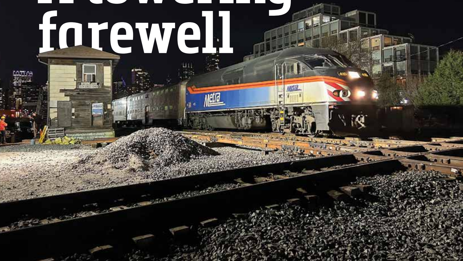
▲ Metra Rock Island District train No. 513 eases past 16th Street Tower at 9:34 p.m. on April 11, 2025. Wires to the signals had been disconnected for the cutover to remote operation about an hour earlier, leaving the tower's operator to talk the train through the crossing. David Lassen
