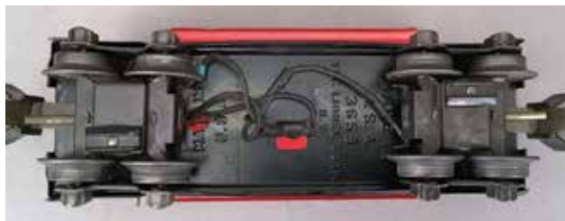
The underside of this No. 3659 Dump Car from 1939 shows the design of the collector shoes — truck-mounted power pickups needed to obtain electrical energy from track power.
