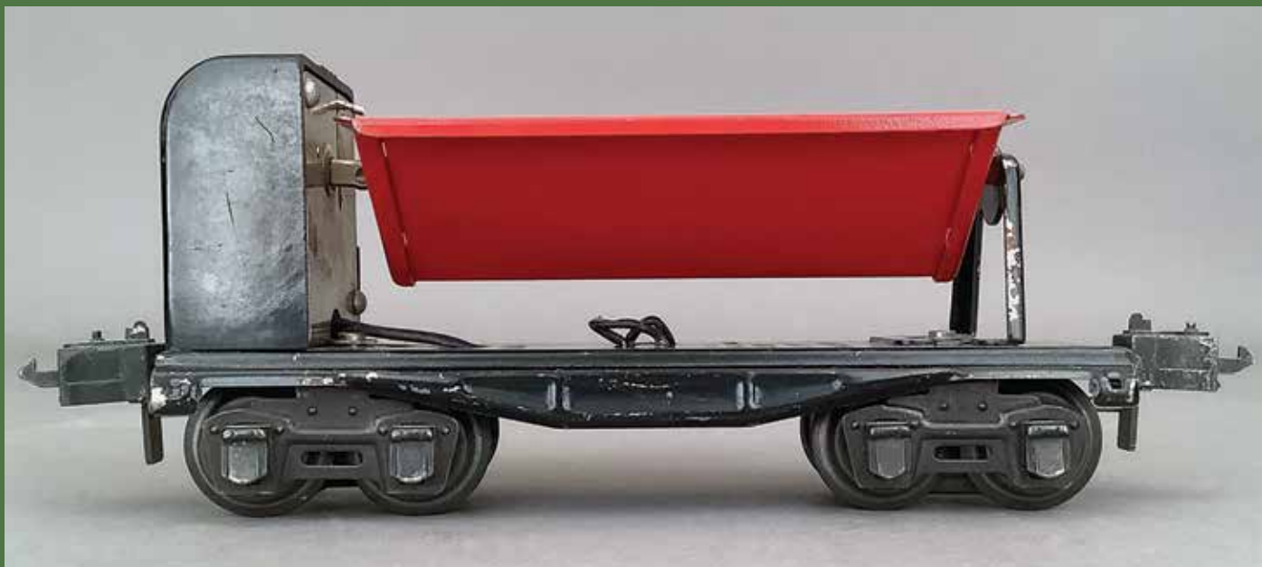
The Lionel No. 3659 Dump Car, introduced in 1938, came about after engineers saw how they could take advantage of the new system of remote-controlled uncoupling to devise a method for unloading by modifying the phenolic control box and the special track section.
