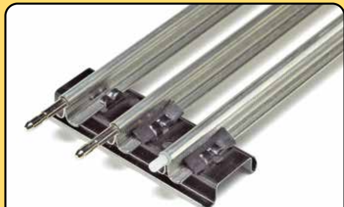
9 This section of Lionel O gauge tubular track has been converted to serve as an insulated track section. Note the short white plastic pin inserted into the outer rail.
