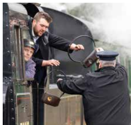
Spa Valley crews perform a classic token exchange on the fly at Groombridge. Engine crew passes the token from the previous section to the signalman while snatching one for the next section.
