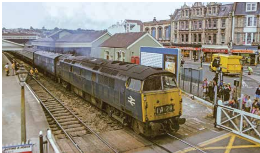
The 2,700-hp "Western" six-axle diesel-hydraulics were the last and most powerful to be built. D1046 Western Marquis departs Paignton in southwest England with the 2 p.m. train to London Paddington in June 1975. John Harrup, Keith Fender collection
