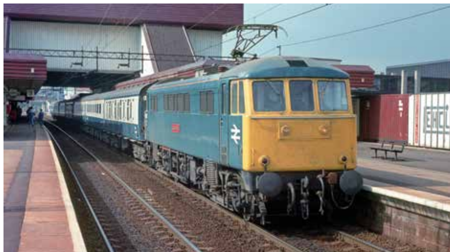
The most numerous electric was the BR type AL6, later the Class 86 25kV A.C. four-axle motor. One hundred were built 1965-66 for use on the West Coast Main Line and later were moved to other electrified routes. No. 86233 is at Birmingham International on April, 20, 1985. Keith Fender
