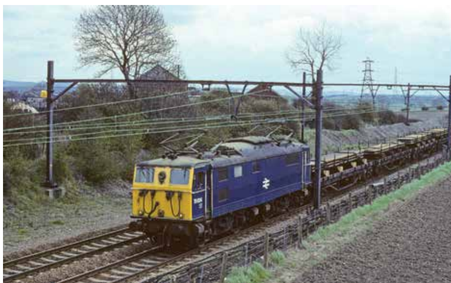
For the 1954 Manchester-Sheffield electrification, BR ordered 57 four-axle 1,300-hp electric locomotives, based on a pre-war prototype. No. 76024 leaves Wath near Sheffield with a train of steel on May 8, 1979, during the final year of operation. John Harrup, Keith Fender collection
