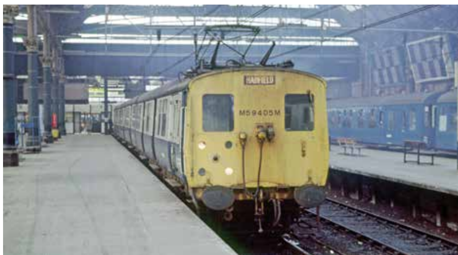
Passenger EMUs were also built for the Manchester-Sheffield electrification. The units remained in use at the Manchester end of the otherwise closed mainline until 1984, when the line was converted to 25kV AC. One poses at Manchester Piccadilly on Dec. 3, 1983. Keith Fender
