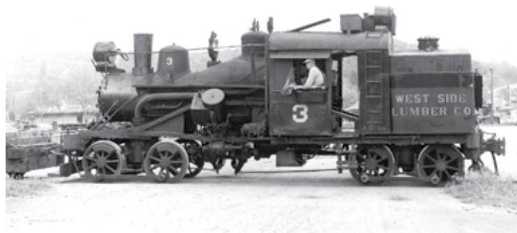
No. 3 is a two-truck, 37-ton Heisler built in 1900 for West Side Flume & Lumber Co. It was converted to standard gauge in 1947. Glenn W. Beier
