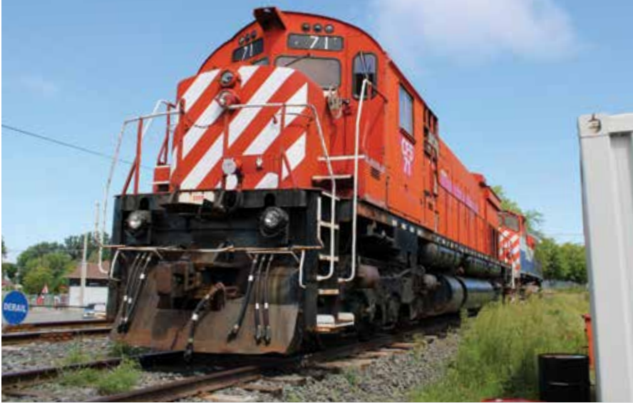
Sartigan's newest locomotive, No. 71, rests in the sun just north of the company's shop in Scott on Aug. 6, 2024. The M636 was a unique rebuild project that resulted from a partnership between Canadian Pacific and Caterpillar. Harrison Smith
