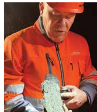
Tunnel project manager Paul Loser discusses a piece of lining that has fallen from the ceiling of the old Albula tunnel.
