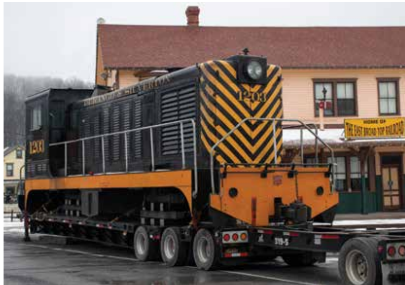
An 80-ton H.K. Porter diesel acquired from the Durango & Silverton Narrow Gauge Railroad arrives at East Broad Top headquarters in Rockhill Furnace, Pa. The locomotive will aid EBT expansion efforts and provide a more powerful backup for its steam engine. Dan Cupper
