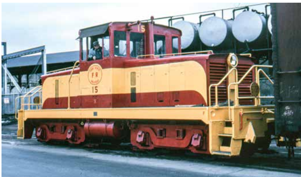
Fore River No. 15, a GE 70-tonner, photographed on March 21, 1962. The oddball 600-hp locomotive has four diesel engines, two under each hood. Ralph L Phillips, author's collection
