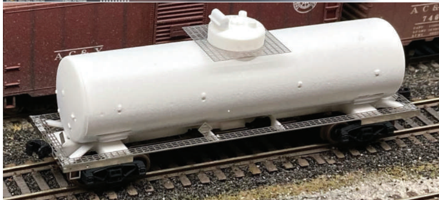
⑤ Finished product. With the artwork completed, Steve sent the electronic files to PPD Ltd. in England, where the parts were etched from .125mm stainless steel sheet (top). He reports a huge sigh of relief was audible throughout the house when it was confirmed the parts fit as intended (bottom).
