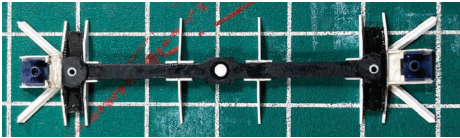
③ Body-mounted couplers. The Bachmann chemical tank car uses truck-mounted couplers. Steve added draft-gear boxes to the tank car frame he used as a master for making copies in resin. He also filed the bolster blocks.
