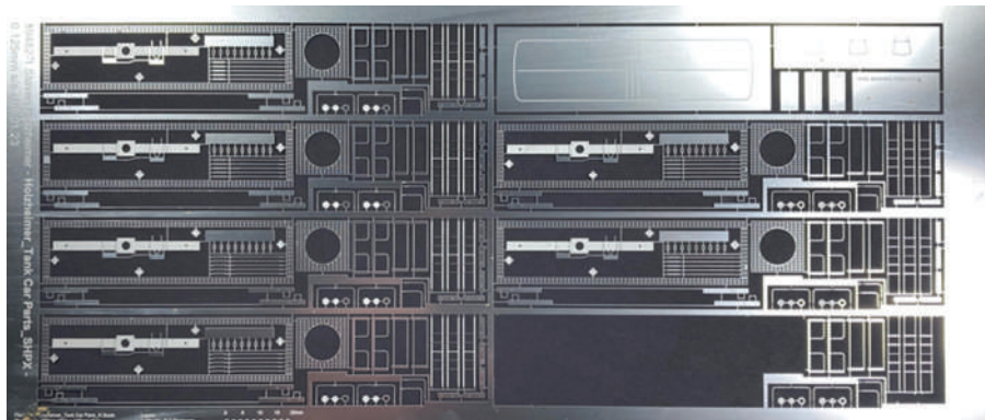
④ Test time. Steve turned to etched-metal parts for the walkways and dome platforms. He printed the artwork and placed it on the model to make sure everything would fit before sending the files off for production.
