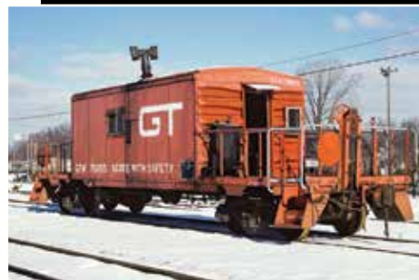
Grand Trunk Western transfer caboose 75055 was rebuilt from a boxcar, providing a warm, dry place to ride during rough weather. Jim Hediger
