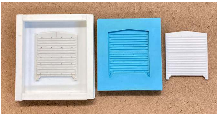
3 Making copies. With the end pattern finished, Paul made a styrene mold box (left) and filled it with Micro-Mark's 1-to-1 rapid mold rubber (center). One of the completed ends, made with CR-600 casting resin, is shown at right.
