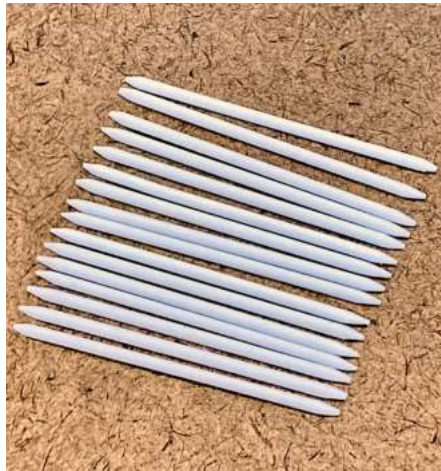
2 Rack of ribs. The ribs for the refrigerator car ends are lengths of .060" half round. Paul tapered each piece with a No. 2 file, 400-grit sanding cloth, and "a lot of eyeballing."
