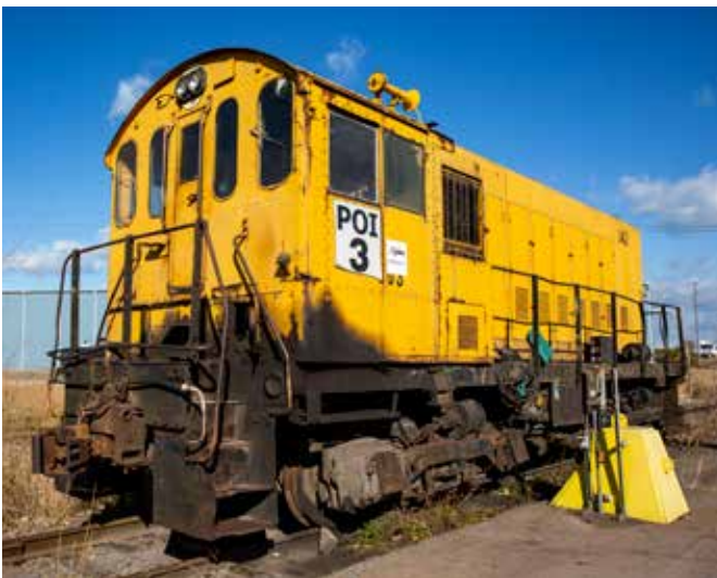
Laboring in relative obscurity, NIWX HH660 is one of the most historic locomotives in the country. Turned out of Schenectady in April 1940 as DL&W 409, it's the oldest Alco diesel in revenue service. Greg McDonnell
