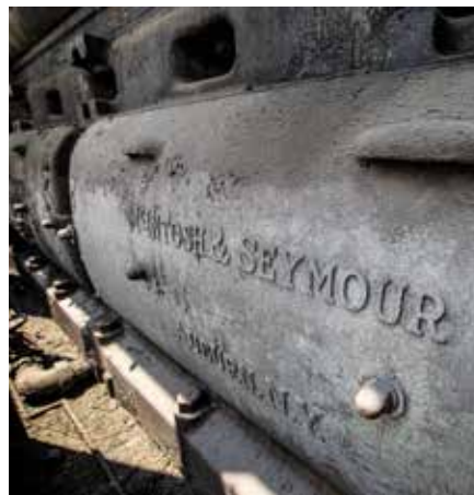
Behind the yellow hood doors of the 79-year-old HH660 is the real thing, an in-line, six-cylinder, 660-hp McIntosh & Seymour 539 engine.
