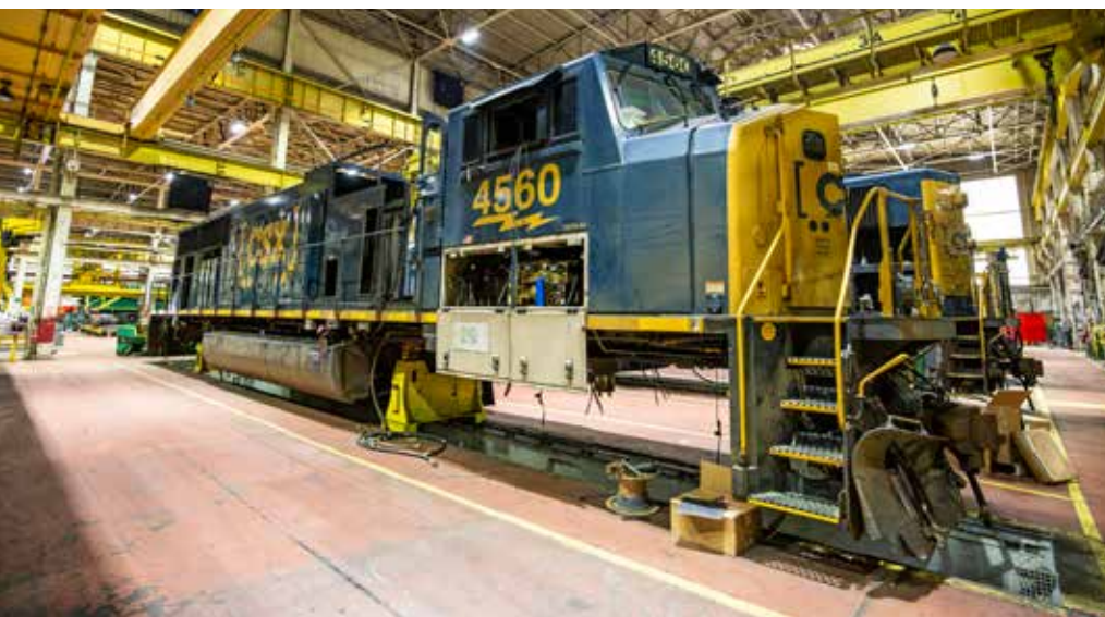
Add CSX to the list of railroads engaged in major rebuilds of modern power. Part of a program to upgrade SD70MACs to SD70ACe specs in its own shops, CSX No. 4560 undergoes conversion at Huntington, W.Va. Marshall W. Beecher
