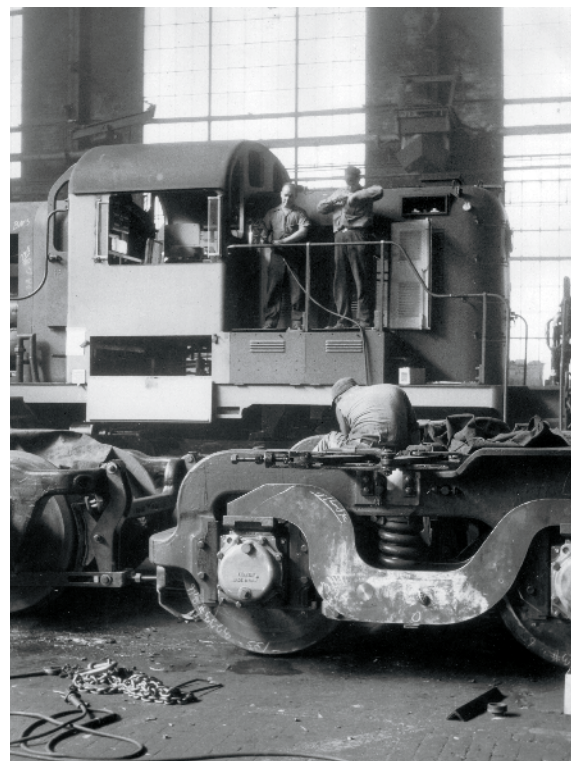
A worker readies the trimount truck for a Ferrocarril del Pacifico RSD5 while others work on an RS3 on the Schenectady floor in November 1953.
