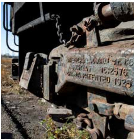
"American Locomotive Co. US Patent 15125/6." Alco staked its claim to the Blunt truck and cast it in the heavy steel frame. Three photos, Greg McDonnell
