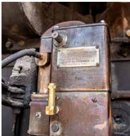
No. 603 was sidelined when its venerable Woodward SI governor blew a seal in 2018. LocoDocs Inc. made it right.
