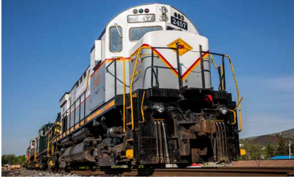
Better than new. D-L C425 No. 2457, completely rewired and upgraded with a 251F engine and GTA11 alternator, gleams in the morning light at Dickson, Pa.
