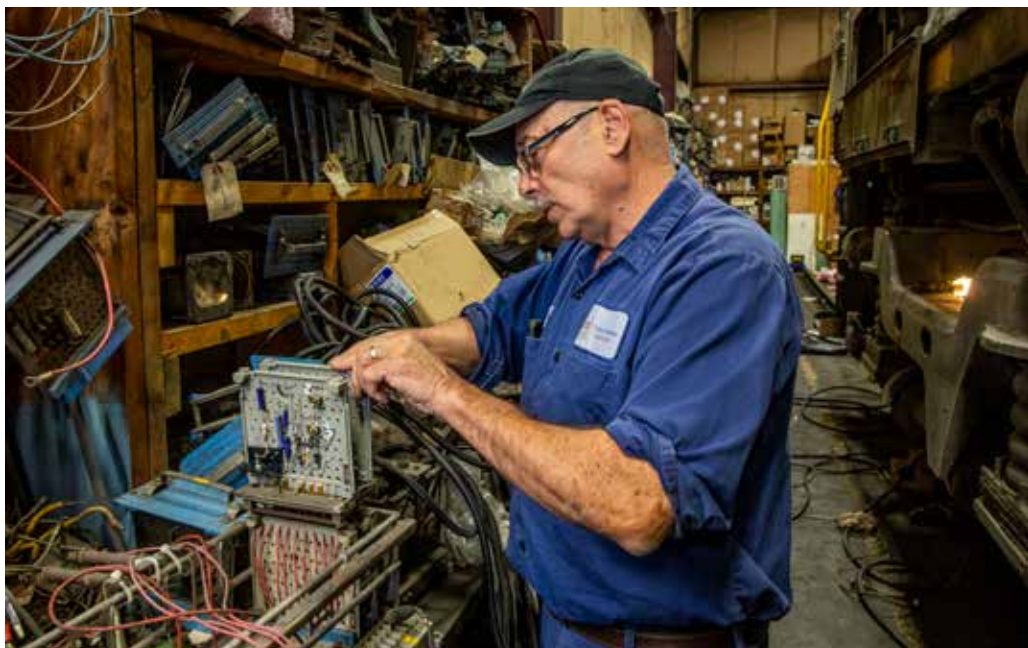
Right: Putting some of his mechanical and electronic wizardry into practice, Don Colangelo tests and adjusts a Type E blue card from a C420. "This is the brains of an Alco."
