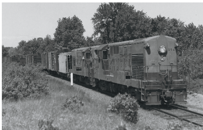
New Haven operated diesels from six builders, including 37 units from Fairbanks-Morse. Two H16-44s lead a train just south of Avon, Conn., on New Haven's Canal Line in June 1953. Barclay Robinson Jr.
