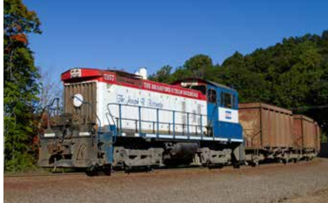
Definitely not steam: Branford Steam Railroad SW1001 No. 7357 leads a loaded stone train on the line serving a quarry at North Branford, Sept. 23, 2013.
