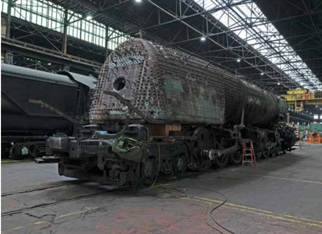
UP Challenger No. 3985 has been stripped of its piping, appliances, and cab in preparation for the boiler to be lifted off the driving wheels. Work on the locomotive has revealed the different maintenance techniques employed since it entered service in 1943.
