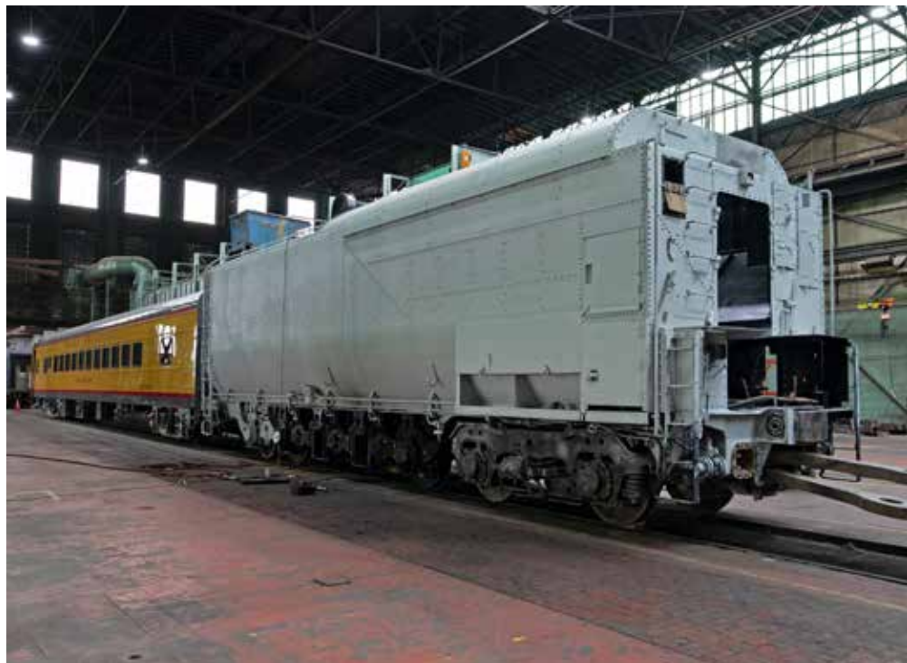
The terms of Union Pacific’s equipment donation included RRHMA rebuilding Big Boy No. 4014’s original tender and converting it from carrying coal to oil. Currently, No. 4014 uses No. 3985’s tender. In early 2024, the Big Boy tender was repainted in primer at Silvis.
