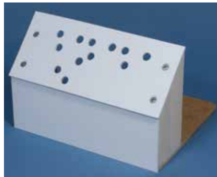
5 The finished box. Glue and screws were all Gerry needed to assemble the box. He later painted it the same color as the fascia so it would blend in with his layout.
