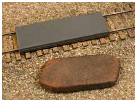
An extra-fine Cratex block (top) and Walthers SceneMaster Bright Boy (bottom) are two types of abrasive blocks used for track cleaning. Paul J. Dolkos photo
