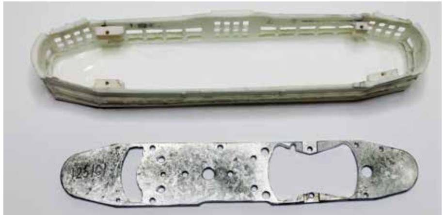
② Making modifications. Here are the changes that Harvey made to the floor. Note the holes drilled in the floor that mate with the four small chunks of resin that were glued to the shell.
