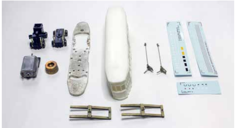
① Project overview. These are the parts Harvey used to build the streetcar. From left to right: Bowser power truck, trailing truck, and motor; A-Line flywheel; Bowser floor; Miniatures by Eric shell, rooftop parts, and trolley poles; and Rail Graphics decals. Harvey bought many of these parts from CustomTraxx.
