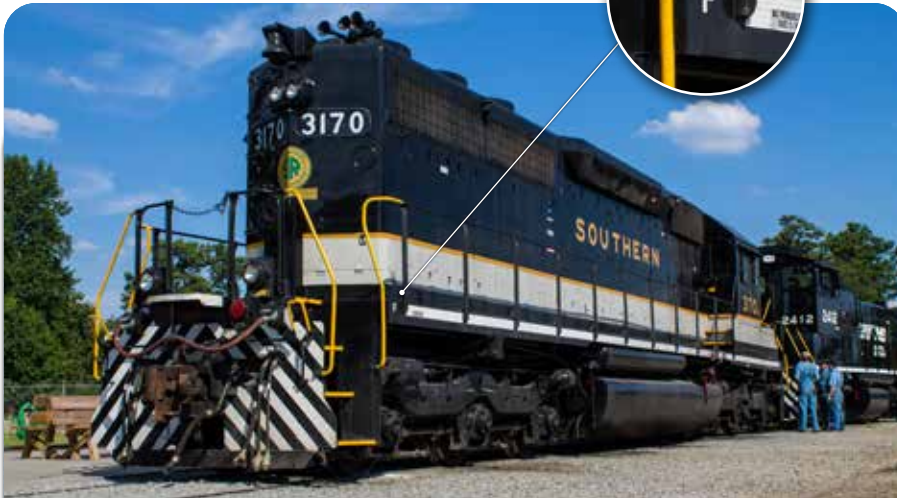
Manufacturers often mark an F on the front of a diesel, like the one on the sill of this Norfolk Southern EMD SD40. This Southern Railway heritage unit is marked to show it's configured for long-hood-forward operation. Kyle Yunker photo
