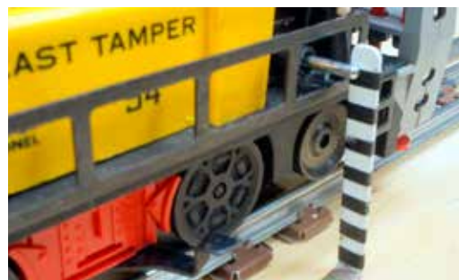
Figure 4. The final step involves making the trip lever. First, you bend the brass strip to form an L-shape. Then you drill a small hole for the screw that will secure the painted lever to the platform.
