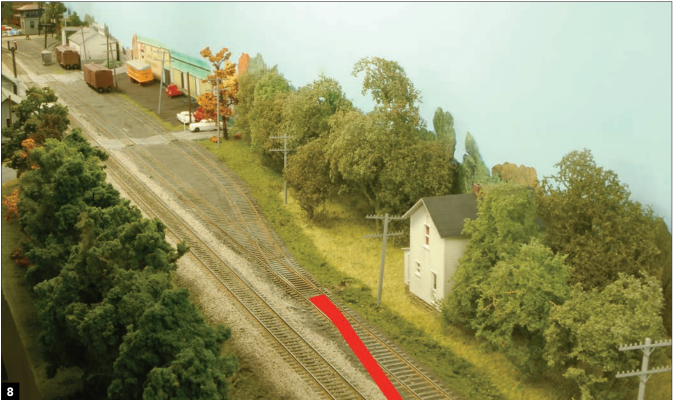
8 To pick up westbound cars at Veedersburg, Ind., the Nickel Plate’s westbound local (oddly, there was no eastbound local on the Third Subdivision) has to pull them off the interchange or team track and run east to the end of the passing track to get around them and shove them onto its train. A crossover (red) would have made this easy—and in fact one was there until the late 1940s!
