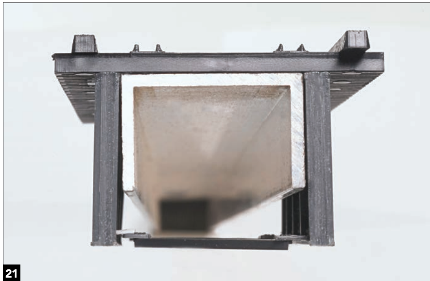
An aluminum channel (designed to dress up the edges of \frac{3}{4} " plywood) can form the core of most deck-girder bridges. The girders are then strictly cosmetic, and work on supporting abutments, towers, bents, or piers can wait for another day.
