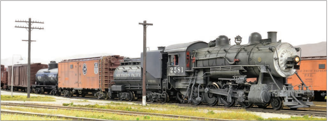
Brian Moore models the Guadalupe Sub of the Southern Pacific's Coast Division in 1954 when most local freights were hauled by 2-8-0s. Brass being beyond his budget, he used Bachmann's Consolidation to create "close enough" versions. SP 2581 has a reworked front end and cylinders, simplified valve gear, modified piping and handrails around the smoke box, new front dome, and a Bachmann coal Vanderbilt tender converted to oil. Brian Moore
