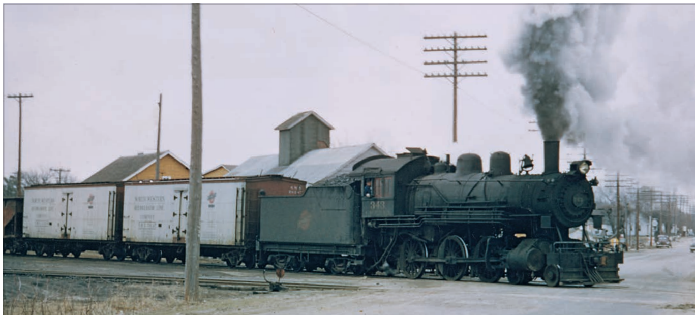
The Omaha used Ten-Wheelers (Class I-1 no. 343 here) extensively throughout its system. Linn Westcott
