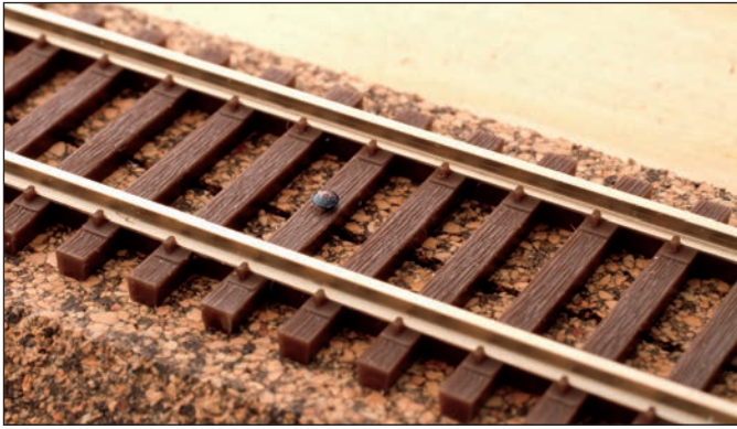
It's wise to lay conventional track atop roadbed such as cork. Small track nails will hold sectional track securely if a plywood tabletop or subroadbed is used.
