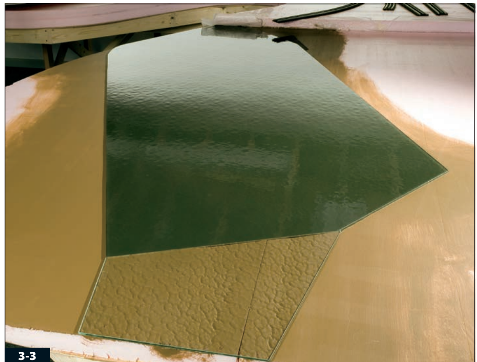
There is a clear difference between the painted glass (top) and unpainted glass. Painting the back of the glass causes the glass to act like a mirror.
