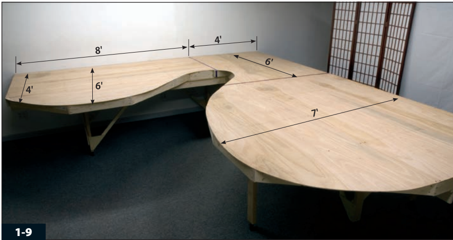
1-9 The tabletop consists of three sections made from five sheets of plywood. Two 4 x 8 sheets fit lengthwise along the rear of the benchwork. The center sheet is cut to 4 x 6. The other two sheets, extending into the interior, are trimmed and rounded to fit the track.
