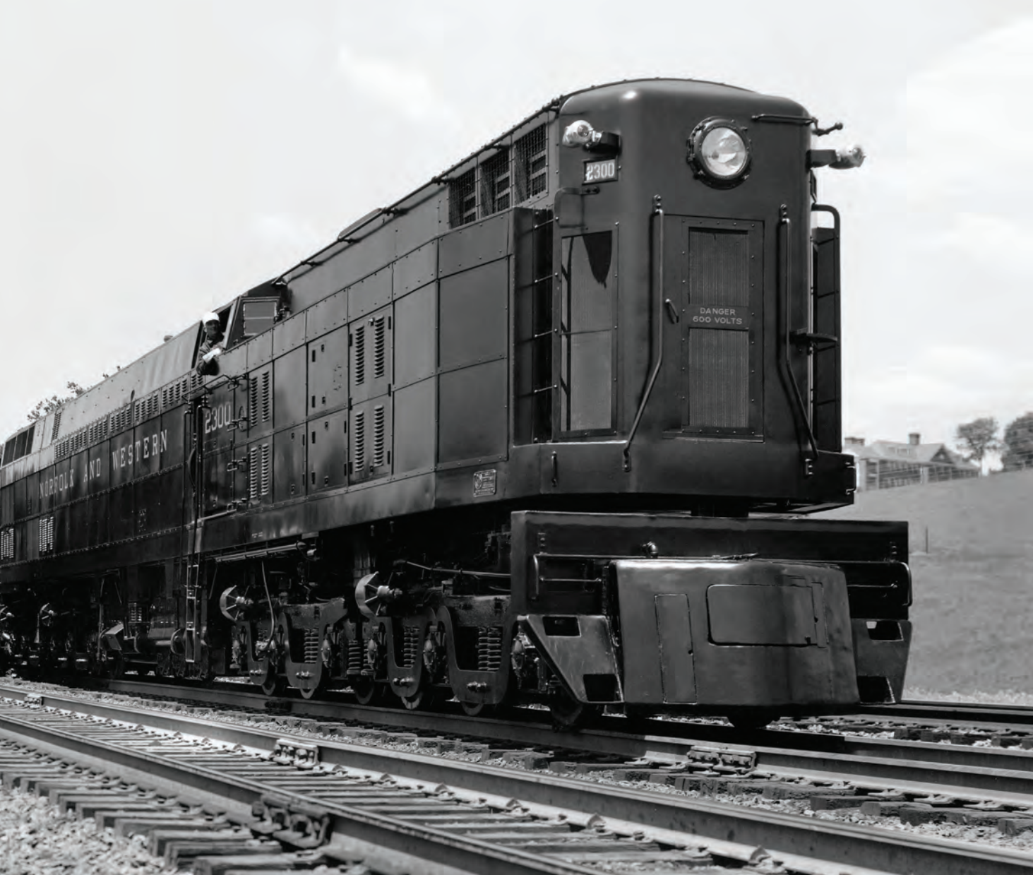
TE-1 No. 2300 makes an early appearance with Class J 4-8-4 No. 605 in Roanoke, May 17, 1954. The TE-1 was designed to haul heavy coal trains from the mines to tidewater for the Norfolk & Western Ry. Norfolk & Western Historical Society
