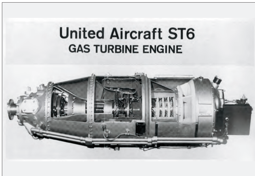
Called a "free turbine engine," the United Aircraft ST6 400 horsepower gas turbine had separate shafts for the air compressor and its turbine and the output turbine. Each engine weighed only 300 pounds, significantly reducing the weight of these trains. United Aircraft Corporation
