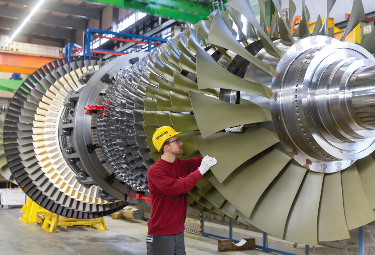
A worker examines an initial compressor blade in the engine's multi-stage axial compressor during assembly of a Siemens SGT5-8000H gas turbine. The large blades in the foreground compress inlet air prior to the combustion section. Smaller blades at the rear of this assembly create rotation from the expanding air/fuel mixture after combustion. Precision machining and material strength are critical to efficient and long-lasting turbines. Design improvements that produce incremental gains in life expectancy and fuel economy are closely guarded trade secrets of the few manufacturers worldwide. Siemens
