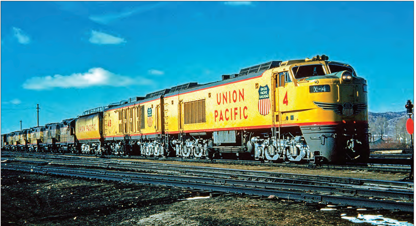
UP Big Blow No. 4 is at Evanston, Wyo., on March 11, 1962. Close inspection reveals that this 8,500 horsepower turbine is followed by six 1,750 horsepower GP9s for a total of 19,000 horsepower. It's unlikely that all this power could be used at low speeds because the tractive effort would likely break one of the couplers on the train. Collection of Chris Zygmunt
