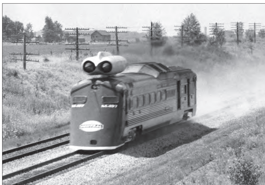
The New York Central wanted to test the physics of high-speed trains on jointed rail and used a jet-powered Budd Rail Diesel Car to go more than 180 mph. Tom Miller
