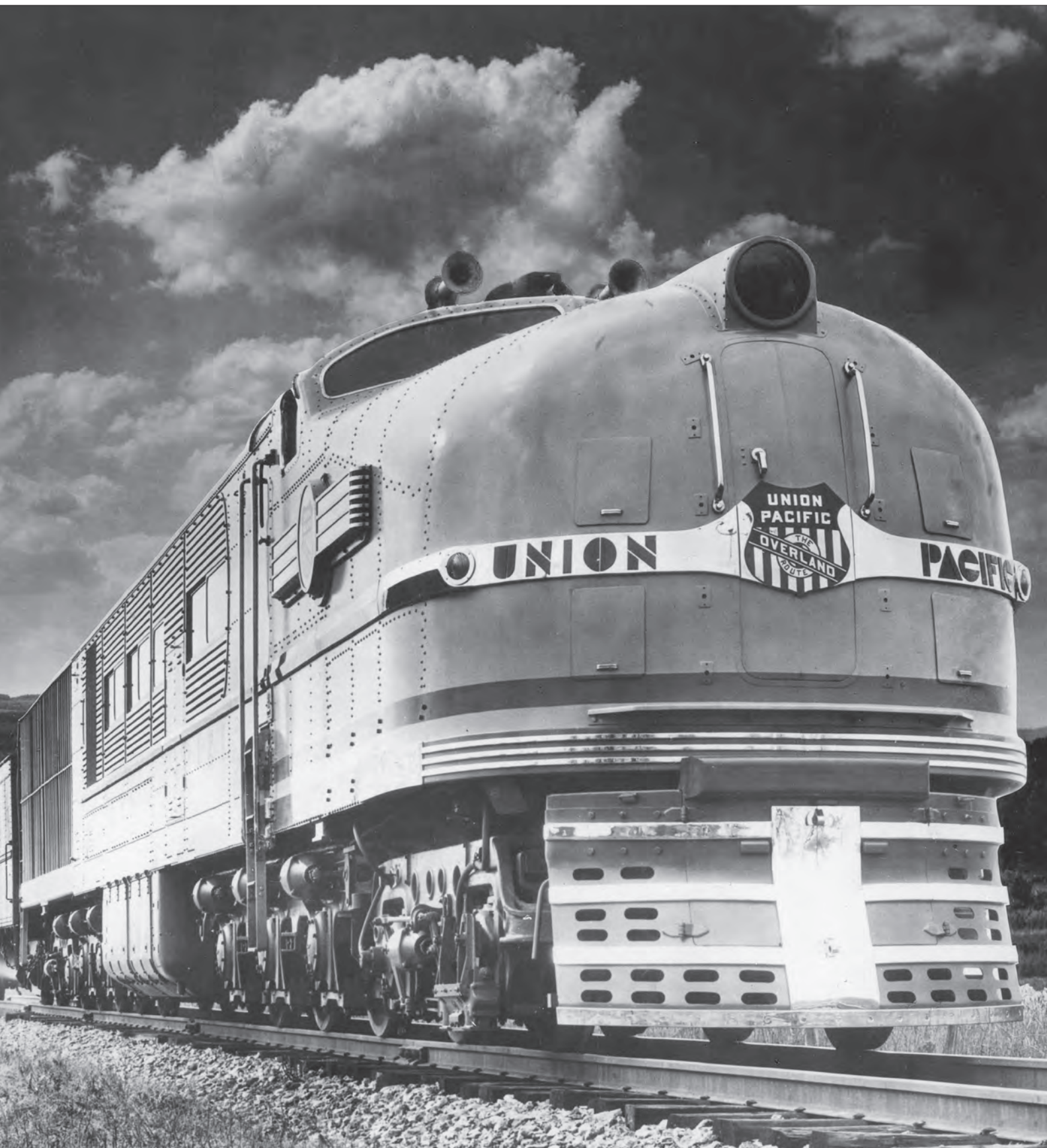
The Union Pacific oil-fired STELs were designed to pull passenger trains at over 100 mph across the Midwest, and up 2.2% grades in the West without helper locomotives. This image was a popular one for advertising. Union Pacific/Trains magazine collection
