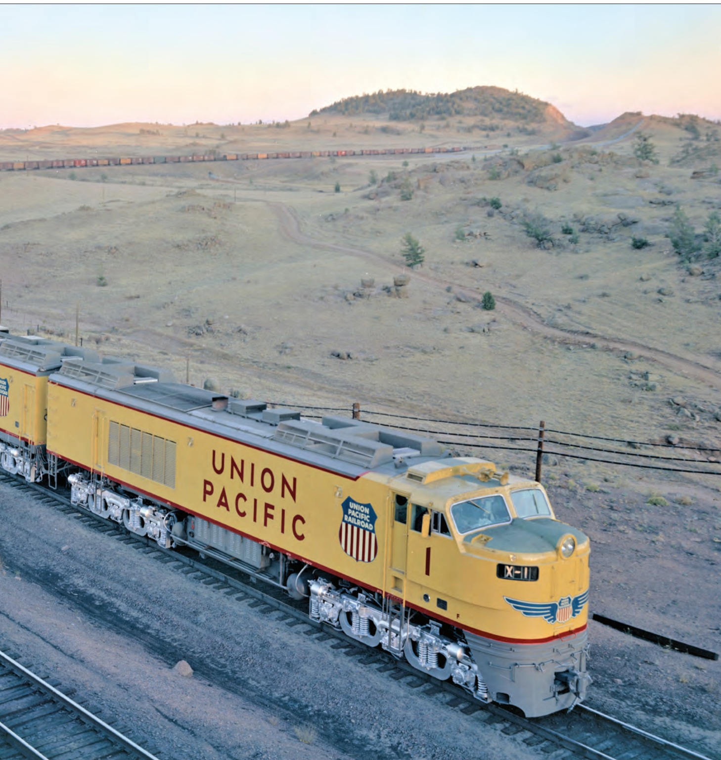
A Union Pacific 8,500 horsepower "Super Turbine" at Dale, Wyo., heads toward Sherman Hill. The gas turbine engine is located in the locomotive's second unit. The third unit is the tender carrying up to 24,000 gallons of fuel oil, compared to 3,000 gallons for diesel-electric freight locomotives of the era. Union Pacific Railroad Museum
