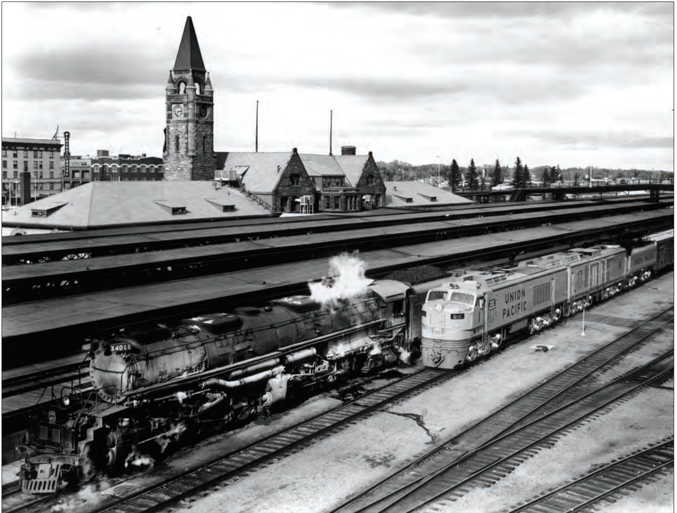
Giants meet in 1956 at the Cheyenne, Wyo, station—a UP 4-8-8-4 “Big Boy” steam locomotive and a super turbine. The super turbines produced nearly double the horsepower of the Big Boys. Union Pacific Railroad Museum/David P. Oroszi collection
