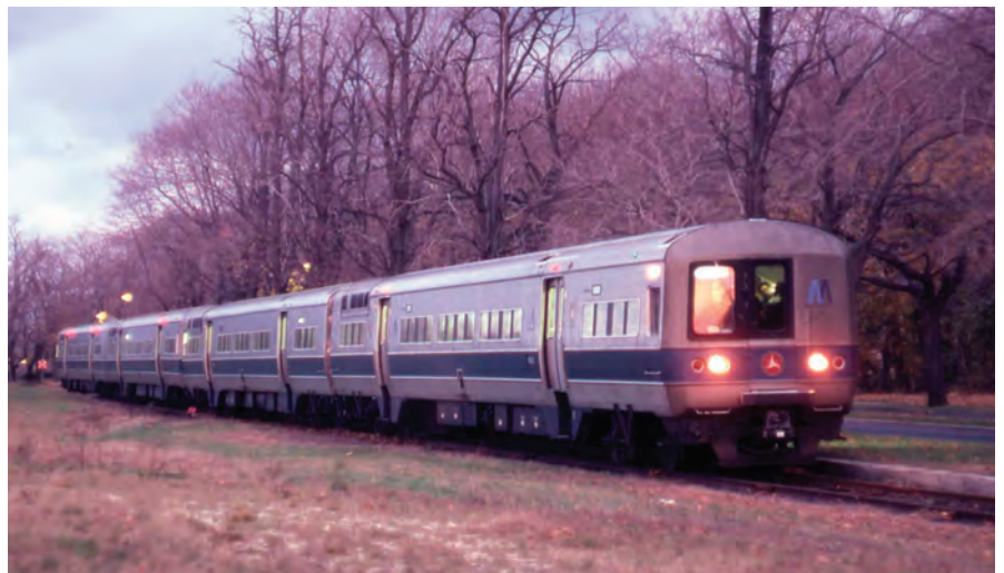
An LIRR four-car GT/E commuter train passes Kings Parks State Hospital, on Nov. 11, 1977. The turbine vents at the top of the second car indicates this is a train of Garrett GT/E cars. David Keller Archive
