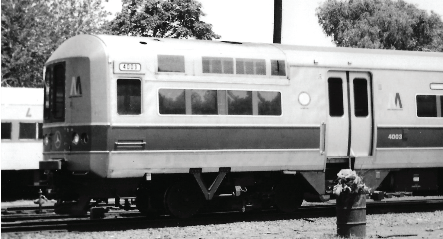
Long Island Rail Road No. 4003, a Garrett GT/E car, is at Oyster Bay, N.Y., July 2, 1977. Gas turbines were at a disadvantage with the long idle times typical of commuter equipment. George E. Votava, Mike Boland collection
