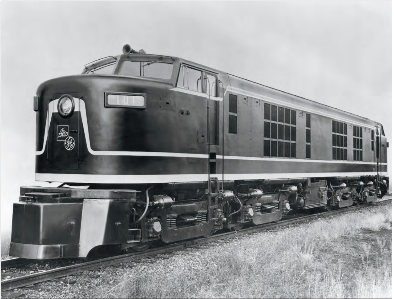
The first gas turbine-electric locomotive (GTEL) in the United States rolled out of the General Electric Erie, Pa., shops in 1948. Its successful testing on the Union Pacific led to orders for 55 more GTELs. General Electric
