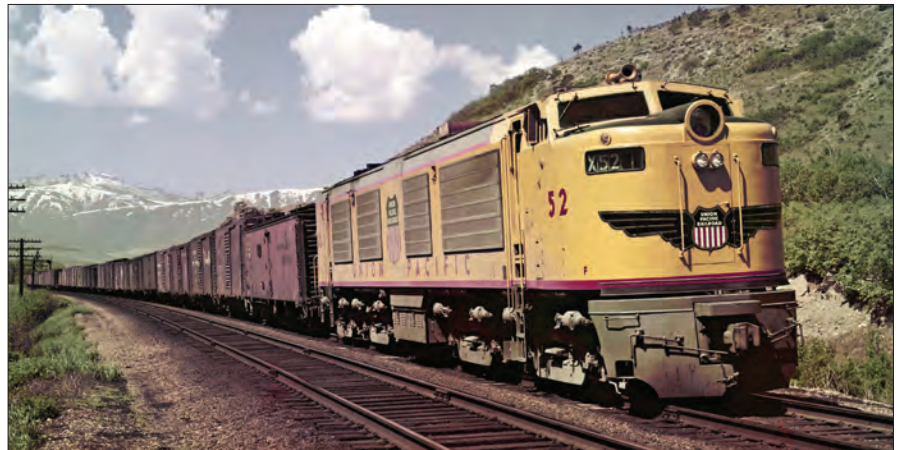
Union Pacific No. 52 leads a freight train through Weber Canyon in the Wasatch mountain range near Ogden, Utah. This first-generation UP GTTEL was equipped with a 4,500 horsepower gas turbine engine, which produced 137,930 pounds of starting tractive effort and 105,000 pounds of continuous tractive effort at 12.9 mph. Maximum speed was 65 mph. Its onboard fuel tanks carried 7,200 gallons of Bunker C fuel oil and 1,000 gallons of diesel fuel. Union Pacific Railroad Museum
