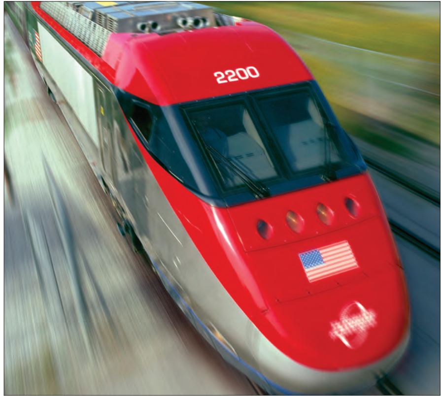
The Bombardier JetTrain was proposed to bring high-speed rail to non-electrified routes. It was put through its paces at the Transportation Technology Center in Pueblo, Colo. During testing, the locomotive with three passenger cars reached 156 mph. Bombardier Transportation
