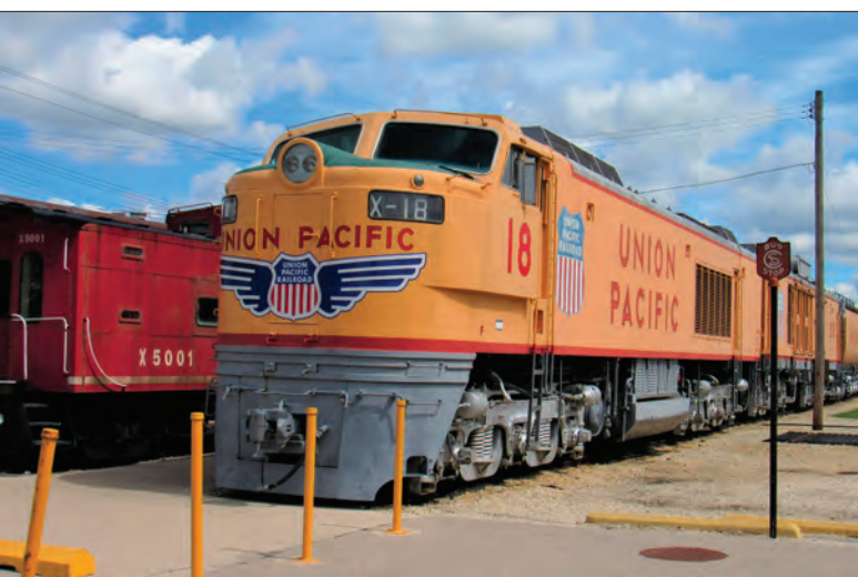
Number 18, one of only two remaining UP super turbines, is preserved at the Illinois Railroad Museum. This two-unit locomotive was rated at 10,000 horsepower and equipped with a 24,000 gallon tender. Signs at the museum note the tender was originally used by a UP 4-8-4 steam locomotive and was rebuilt with electric heating elements to allow Bunker C fuel oil to flow at 200°F. Maximum fuel consumption for turbine No. 18 is given at 800 gallons per hour. Walter Simpson
