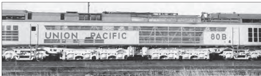
The turbine section of the locomotive was built on a former Great Northern electric locomotive chassis. Union Pacific
