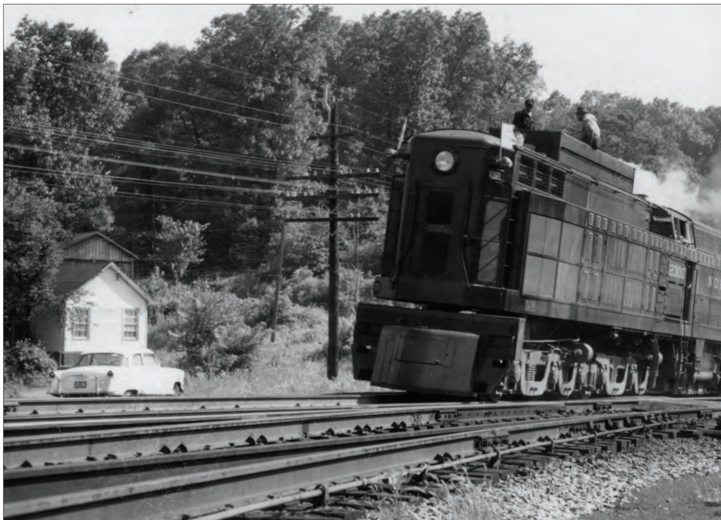
Jawn Henry pulls a test train at Riverside, Va. The men on the top of the locomotive are standing in the coal bunker shoveling coal onto a scale during an efficiency test in 1954. Norfolk & Western Historical Society
