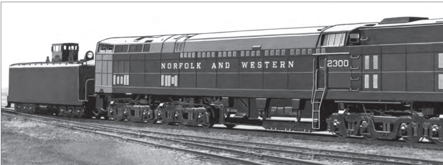
Norfolk & Western's TE-1 is shown in a publicity photo. The coal bin and the dynamic braking grids are in front of the cab. Behind it are the high-pressure boiler, steam turbine, electrical generators. Norfolk & Western Historical Society
