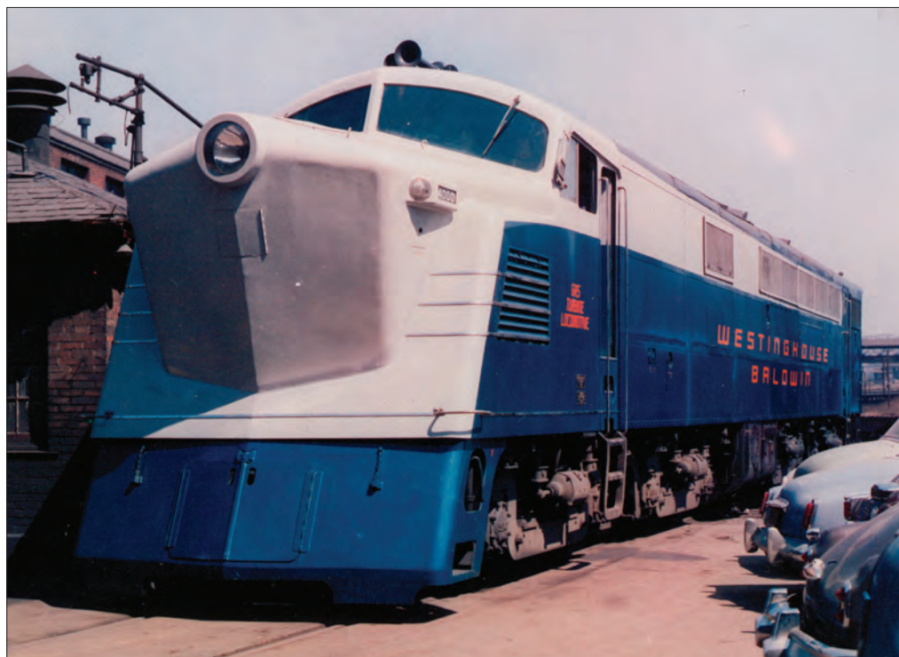
The B-B+B-B gas-turbine-electric passenger locomotive, dubbed the "Blue Goose" because of its paint scheme (and perhaps for its unusual appearance), came just as builder Westinghouse was exiting the locomotive business. It was dismantled in 1953. From the collection of Johann Arthur Stamm
