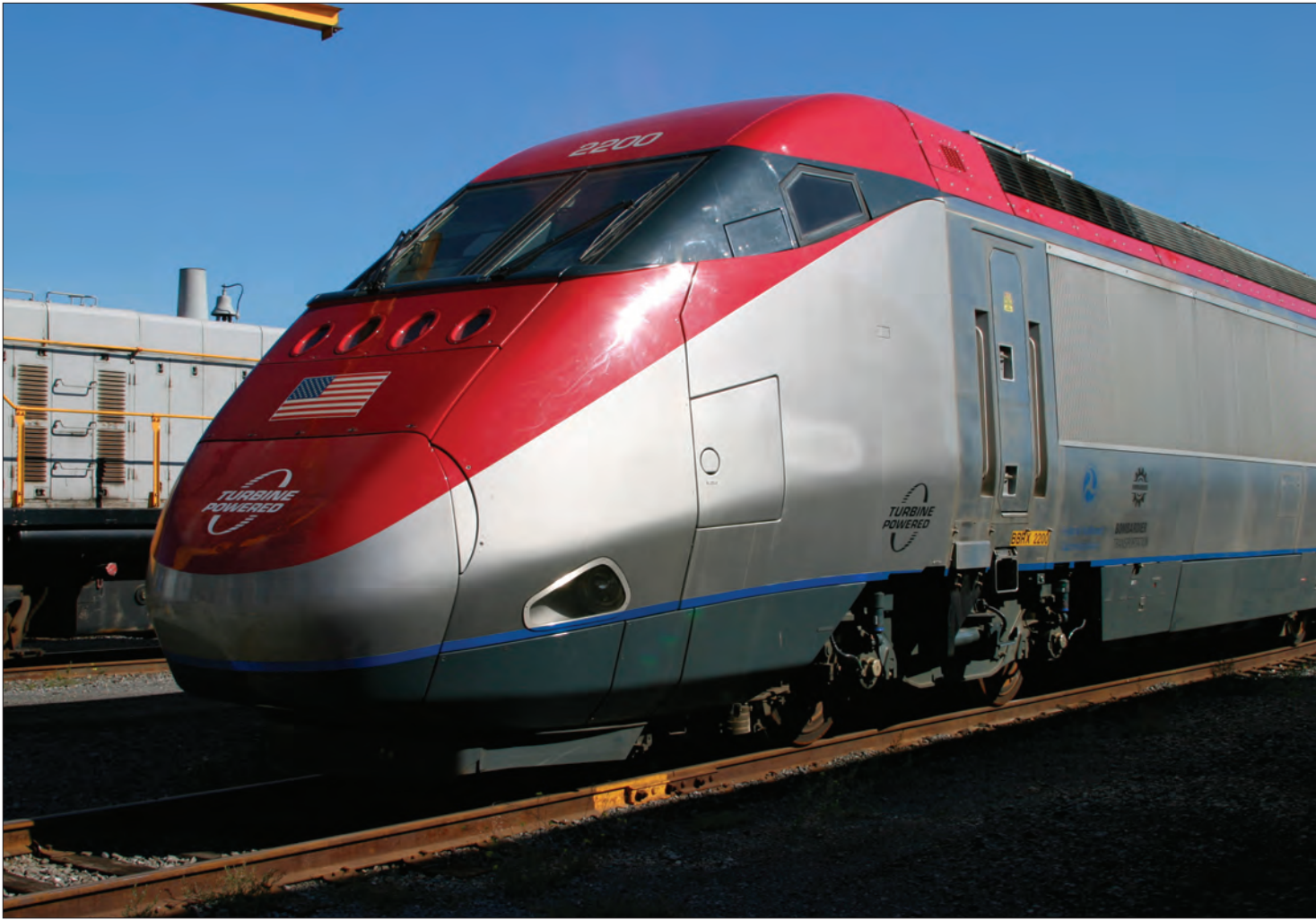
Its appearance modeled after the Amtrak Acela, Bombardier's JetTrain prototype gas turbine locomotive was on display at VIA Rail's Montreal Maintenance Center on Sept. 6, 2003. Michel Robichaud
