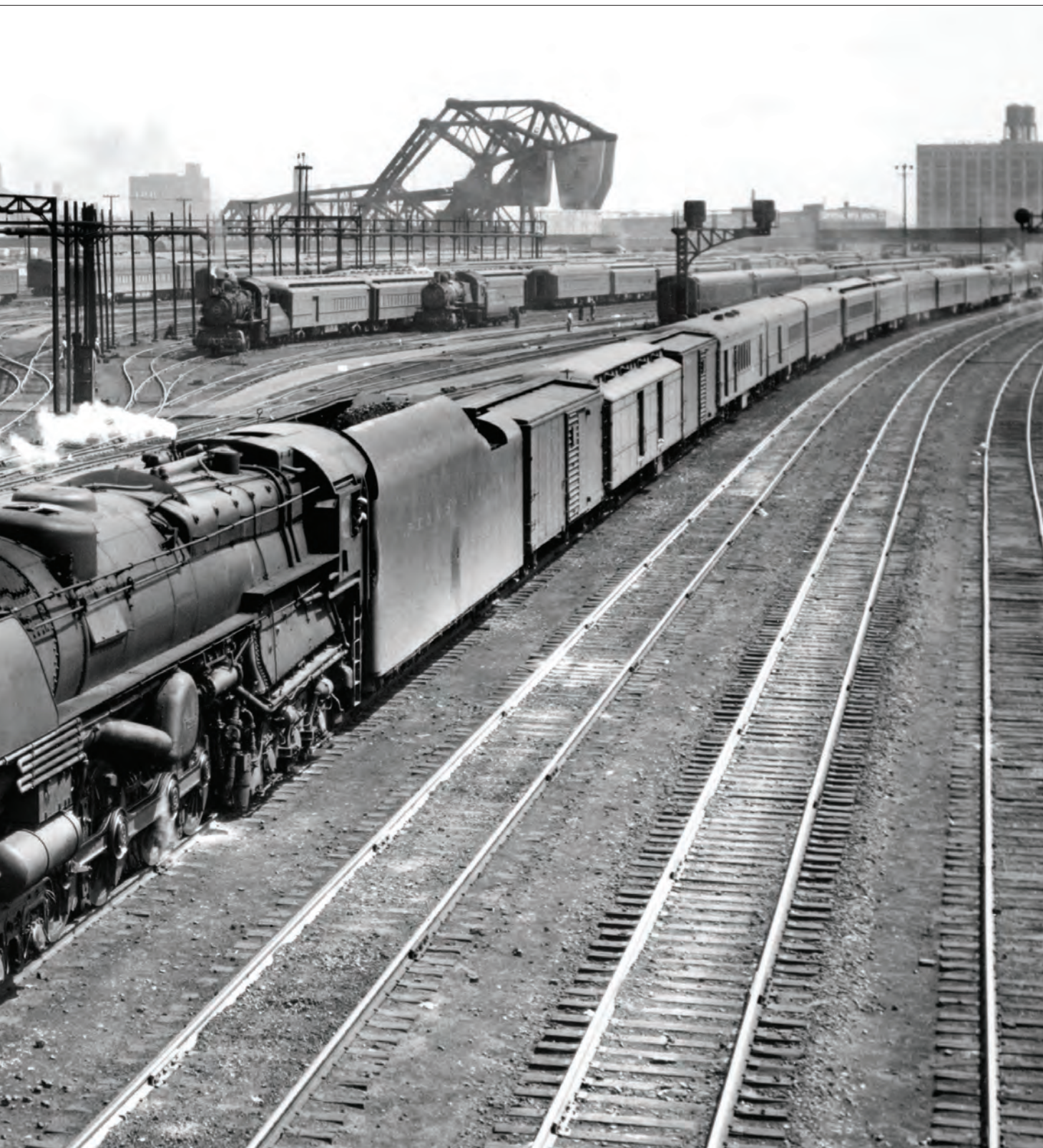
The Manhattan Limited leaves Chicago Union Station with a 14-car train in June 1947. The 1,500 horsepower reversing steam turbine is evident on the left side of the Pennsylvania RR class S2 6-8-6 along with the steam line feeding it from the front of the boiler. PRRT&HS/The Keystone
