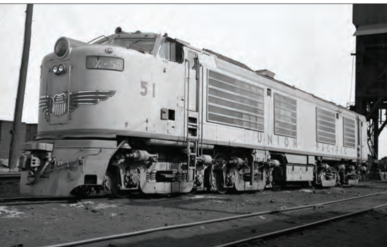
First-generation 4,500 horsepower gas turbine locomotive No. 51 was the first production model. These locomotives initially used heated onboard Bunker C fuel tanks. The 7,200-gallon tanks gave the locomotives an approximate range of 400 miles. They were later equipped with heated fuel tenders. David P. Oroszi collection
