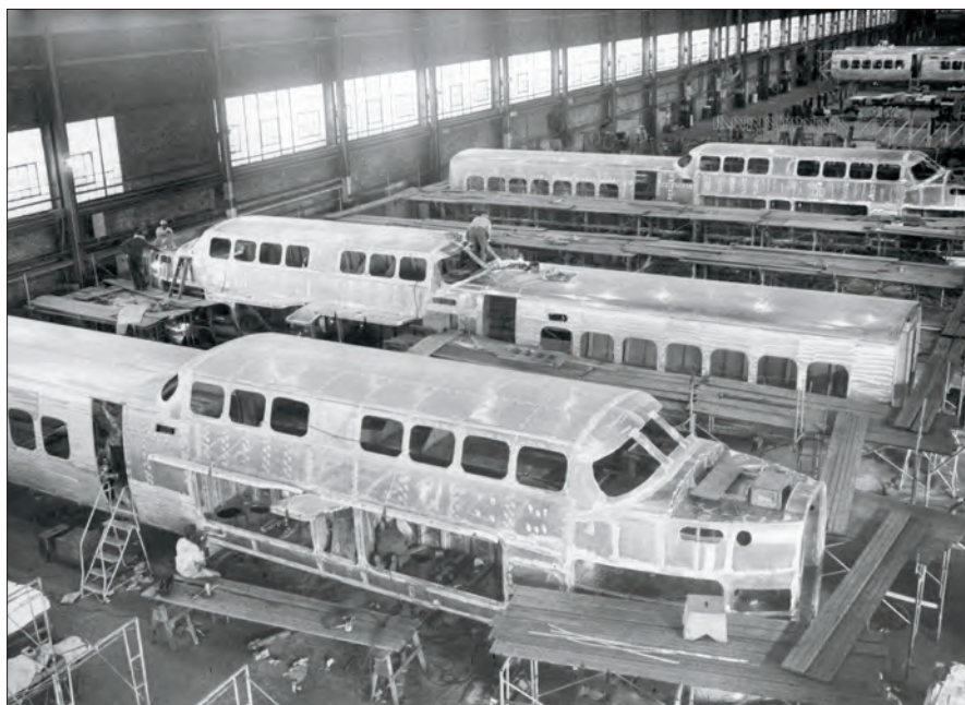
TurboTrain powerdome cars and coaches are under construction at Pullman-Standard's plant in Chicago. To cut weight, these trains were made of aluminum alloys, up to 1 inch thick in places to produce required strength. Pullman-Standard
