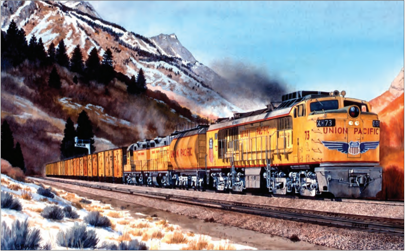
A 4,500 horsepower UP GTEL "Veranda" (Nos. 61-75, so-called because of the external walkways) is depicted in a watercolor climbing over the Wasatch mountain range with a "hot fruit drag" loaded with cabbage, carrots, celery, tomatoes, spinach, and mandarins. The train is 20 miles outside of Ogden, Utah, destined for Chicago and points East. Gil Bennett, collection of Dick Harley
