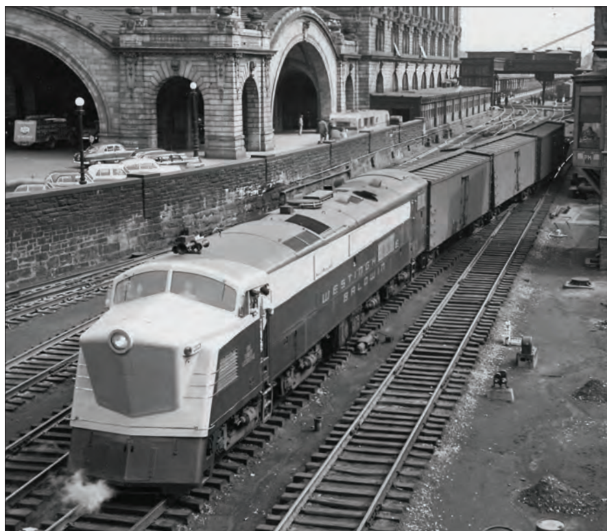
The Blue Goose pulls out of Pittsburgh Union Station with a test train. The 4,000 horsepower locomotive once pulled a 29-car passenger train from Altoona to Pittsburgh, Pa., unassisted. From the collection of Johann Arthur Stamm
