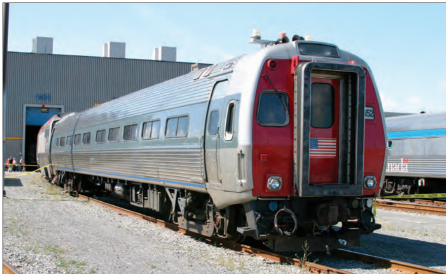
The JetTrain was tested with Amtrak cars and successfully reached 130 mph as a matter of routine. Michel Robichaud
