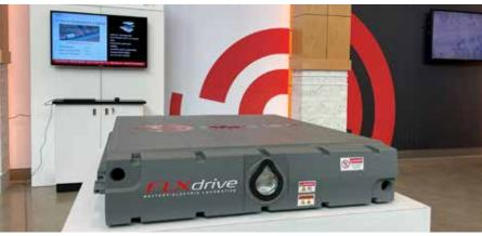
A FLXdrive battery pack. The Roy Hill unit contains 72 battery packs with more than 36,000 cells, giving the unit 7 megawatt-hours of power.
