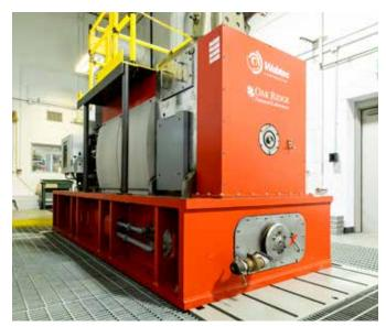
A single-cylinder, hydrogen-fueled engine is undergoing testing at the U.S. Department of Energy's Oak Ridge National Laboratory.
