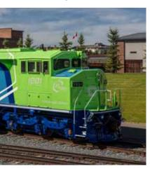
Units converted to hydrogen fuel could look much like the LNGpowered locomotive-and-tender sets now in use the Florida East Coast. Travis Mackey
