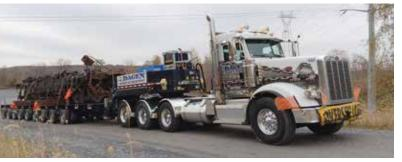
Weighing 87 tons, the S1 undercarriage, the heaviest piece to be moved, required a special trailer and was moved as a "super load."
