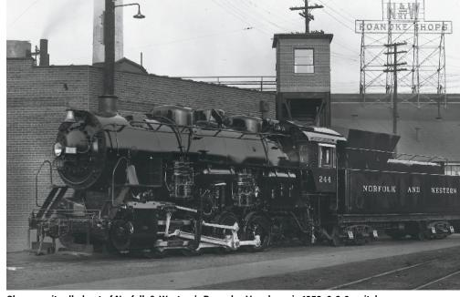
Shown as it rolled out of Norfolk & Western's Roanoke, Va., shops in 1953, 0-8-0 switcher No. 244 concluded a group of 30 such locomotives built by the railroad, and was the last steam locomotive constructed in the U.S. for a major American railroad. Norfolk & Western
