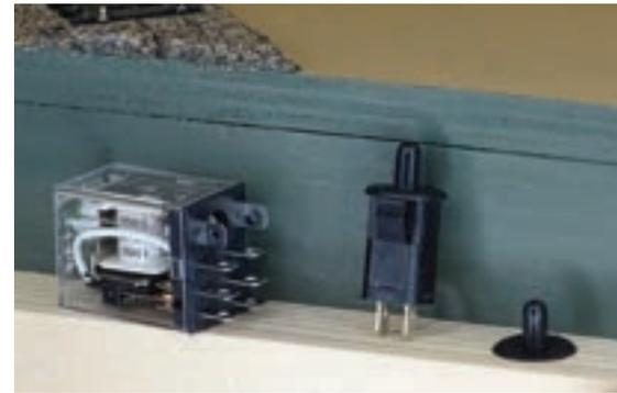
**2** Dave used Forstner bits to countersink the normally open plunger switch into the lift bridge's stop block. When the bridge is down, the switch is closed, changing the polarity of the power to the Tortoise and retracting the wire.
