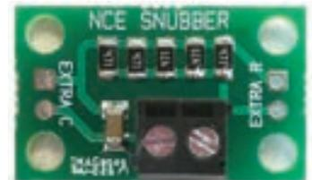
5 This NCE snubber is sold in two-packs. They are attached to the ends of the track bus.
