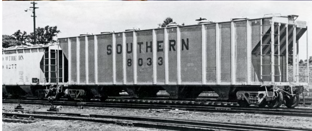
New freight car designs: tri-level auto-rack (carrying '66 Mustangs), 86-foot hi-cube boxcar for auto parts, and "Big John" covered hopper. Top two, Jim Hediger; above, Southern
