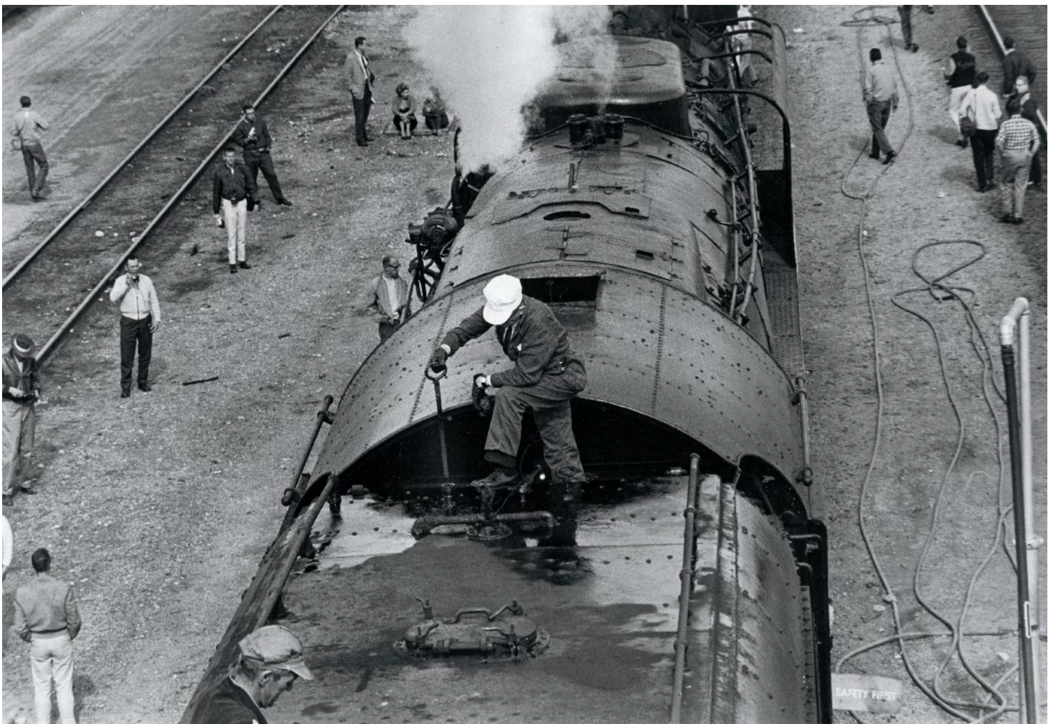
At Laramie, Wyo., a crewman checks the reserves of a tender that holds 6,550 gallons of fuel. John Gruber
