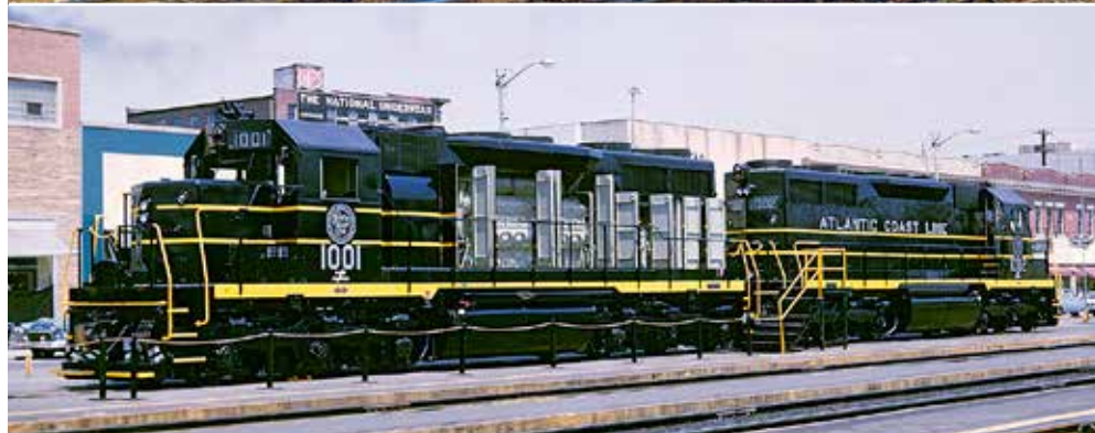
Both roads bought EMD's six-motor, 2,500 h.p. road-switcher. Top, a dual-service SDP35 leaves Birmingham with Seaboard train 6 in 1966. Above, Coast Line shows off two of its SD35 freight units at Rocky Mount, N.C., in 1964. SAL: J. David Ingles; ACL: Wiley M. Bryan
