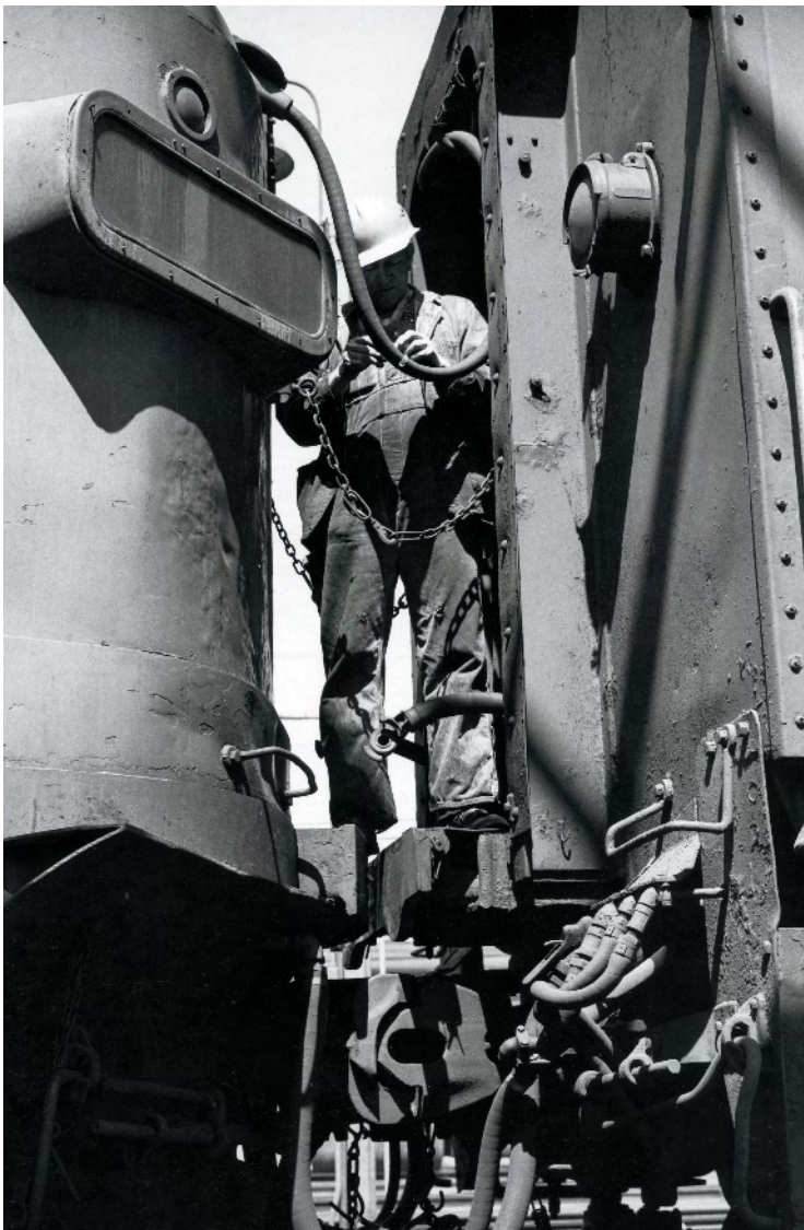
12 Electrician Ed Robinette renews an m.u. jumper cable between units, affixing its new date tag.
