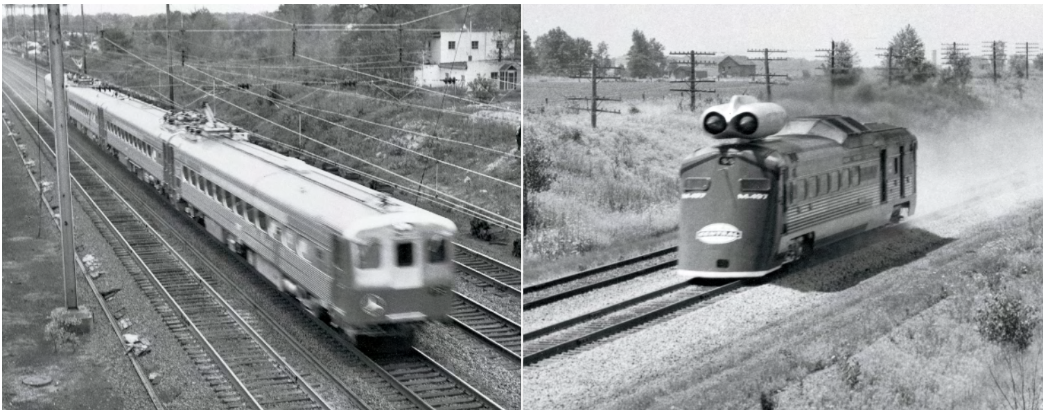
High-speed tests made headlines in 1966-67. Left, U.S. DOT electric M.U.'s attained 156 mph on PRR in New Jersey on May 24, 1967. Right, NYC M-497, an RDC3 fitted with jet engines, hit 183.9 mph west of Stryker, Ohio, on July 23, 1966. PRR: Don Wood; NYC: Tom Miller
