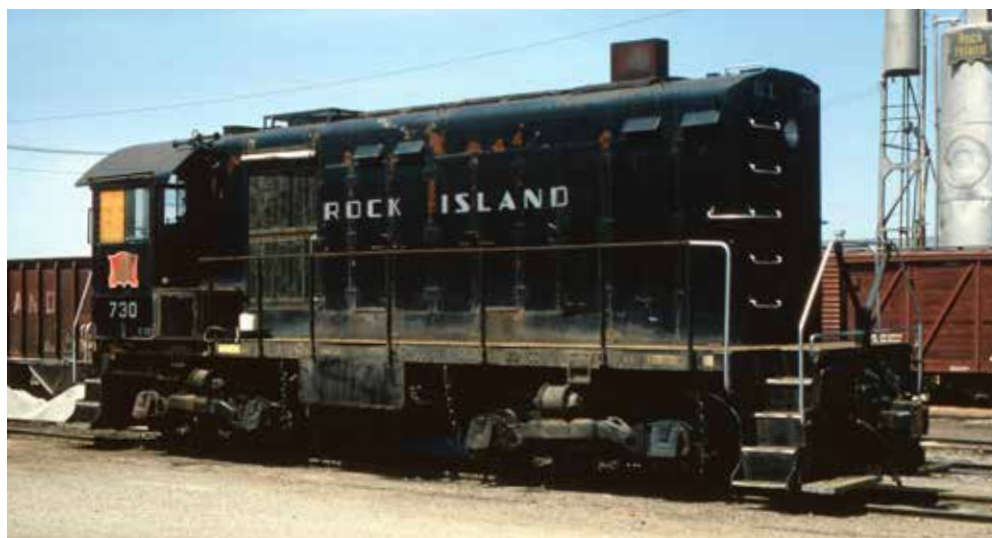
Rock's only high-hood Alco, ready for trade-in at Kansas City, Kans., on April 16, 1965, is thought to have been built in 1937, two years before the railroad bought it. J. David Ingles
