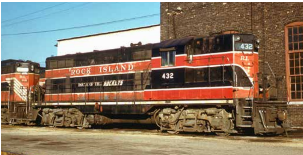
Rock's first 12 GP7's, in 1950, wore this simple red and black, as did the BL2's. Beginning in '51, RI Geeps had the fancy "barber pole" version, as on the unit at left. Monty Powell
