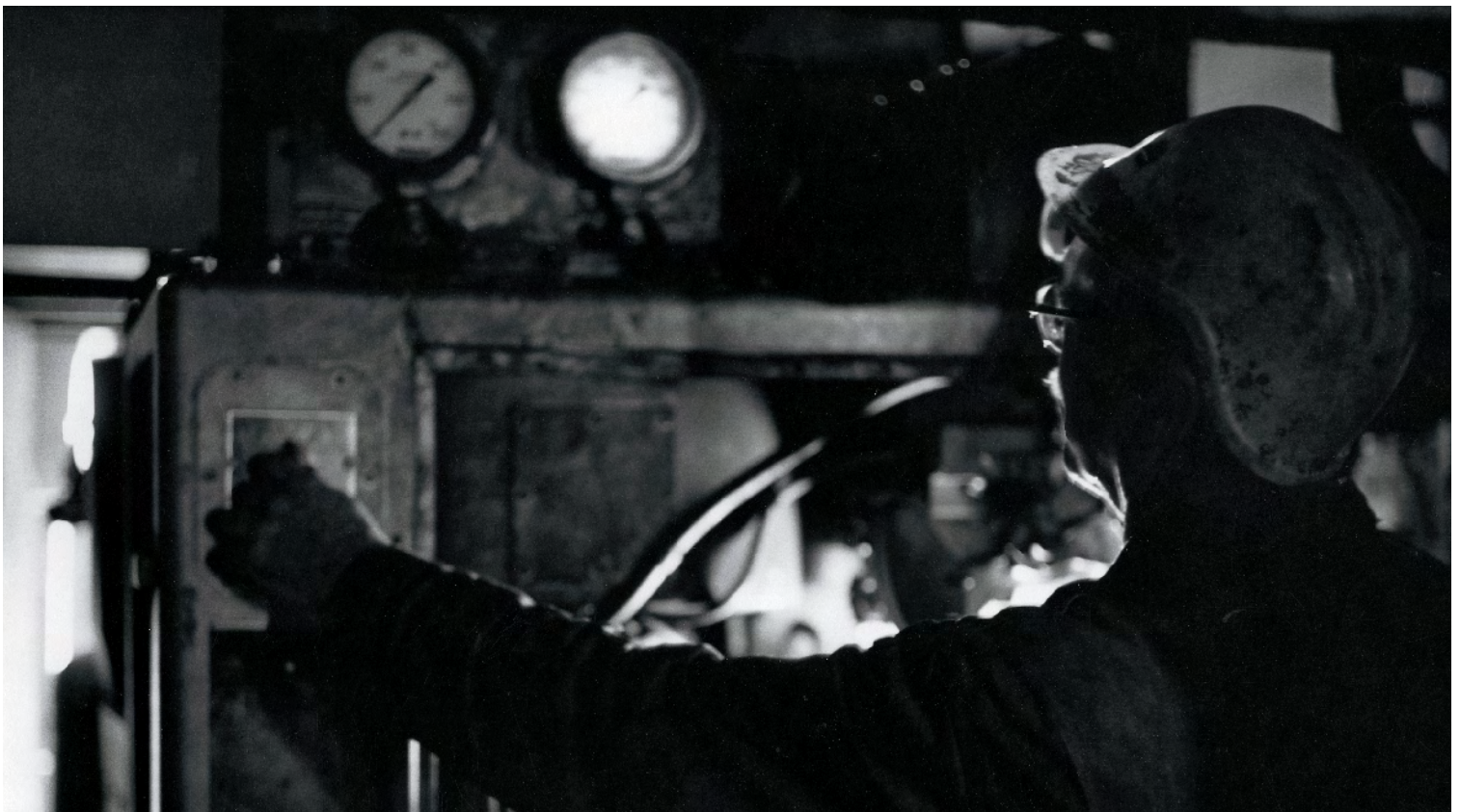
11 In the darkness of a locomotive's interior, a boiler-machinist checks the performance of a steam generator for train heating. SP's fleet of 66 PA/PB's, which included the 2 inherited from Cotton Belt, dated from 1948–53. Santa Fe's fleet of 44 ranked second.
