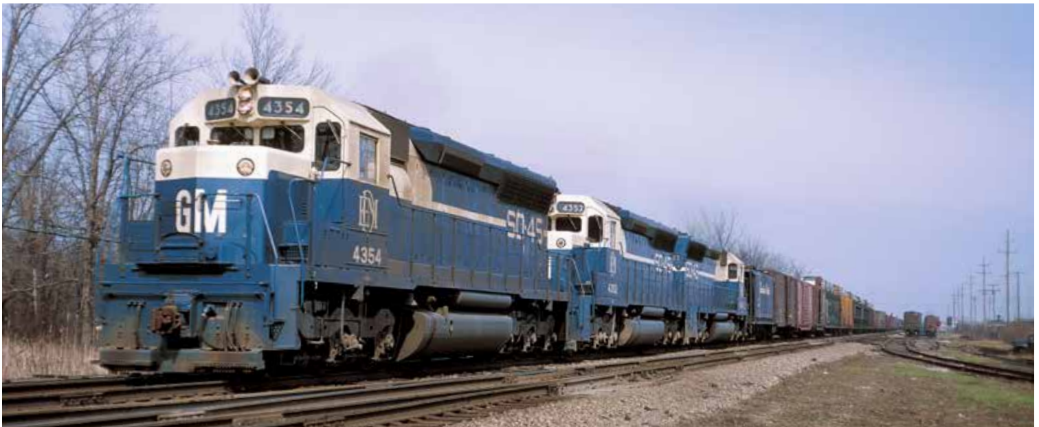
Surprise of the season: EMD's unprecedented 3,600 h.p., 20-cylinder SD45 was a big seller from its introduction in 1966. Demonstrators 4352–4354 roll a Norfolk & Western freight west out of Detroit through Romulus, Mich., on the old Wabash in April '67. J. David Ingles
