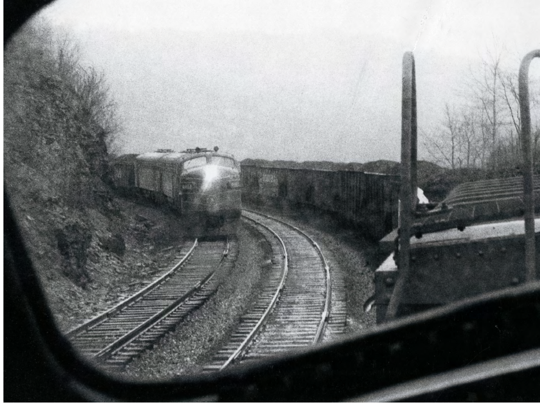
Partway up Cranberry, helper 4493 has stopped to cool its traction motors as yet another set of F7's swings past with empties headed back to the mines. Frank E. Shaffer
