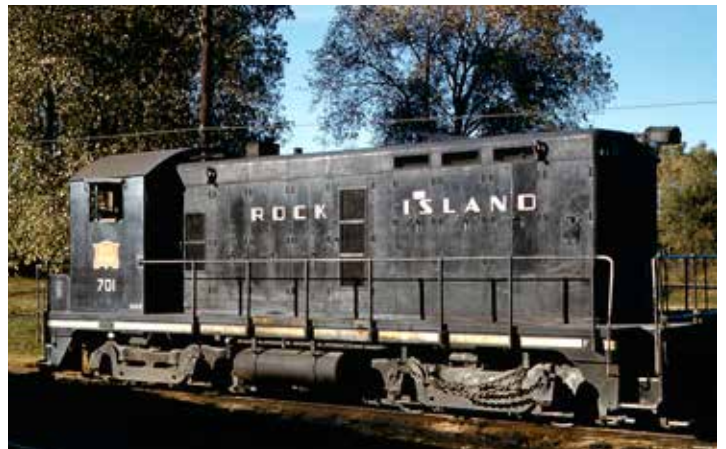
Clockwise from top left: Rock's only FM's, Nos. 400–401, were repowered at age 10 in 1958 by EMD. No. 401 is at Chicago's 47th Street "Rocket House" diesel shop on June 15, 1955, and is in a suburban-train race with an RS3 out of La Salle Street August 1, 1963. Rock repowered five of its eight EMC NW1's with Alco 244's during 1956–62. No. 701, at Silvis in fall 1958, shows the unique result. No. 703, at Peoria, Ill., in fall '58, was not done. Clockwise from 401: Monty Powell, Tom Smart, Max Zimmerlein, Monty Powell
