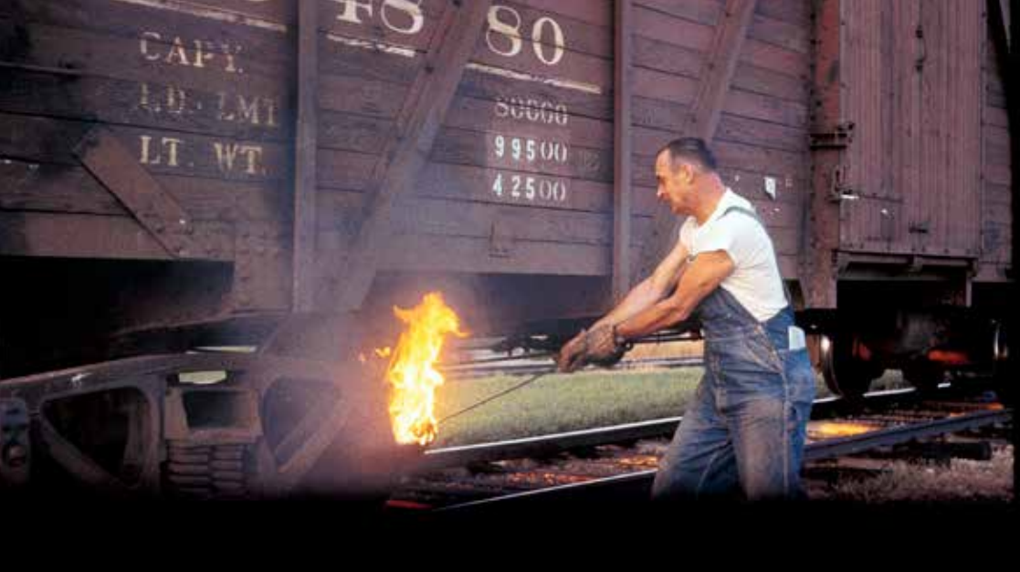
On Soo 76 east of Fredonia, an old railroading lesson is relearned: When non-roller-bearing cars sit for a time, make sure there's enough oil in the journal boxes.
