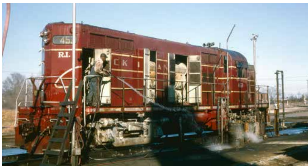
EMD prime mover is visible in RS2 453 at Little Rock on the last day of 1962. J. David Ingles
