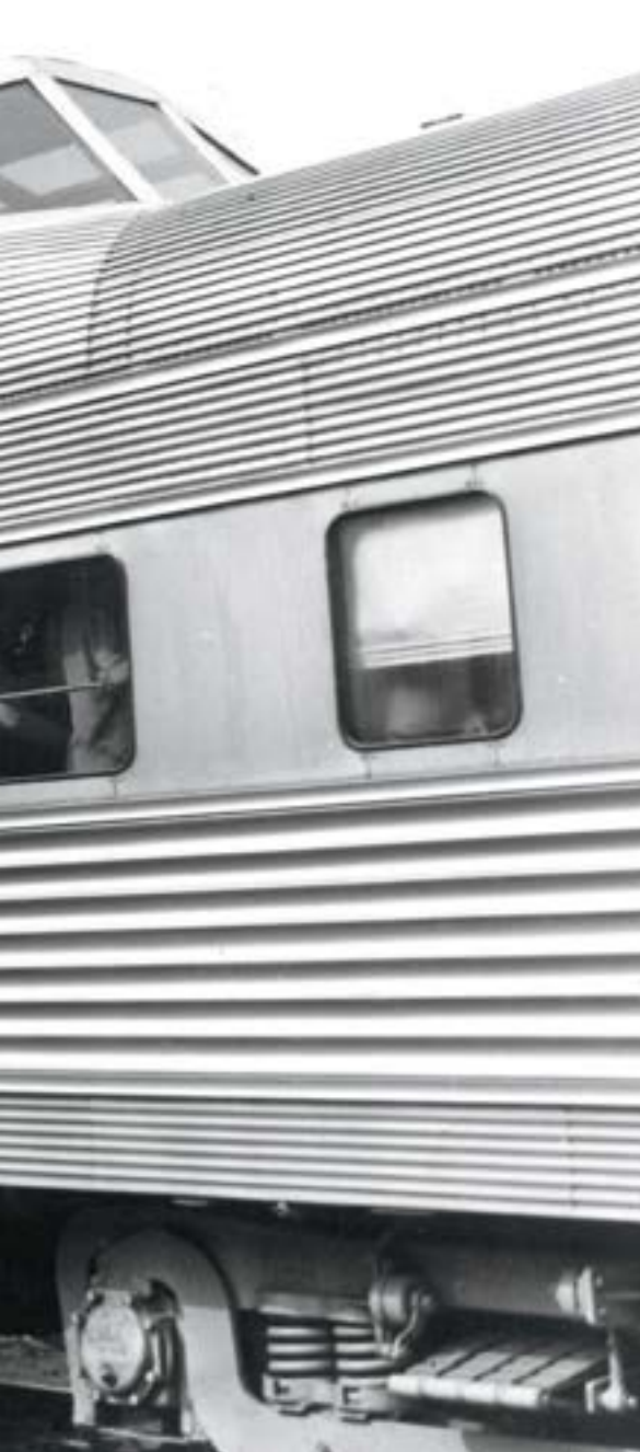
All four of the Train of Tomorrow's cars had domes. Material shortages precluded use of the planned curved glass, so Pullman-Standard settled for flat panes, a style P-S stuck with in its subsequent domes. This view is in the chair car Star Dust . General Motors
