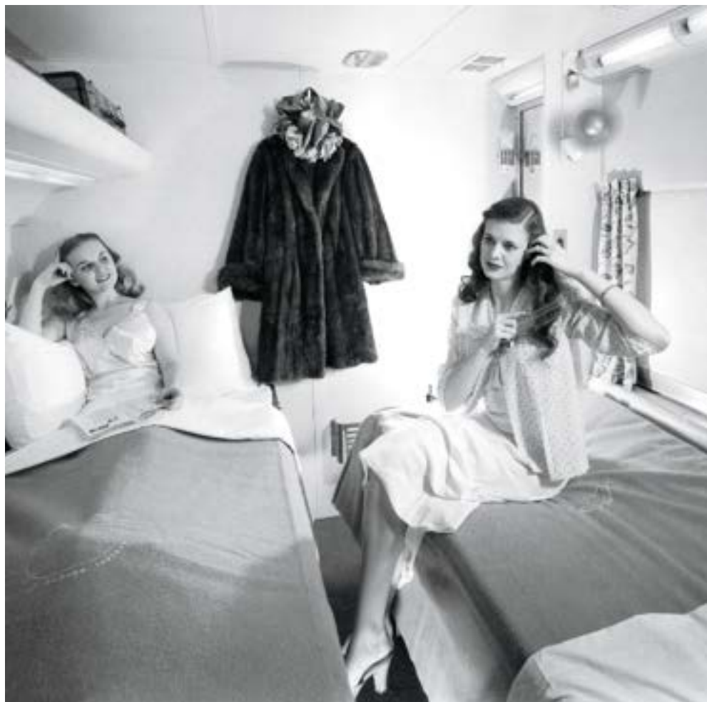
Dream Cloud's compartments featured two lower berths instead of the more usual upper and lower. The berth at left converted from a sofa, while the one by the window folded down from the wall. Note the blankets with Train of Tomorrow markings. General Motors
