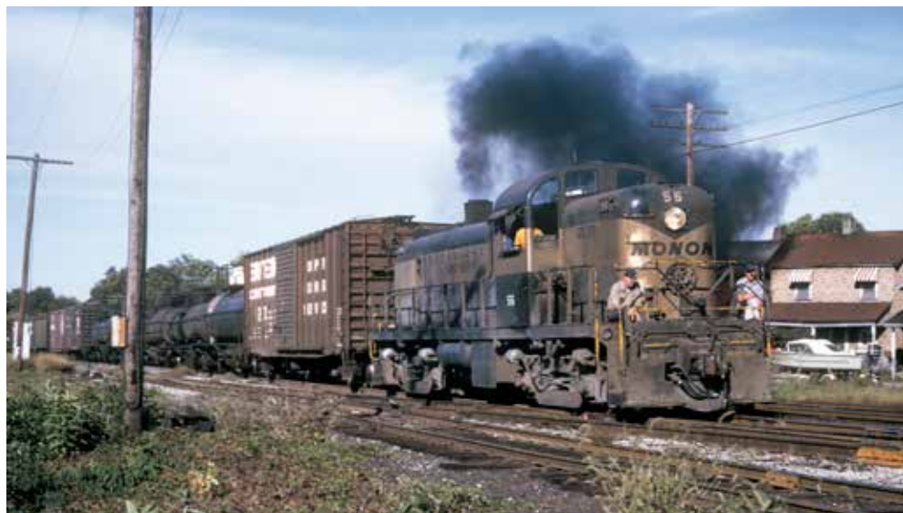
Having pioneered the road-switcher type of diesel in 1941 with the 1,000 h.p. RS1, Alco released the 1,500 h.p. RS2 in 1946, the same year Baldwin rolled out its first road-switcher. In 1969, 22-year-old Monon RS2 No. 56 works at Lafayette, Ind. Eric Hirsimaki
