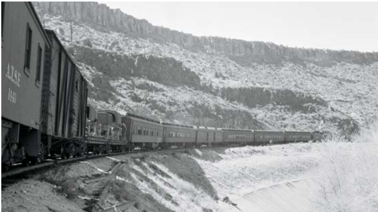
A California-bound troop train has halted near Peach Springs, Ariz., about 5½ miles beyond Nelson. Between 4-6-2 No. 1329 and the caboose are three sleepers, a baggage car serving as kitchen, two more sleepers, and two flatcars and a boxcar for equipment.
