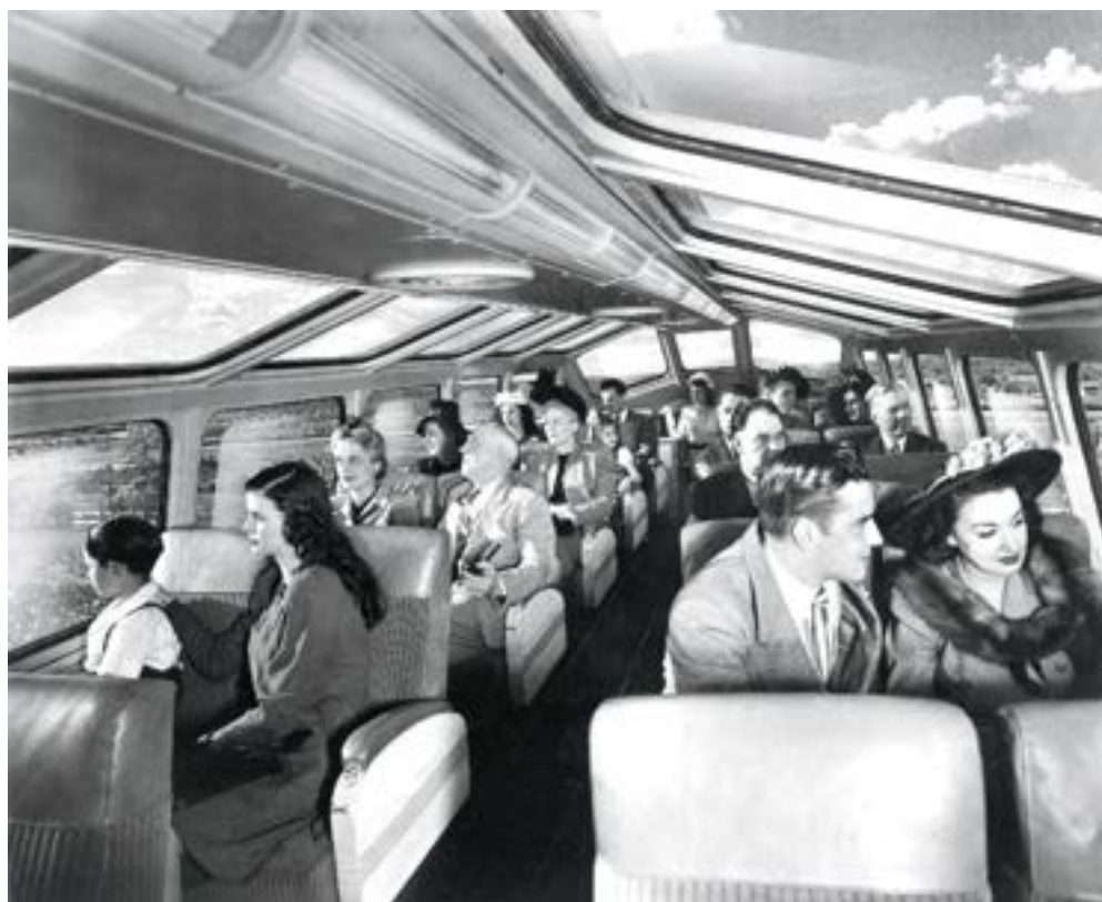
All four of the Train of Tomorrow's cars had domes. Material shortages precluded use of the planned curved glass, so Pullman-Standard settled for flat panes, a style P-S stuck with in its subsequent domes. This view is in the chair car Star Dust . General Motors
