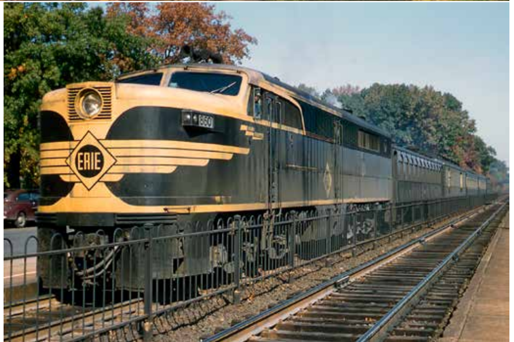
Alco's mid-1940s freight unit was the 1,500 h.p. diesel later known as FA (cab) and FB (booster), three of which (top) work on the MoPac near the state capitol at Jefferson City, Mo., in 1956. Erie 860, at Ridgewood, N.J., in '56, represents Alco's 2,000 h.p. passenger diesel, later called PA and PB. FA, Mac Seabee, Krambles-Peterson Archive; PA, Bob Krone
