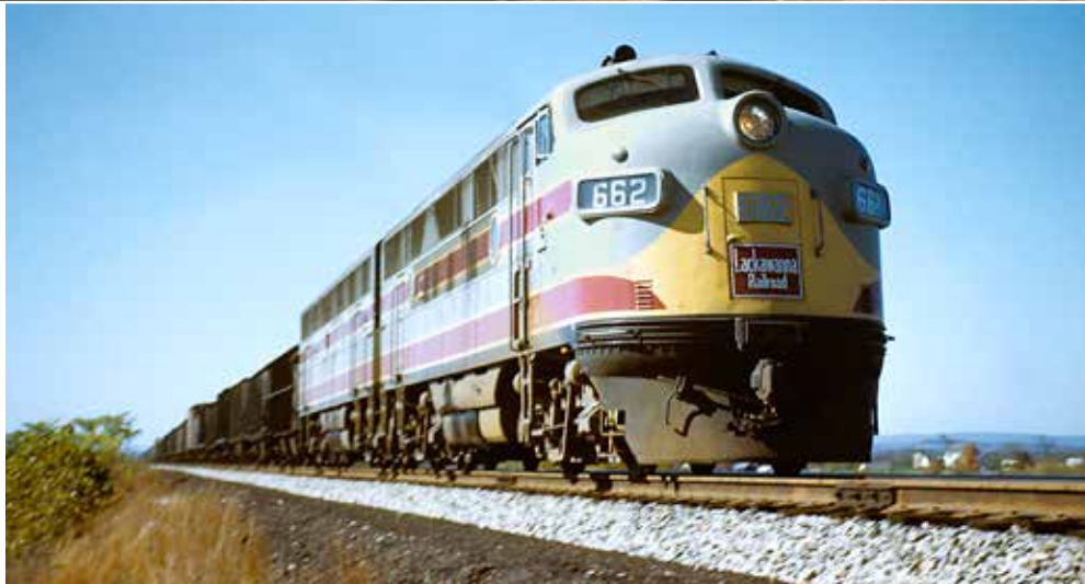
EMD swamped all other builders in postwar diesel sales. Its E7, represented by Alton Railroad No. 100 (top, trailed by an ex-B&O prewar EA on the Abraham Lincoln at Joliet, Ill.), was the best-selling passenger diesel of all time. DL&W 662 and its B unit mate were among 1,807 F3s sold, mostly for freight. E7, B. L. Stone, Krambles-Peterson Arch.; F3, John R. Canfield
