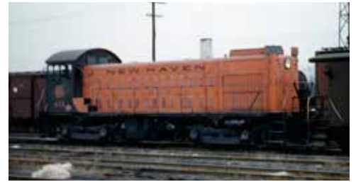
Lima Locomotive Works shed its commitment to steam by merging with Hamilton Engine in 1947. Lima-Hamilton built 174 units, all switchers, road-switchers, and transfer units, including 1,200 h.p. New Haven 633, during 1949-51. Ed Theisinger
