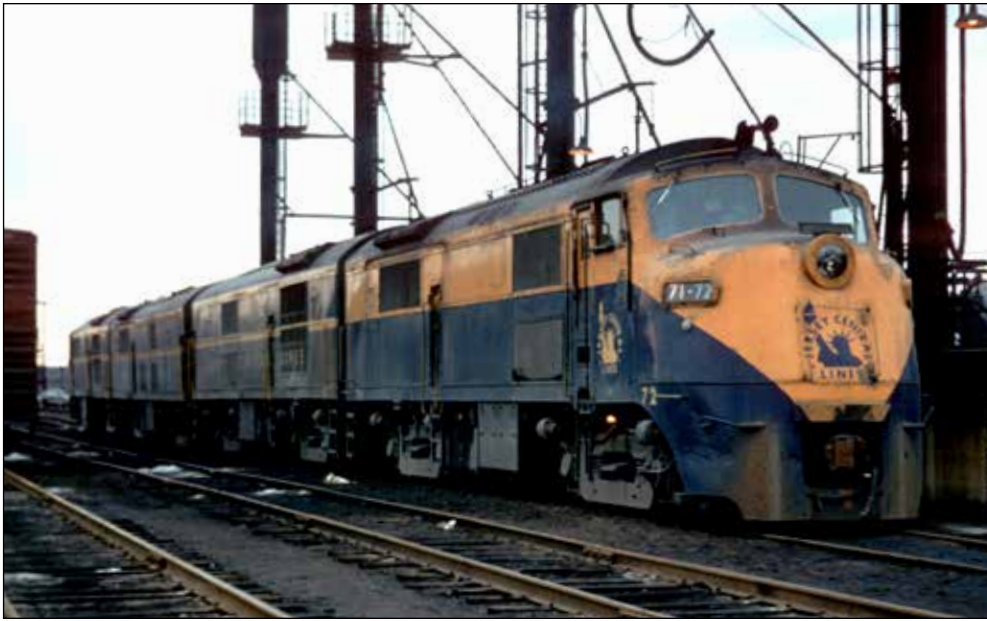
Baldwin Locomotive Works, founded in 1831, dabbled in diesels in the 1920s and '30s, but didn't field a successful road unit until its 20-axle "Centipedes" of 1945. Its 1,500 h.p. "Babyface" freight diesels, like this Jersey Central foursome, debuted in 1947. Paul Lerman
