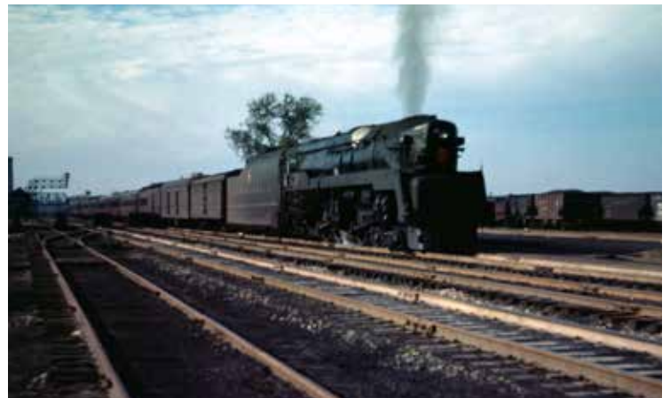
No. 5526, one of the Pennsylvania's 52 sleek T1 4-4-4-4 duplex drives of 1942-46, is in charge of a midday eastbound train at Englewood in the late 1940s. Barney L. Stone, Krambles-Peterson Archive
