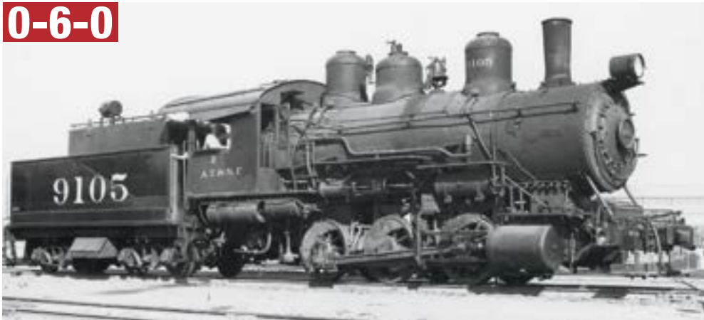
Six-wheel switcher 9105, built by the Santa Fe in 1904 as No. 2105, rests at Richmond, Calif., in 1946. Imagine a 128-mile L.A.–San Diego trip on this 51-inch-drivered engine!
