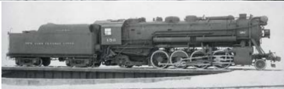
Capacity tests of 1919 on the P&LE with an H-9 2-8-2 (like No. 9593, top) helped determine optimum cut-off settings and led to cut-off/speed cards for engineers. A few years later, tests with H-10 156 (above) established the importance of constant back pressure.
