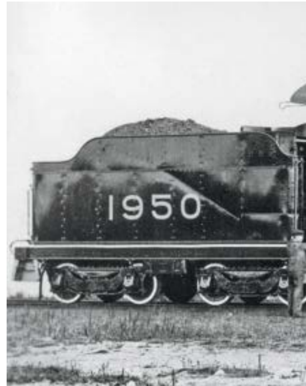
Prototype 1950 wears flat gray and white striping for its builder's portrait. The boxy "reheater," unique to this engine, gave way to a more conventional superheater.
