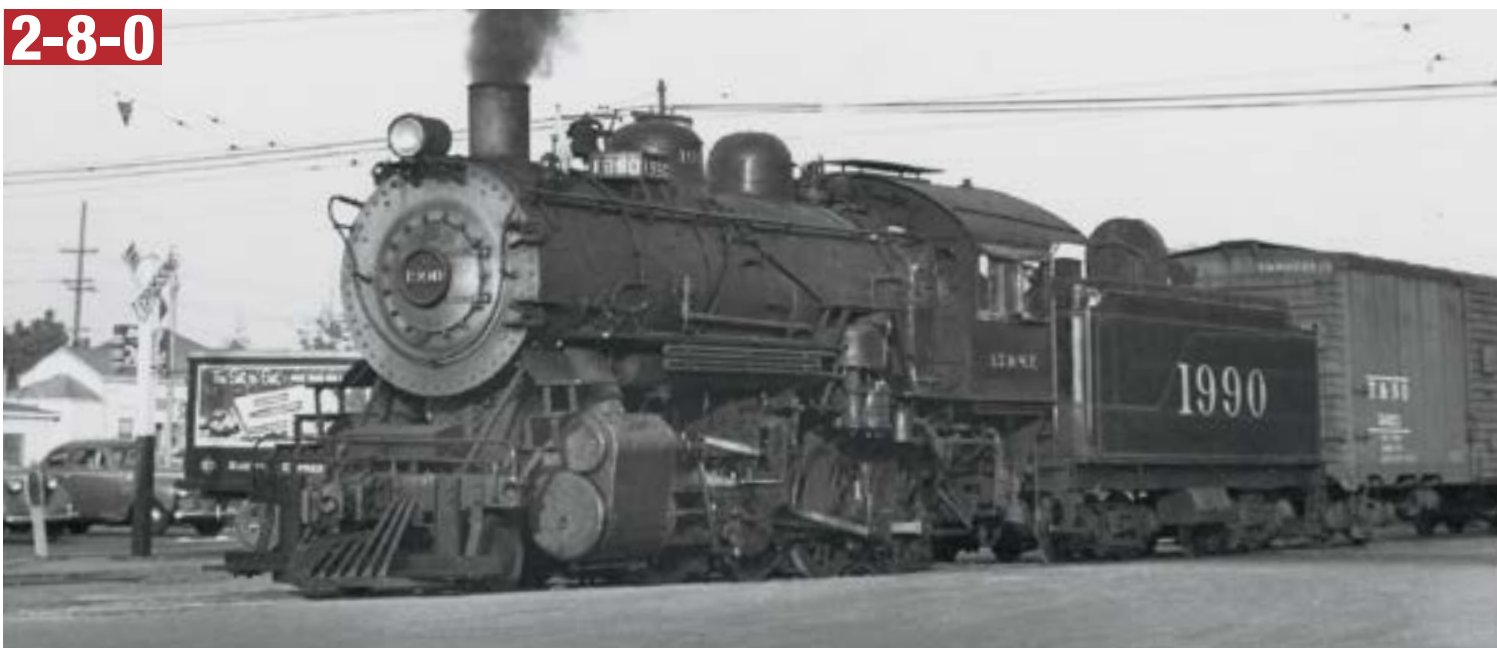
Consolidation 1990 was a heavy road freight engine when built by Baldwin in 1907; 40 years later it works a local freight in Oakland.
