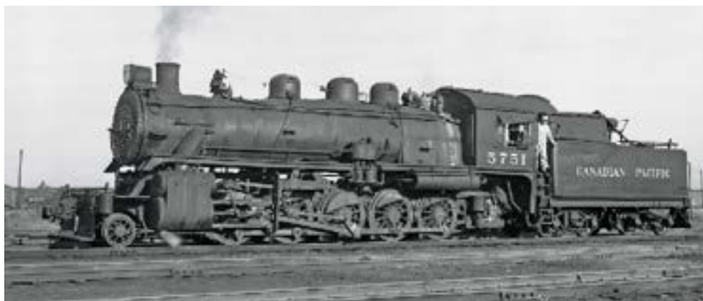
After less than a decade, CP rebuilt the class R1 0-6-6-0s to R2 2-10-0s; as Decapods, they led long lives. R2a 5751, originally R1a 1951, rests in Montreal on July 27, 1956.
