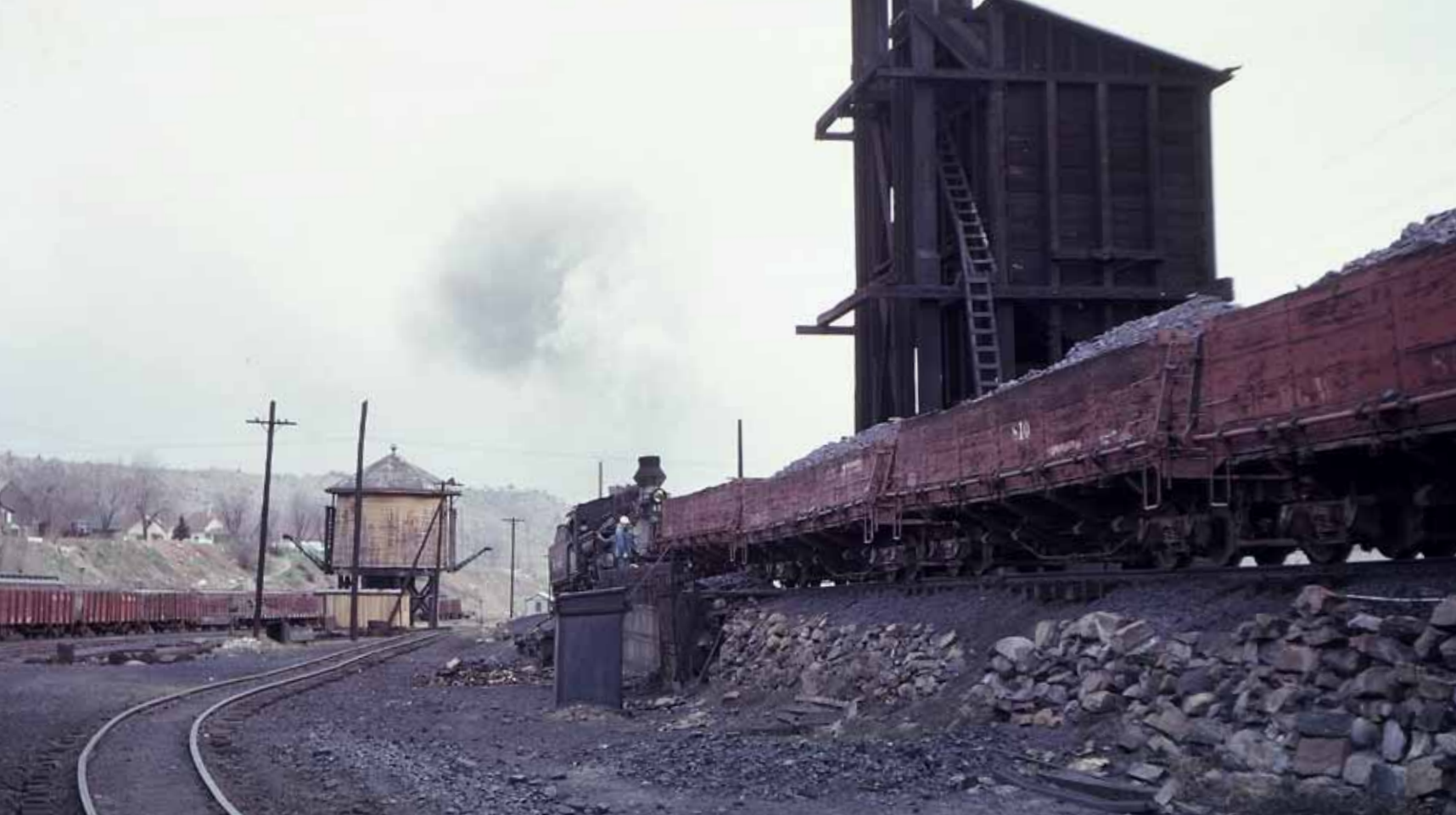
Leaving Chama and stopping in Durango on my way back to southern California in September 1963, I encountered class K-28 No. 478 (one of D&RGW's 10 K-28's, all built by Alco in 1923) positioning a cut of drop-bottom gondolas at the coaling tower. The cars were dumped and the coal then hoisted by a bucket device into the tower. Two crewmen just in front of the locomotive guide the engineer.
