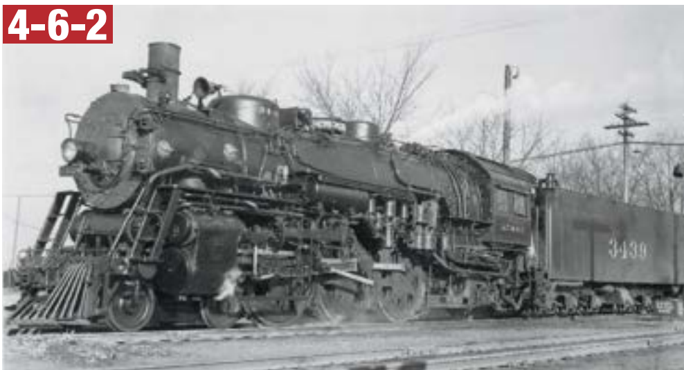
Santa Fe's newest 4-6-2s were 50 rather ordinary 3400-class engines of 1919–24, which were rebuilt for high performance in the 1930s and '40s. No. 3439 digs in at Chillicothe, Ill.
