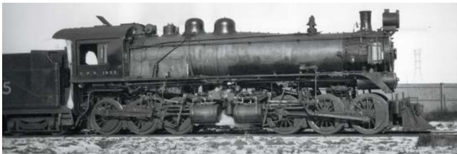
As a simple articulated, R1c 1955 had cylinders of equal diameter, although they were positioned face-to-face as on the five Mallets.
