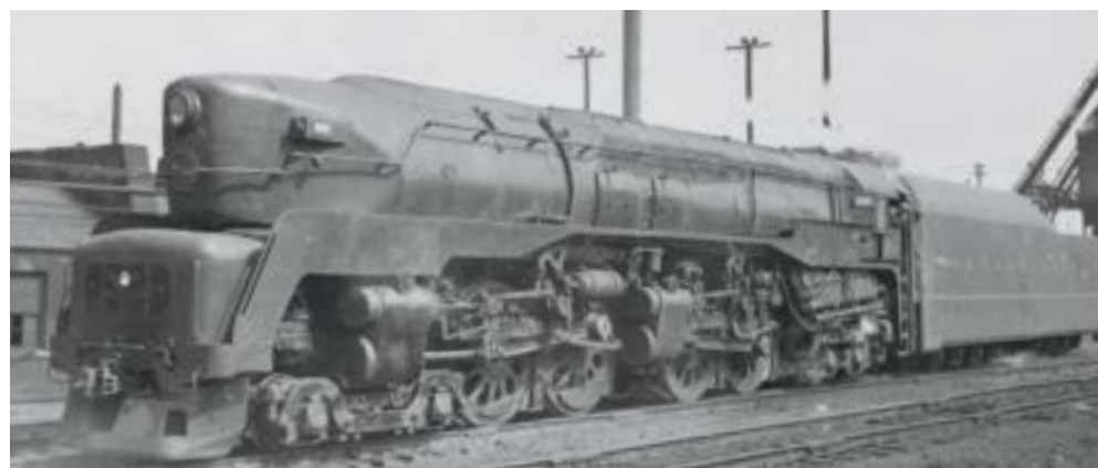
Even as diesels were coming on strong, PRR tinkered with the T1's. No. 5500 (top, at Cincinnati with two K4's) was re-equipped with Franklin rotary cam valve gear, while 5547 (at Pittsburgh in '48) got Walschaerts, prompting a change in classification to T1a.
