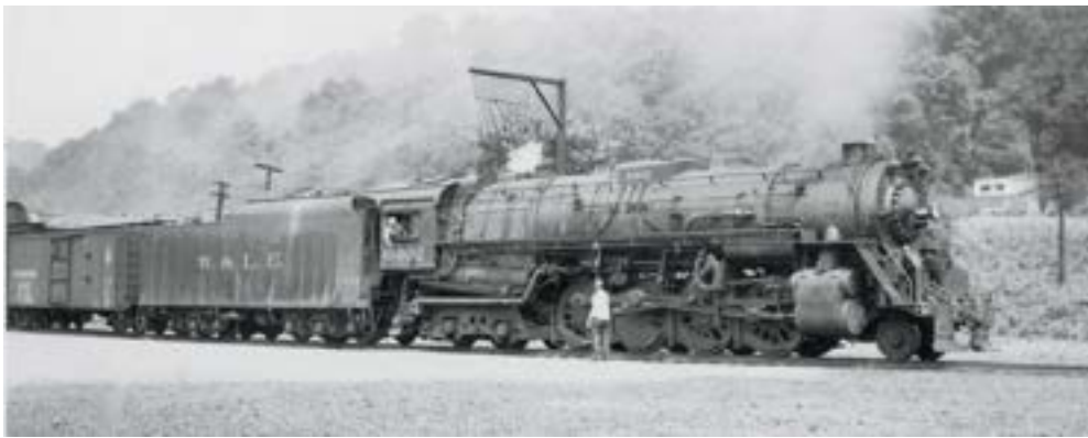
Wheeling & Lake Erie 2-8-4 6402 on train 96 gets orders at Warrenton, Ohio, in July 1949. The K-1's Valve Pilot cam box is just above operator Johnnie Dietrich's right shoulder.
