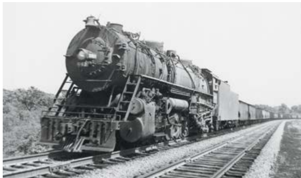
Bessemer & Lake Erie 2-10-4 643, the only Valve Pilot engine to steam in the preservation era, nears Albion Yard, Pa., with ore from the Conneaut, Ohio, docks in the 1940s.
