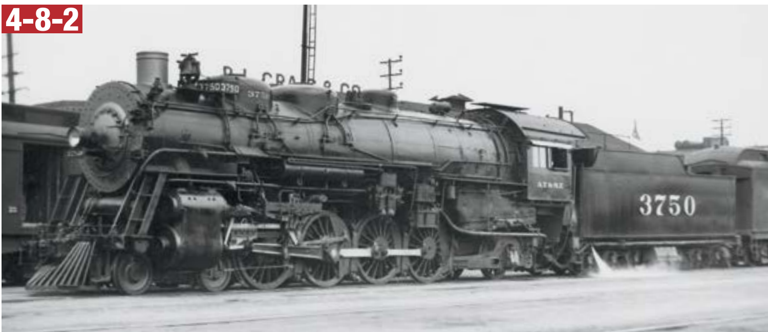
Engine 3750 was the last of Santa Fe's 51 Mountain types, built during 1918–24. Their 69-inch drivers precluded high-speed running.
