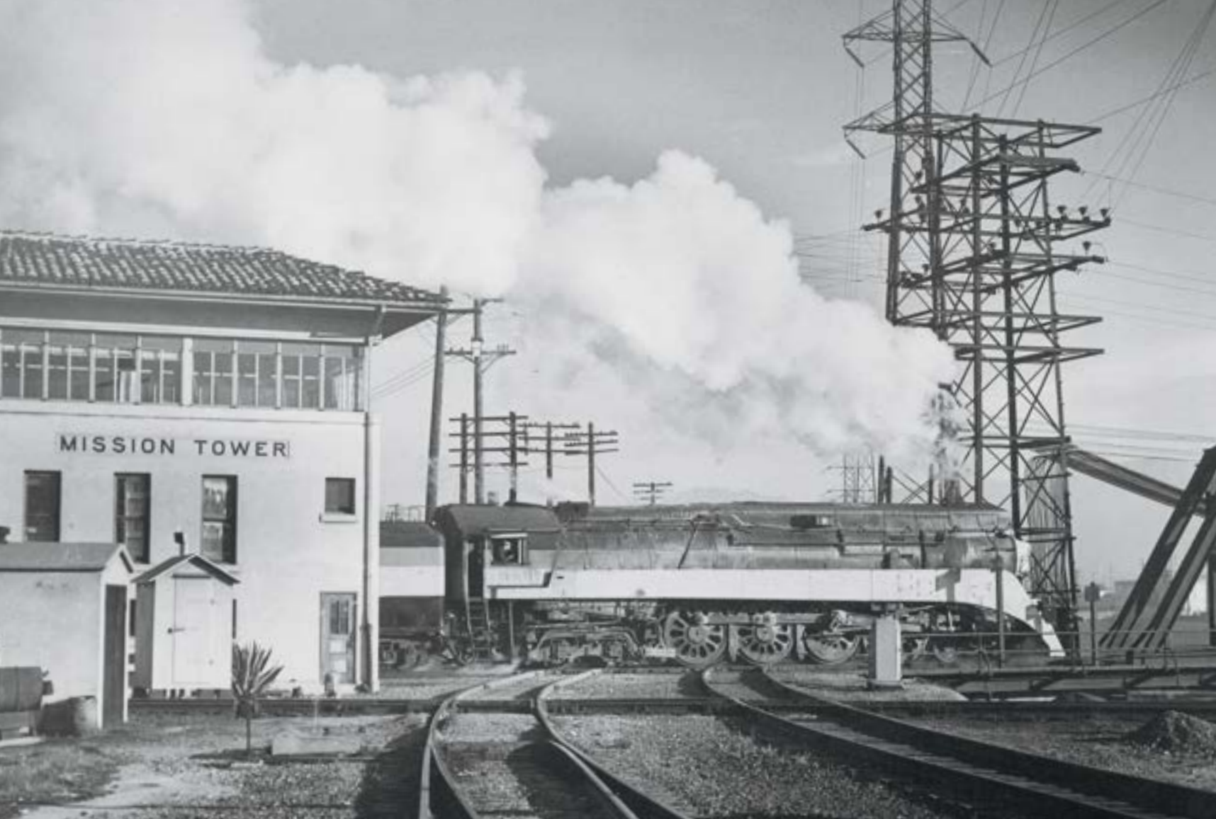
Running-board skirting hides the cam box on GS-4 4454, departing Los Angeles with SP's Coast Daylight . Many GS's had their Valve Pilots removed before retirement.
