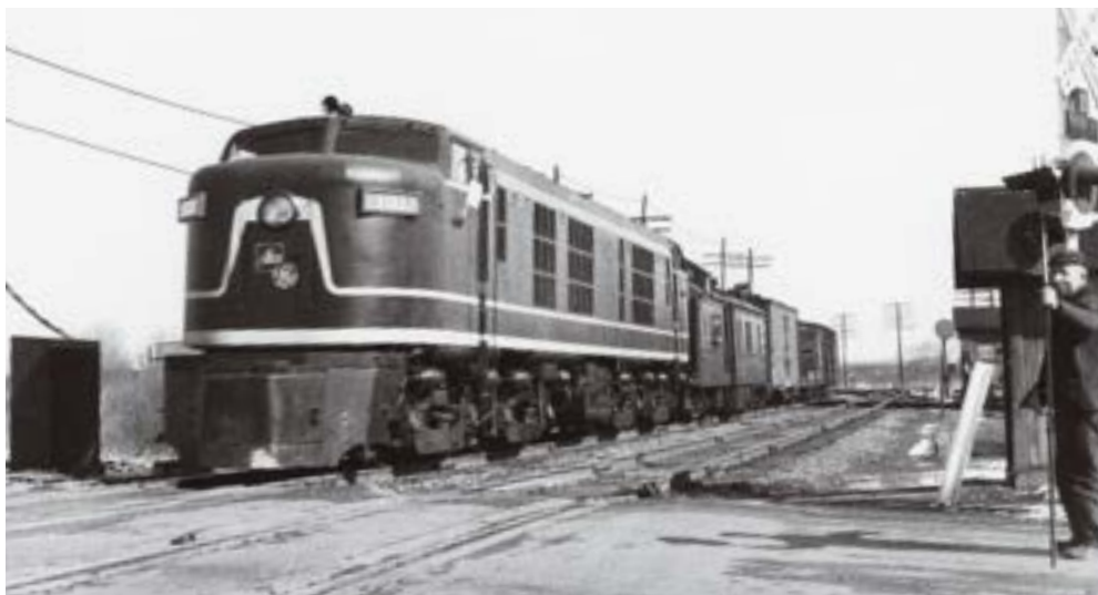
Experimental Alco-GE gas turbine No. 101 hauls a dynamometer car and a freight at Blasdell, N.Y., during a test run on the Nickel Plate. UP’s order for 10 similar units underscored the gas turbine’s role as the diesel’s biggest challenger in 1950. Franklin E. Gnau
