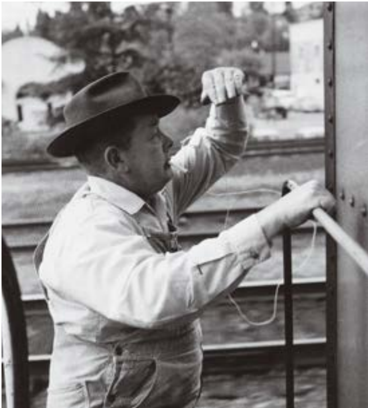
With practiced ease, flagman Selanders snags “19” orders as the train passes Colfax. The orders tell the extra not to pass Midas, 19 miles ahead, before train 28, the eastbound Overland .
