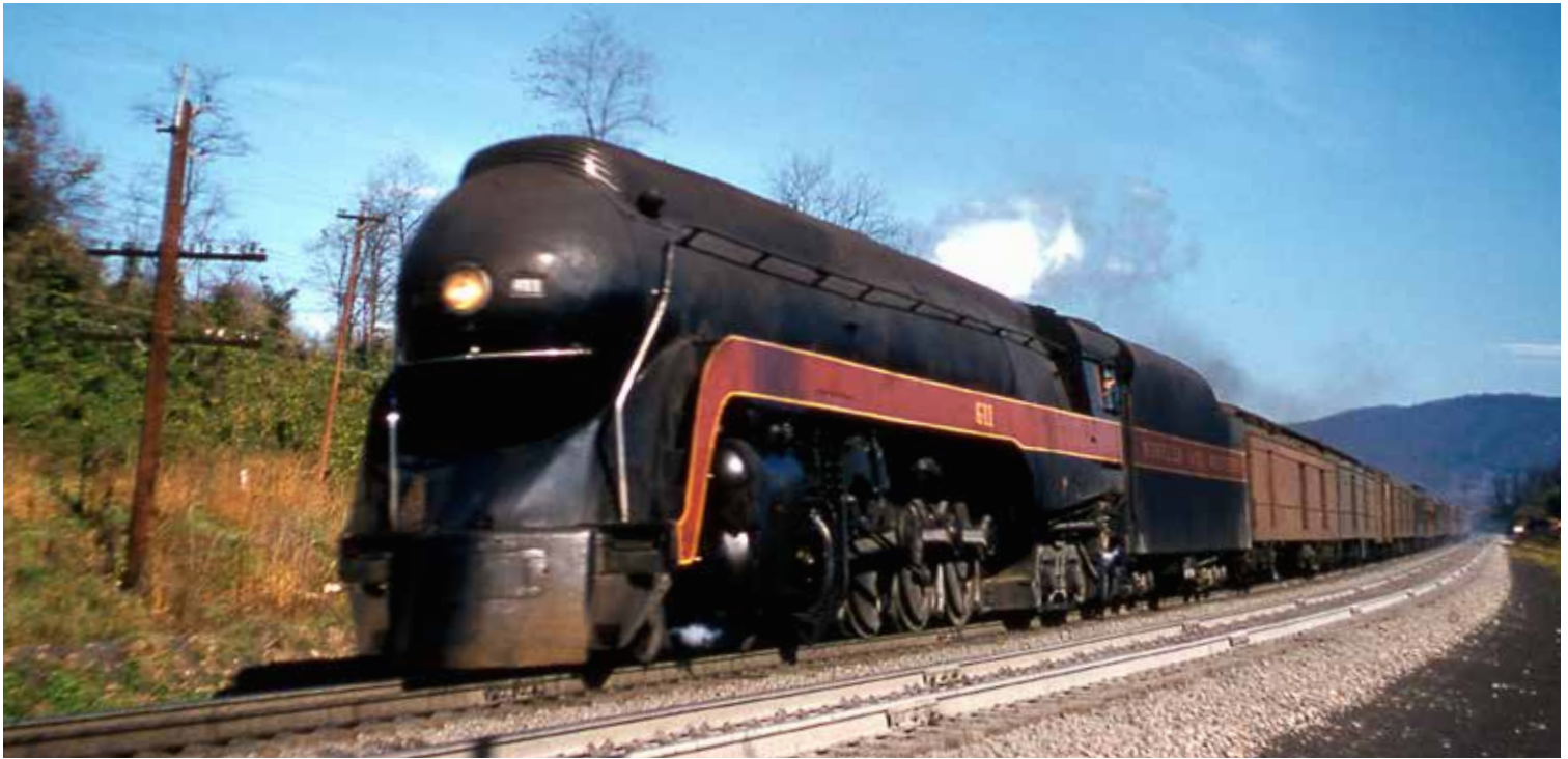
N&W class J No. 611, first of the three 4-8-4s Roanoke built in 1950, brings the westbound Tennessean down Blue Ridge Grade at Bonsack, Va., in 1956. The Js of 1950 would be America's last 4-8-4s, and 611 would be reactivated for excursion service twice, in 1982 and 2015. Bob Krone
