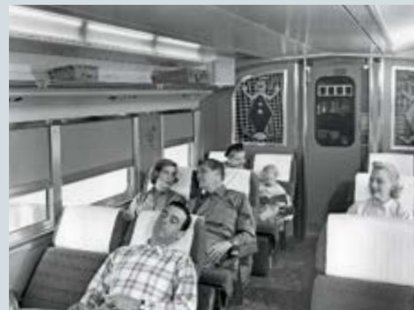
The Santa Fe Hi-Levels feature reclining leg-rest seats, air-powered sliding doors, and Southwest Indian imagery. Budd Co.
