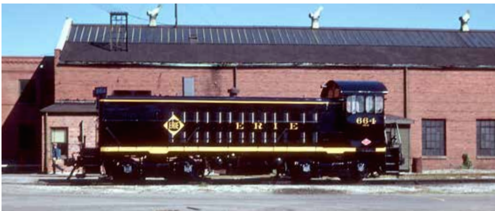
Lima, the last builder to give up on steam, launched a diesel line in 1949 after merging with engine-maker Hamilton. Erie 664, a 1,200 h.p. switcher, was built in August 1950, two months before Lima-Hamilton merged with Baldwin. Barney L. Stone, Krambles-Peterson Archive
