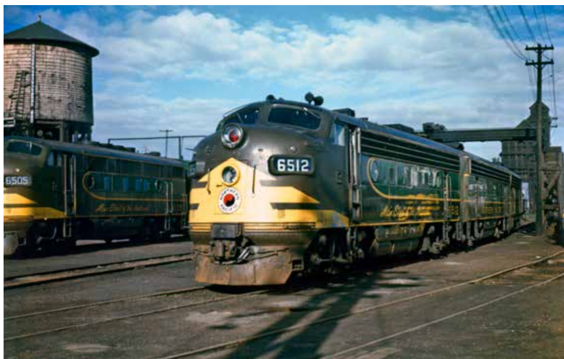
Pre-Loewy NP power: Northern Pacific passenger F3A 6505 and F7A 6512 idle with their companion B units at Seattle in the early 1950s. The color scheme the diesels wear gave way to the two-tone green livery created for NP's passenger trains by designer Raymond Loewy's firm in 1952. Tom Miller, Steven Thompson collection
