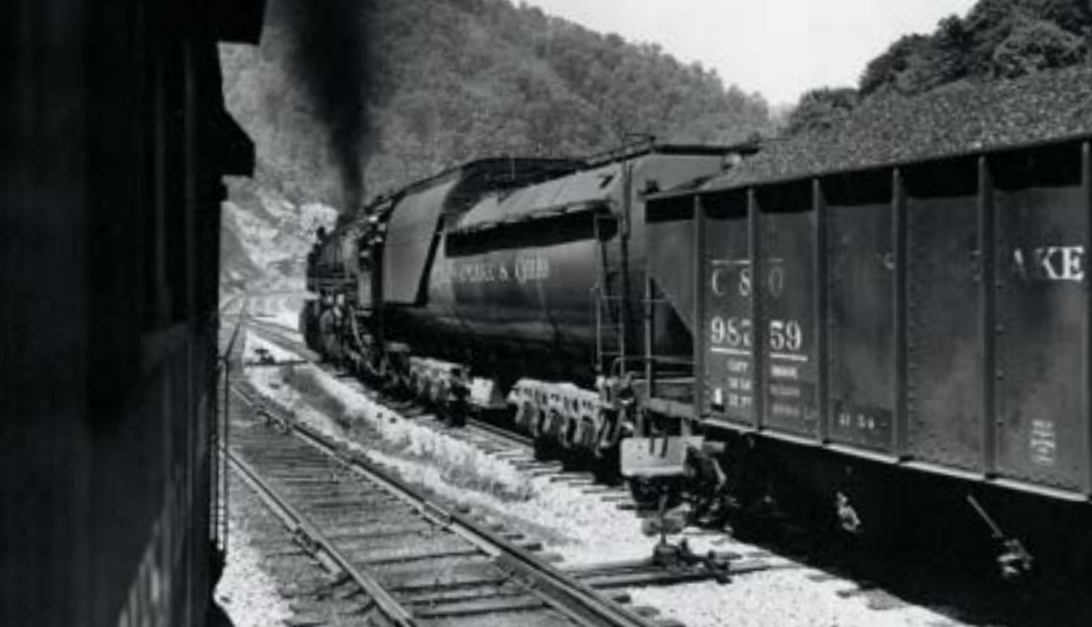
Mallet 1498 starts downgrade to Barrett with loads from Wharton No. 2 mine. The train's caboose (vantage point for the photo) will follow, its crew using the hand brake to control speed as a flagman hops off and on, resetting switches and derail devices.
