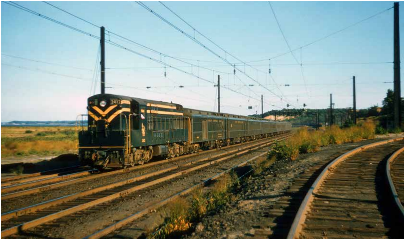
Train Master under wire: Jersey Central 2412, a Fairbanks-Morse H24-66 Train Master, approaches South Amboy, N.J., with a passenger train in August 1957. This is the New York & Long Branch, the joint Pennsylvania-CNJ line up the North Jersey coast; the catenary, which ends at the signal bridge in the distance, is for PRR trains. Curving off to the right is the connection to short line Raritan River Railroad. Jack Raymus, Krambles-Peterson Archive
