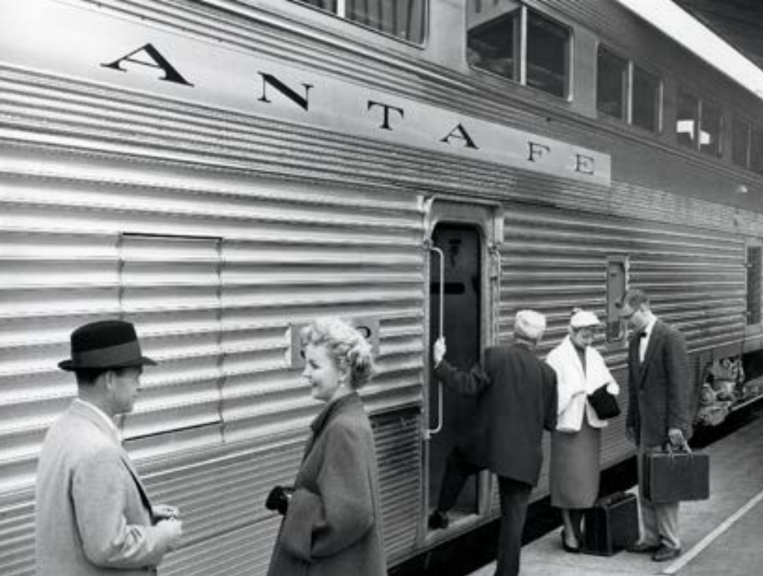
Among the Hi-Levels' new features is the low boarding door. Passengers can board from a standard platform without climbing vestibule steps or even needing a step box. Santa Fe
