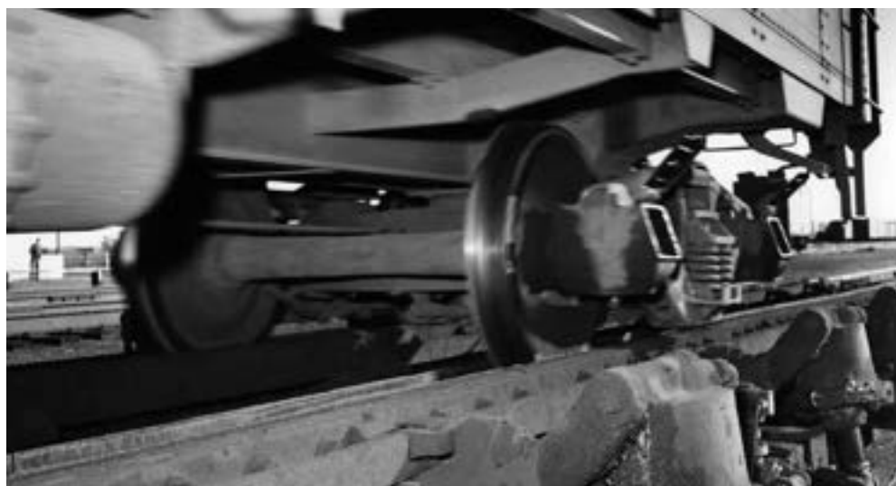
Air-operated pistons press steel bars against car wheels as they pass over the retarders. Journal-box covers are open for inspection and addition of lubricant if needed. Both, UP
