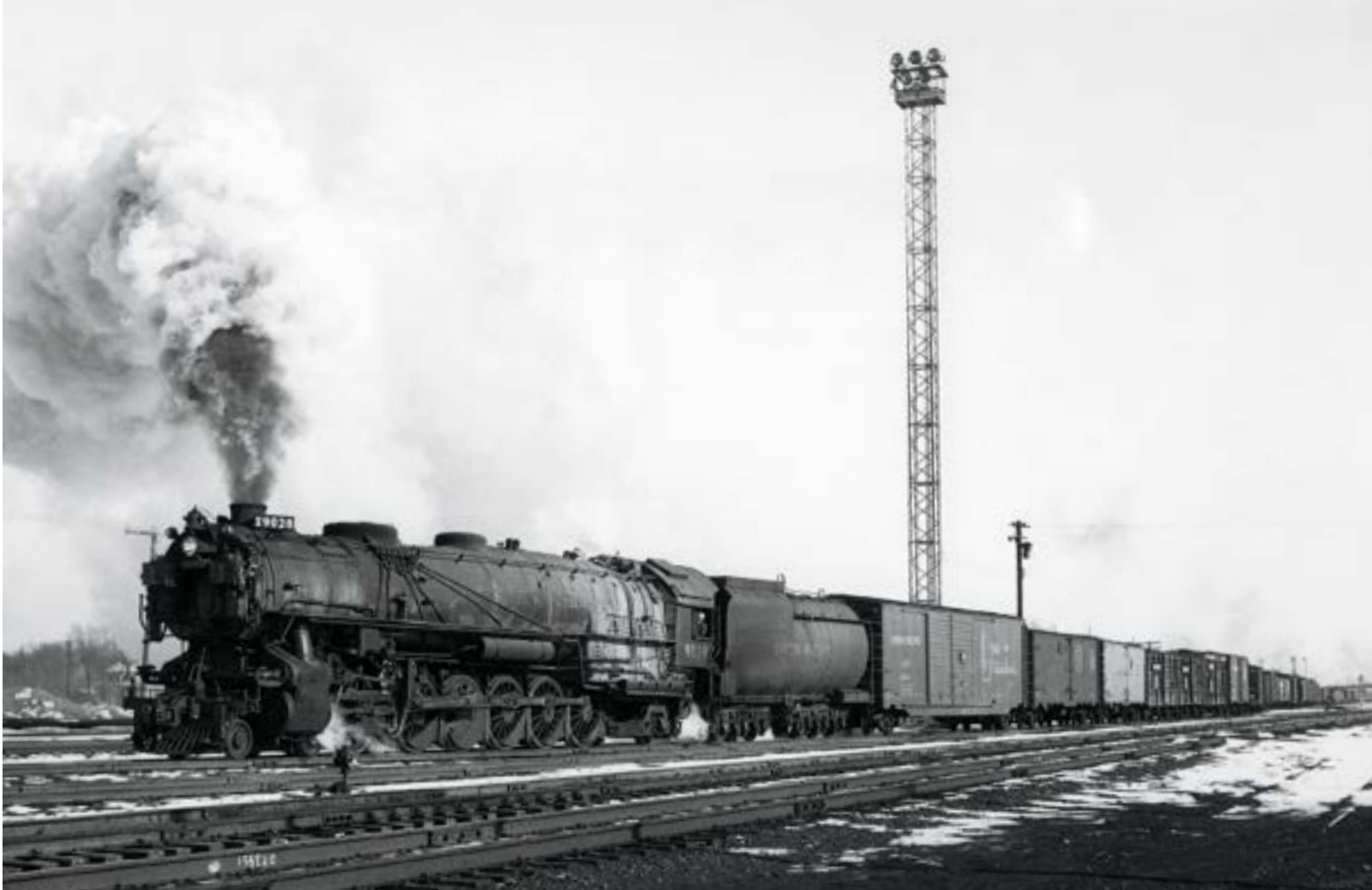
In early 1954, 4-12-2 No. 9028 brings a train into North Platte from the east. Only UP had 4-12-2s, 88 built during 1926–30. Art Stensvad
