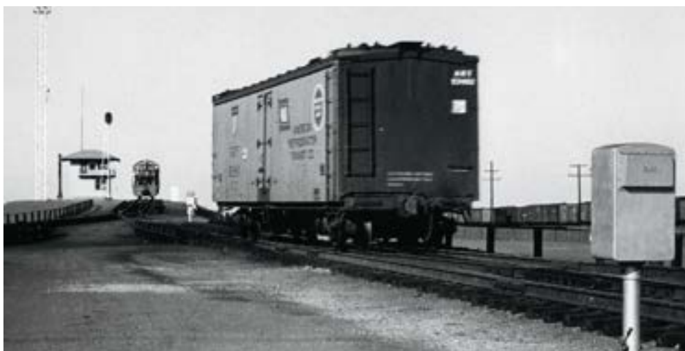
Having rolled free of the NW2 in the background, a refrigerator car headed for the bowl of the yard approaches a box containing a radar speed-monitoring device. Union Pacific
