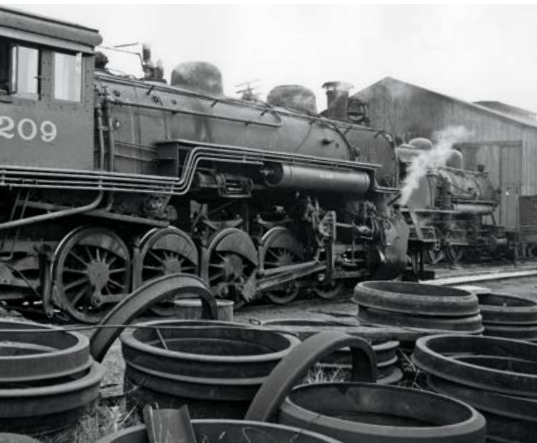
Stacks of driving-wheel tires keep company with 2-10-0 No. 209 and half-century-old slide-valve 2-8-0 No. 116 (the Midland's senior engine) at Gainesville.
