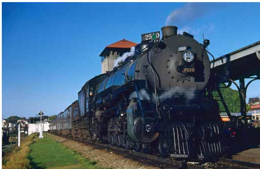
Cascadian at Everett: Great Northern 4-8-2 No. 2510 stands with the Spokane-Seattle Cascadian at Everett, Wash., on September 5, 1950. The green-painted 1923 Baldwin was upgraded after World War II with roller bearings, twin sealed-beam headlight, and other improvements. H. M. Stange, Krambles-Peterson Archive
