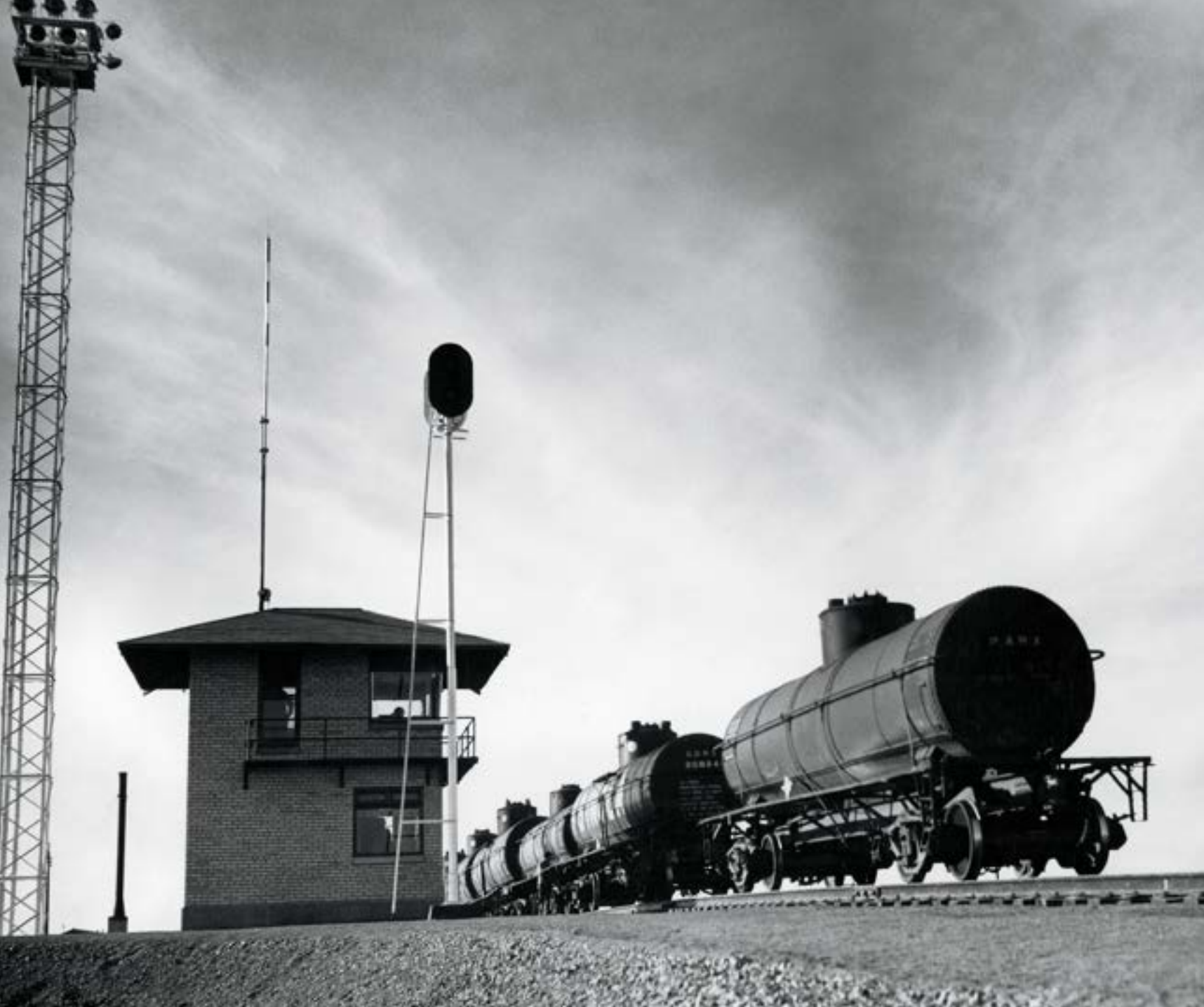
A tank car begins its descent from the crest of the hump at UP's new North Platte yard. The mast atop the hump control tower is for radio communication with switch engines. A hump conductor directs the pin-puller from a position on the ground floor. Wallace W. Abbey
