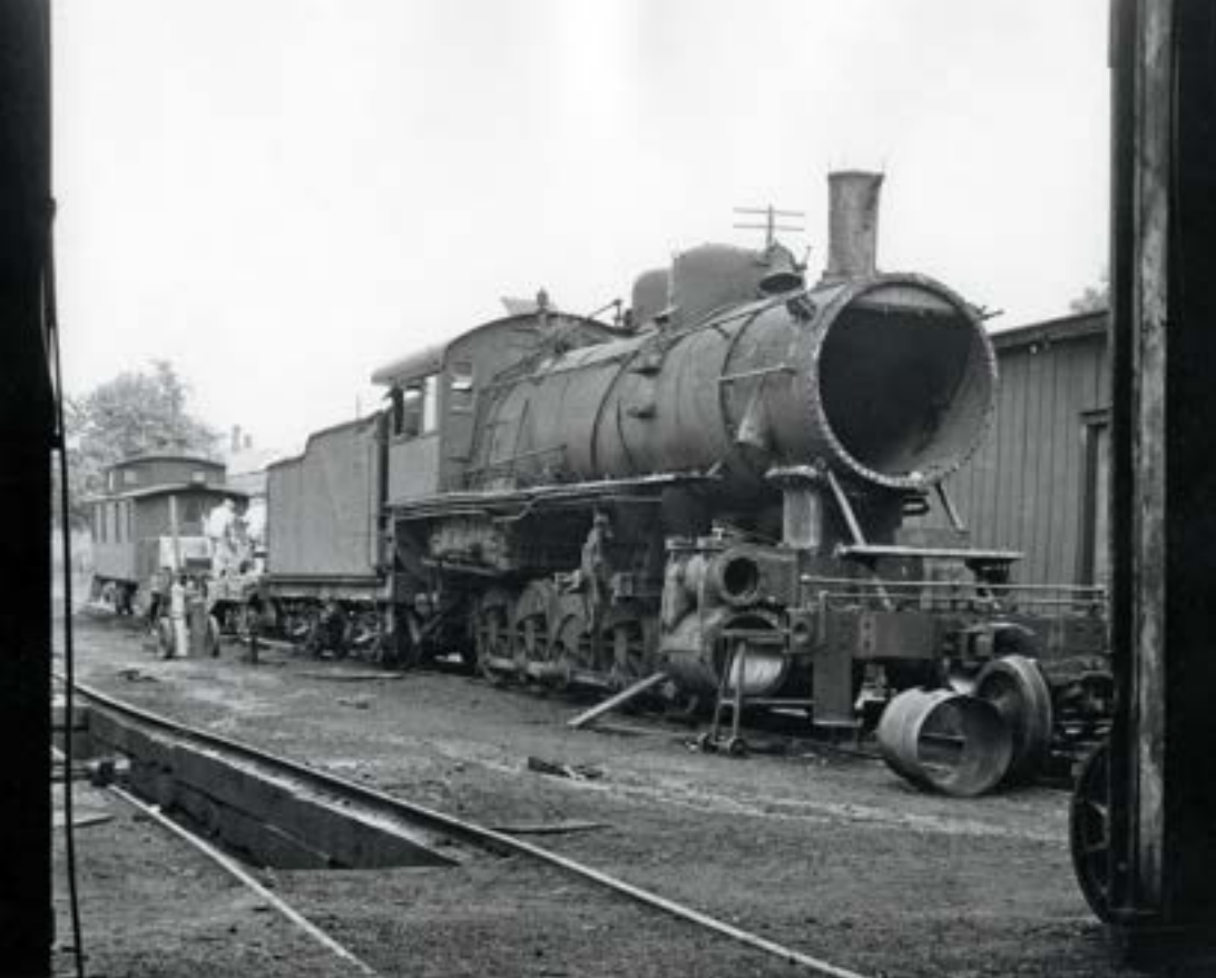
Engine 206, one of 200 light 2-10-0s built for export to Russia during World War I but stranded stateside after the 1917 Soviet revolution, is partially torn down for repairs outside the Gainesville shops. The 52-inch-drivered engine is GM's only Russian Decapod.
