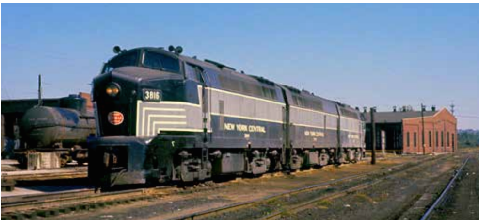
Big roads like New York Central tended to buy from all diesel builders. Along with legions of EMD and Alco-GE freight cab units, NYC rostered 25 (17 cab, 8 booster) Baldwin 1,600 h.p. "Sharknoses," three of which rest at Sharonville, Ohio, in 1960. Tom Gildersleeve
