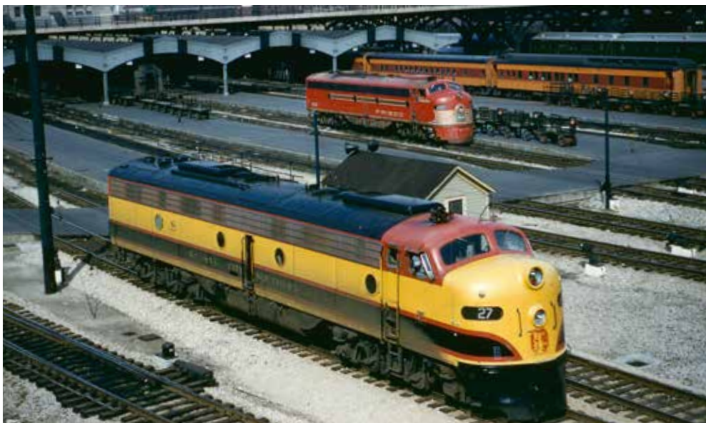
KCS and Frisco E8s mingle at Kansas City Union Station in April 1954. Electro-Motive built 460 of the 2,250 h.p. passenger units during 1949–53. Dick Neumiller, Bon French collection
