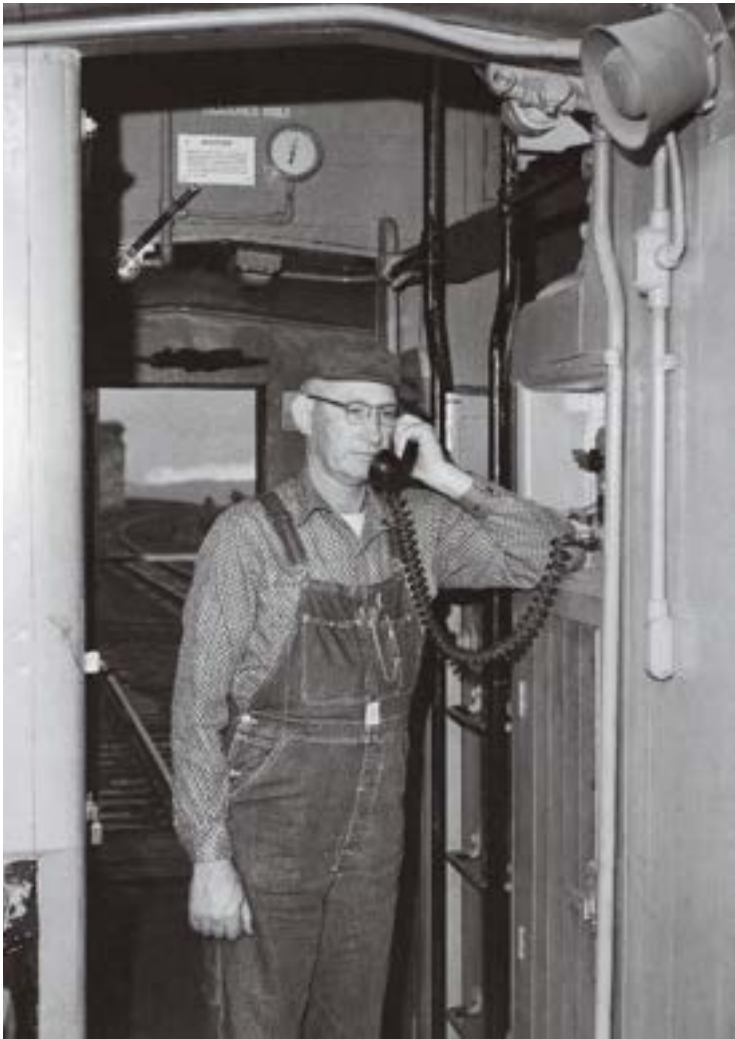
Conductor Bert Elam talks with the train's engineer over the caboose's Bendix radio set, whose speaker is at top right of photo.
