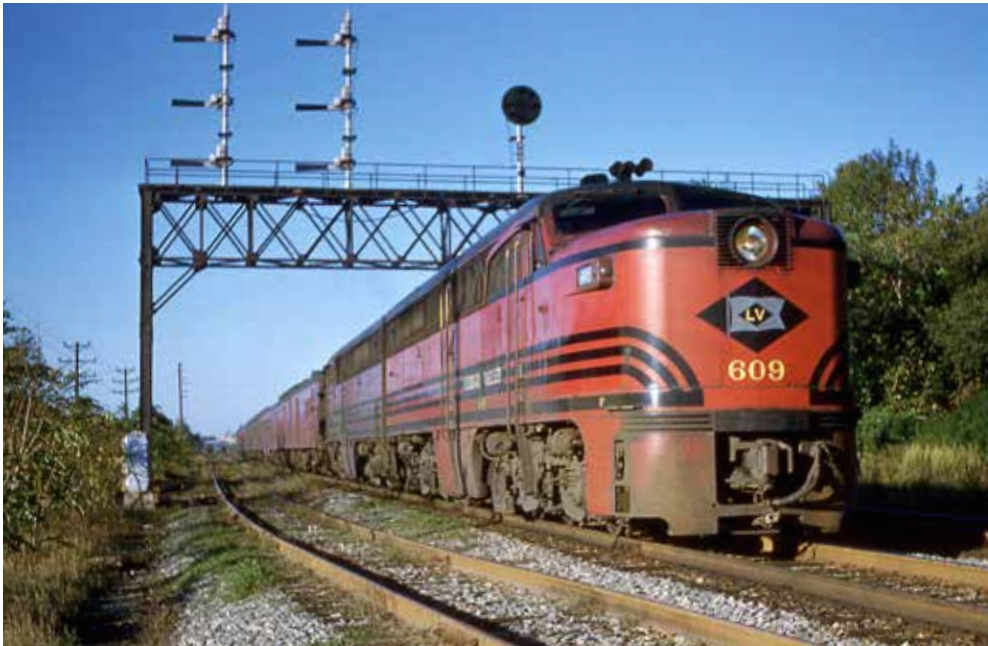
Two of Lehigh Valley's 14 Alco-GE 2,000 h.p. passenger units (later dubbed model PA), bring the eastbound Maple Leaf into Newark, N.J., in September 1960. The PA dominated on a few roads, but overall was a distant second to EMD's E units. Richard Steinbrenner
