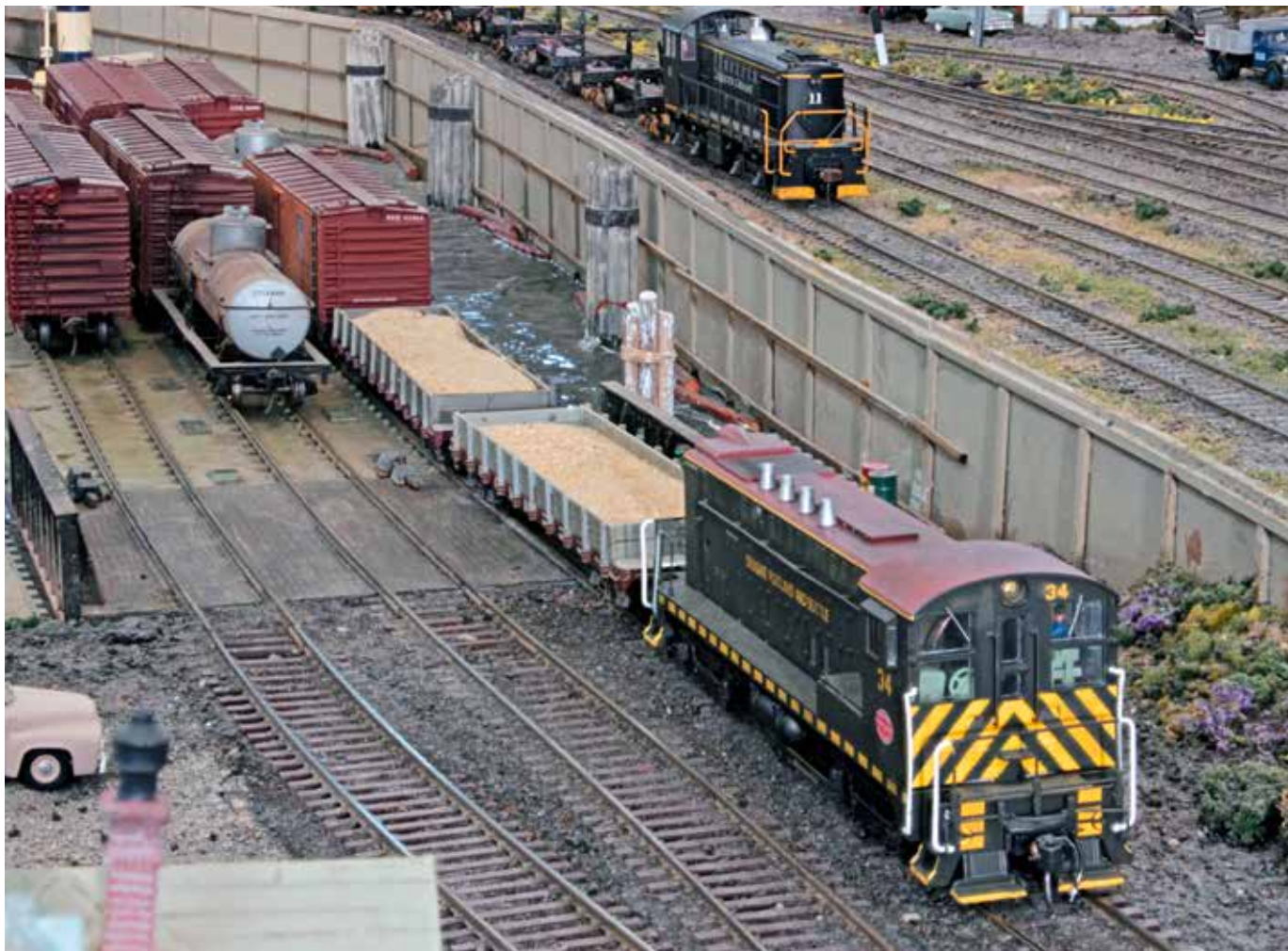
Mat Thompson uses continuous rail across the apron and onto float to eliminate possible derailments. He painted, thus insulating, the top surfaces of the apron and float rails to require the operator to switch the float using idler cars with the locomotive still on land. Mat Thompson photo
