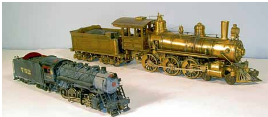
Andrew appreciates the greater heft of O scale models – note the size comparison between an HO 2-8-0 Consolidation and one of his scratchbuilt Proto:48 Colorado Midland 4-6-0s. A 19th-century CM Ten-Wheeler locomotive would be very small in HO, but its compactness is a virtue in 1/4" scale.
