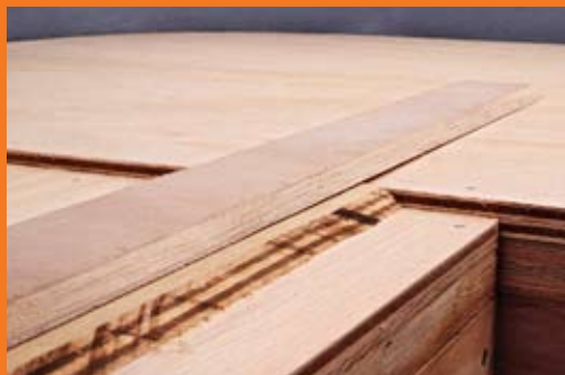
He cut the roadbed for his layout from 1/4" lauan plywood.
