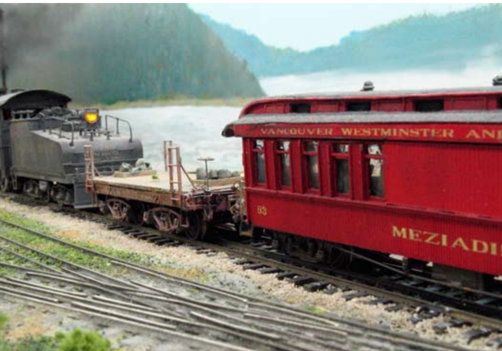
At the dual gauge yard in Sicamous, a standard gauge 0-6-0 makes up the narrow gauge passenger car consist of VW&Y train No. 2, the Sourdough . The switcher uses an idler car with both standard and narrow gauge couplers.
