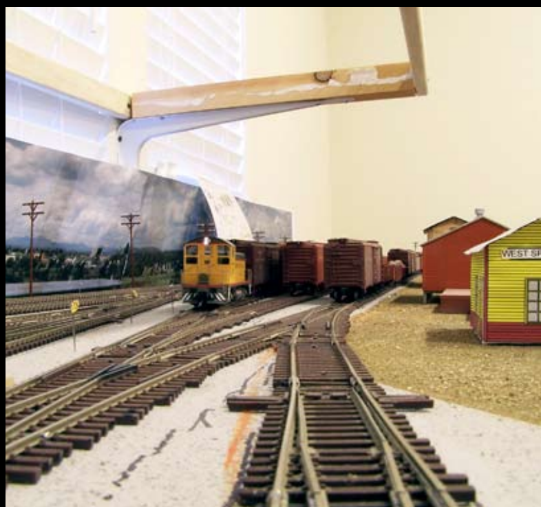
Inexpensive L-shaped shelf brackets support the lightweight upper deck above West Spokane.
