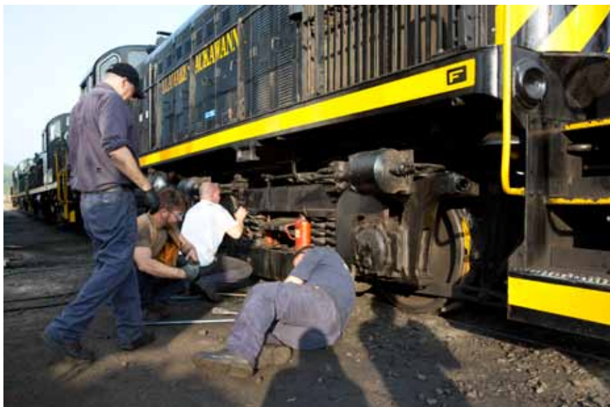
With precision and coordination befitting a NASCAR pit crew, the Scranton shop force tends to a broken equalizer bolt on D-L No. 4068. Left to right: Don Colangelo, Micah-John Kirstner, Bill Strein, and Billy Birdsall.
