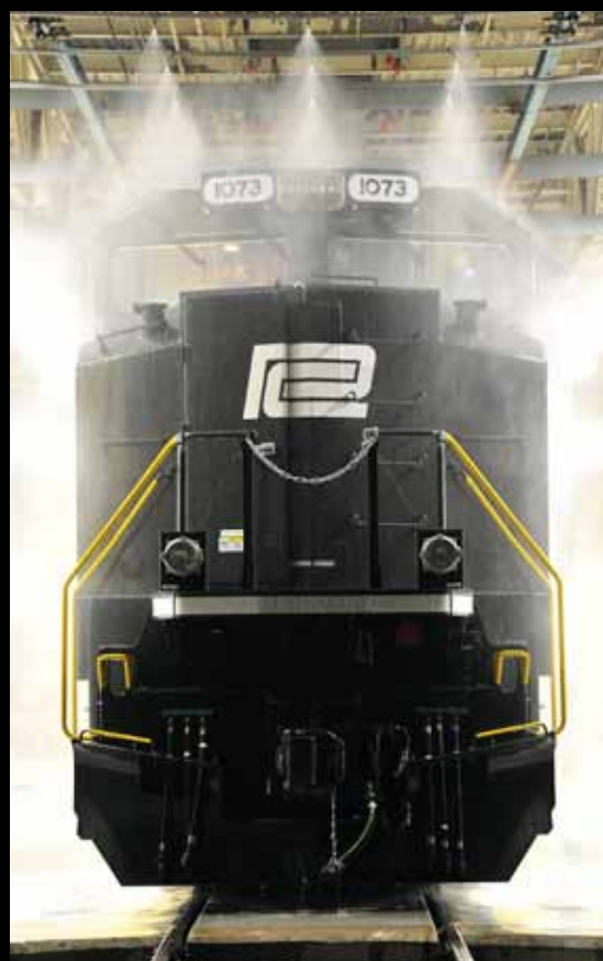
Water jets blast Penn Central-painted Norfolk Southern 1073 as the newly completed SD70ACe undergoes pre-delivery tests at Progress Rail Manufacturing's locomotive plant in Muncie, Ind. NS: Casey Thomason
