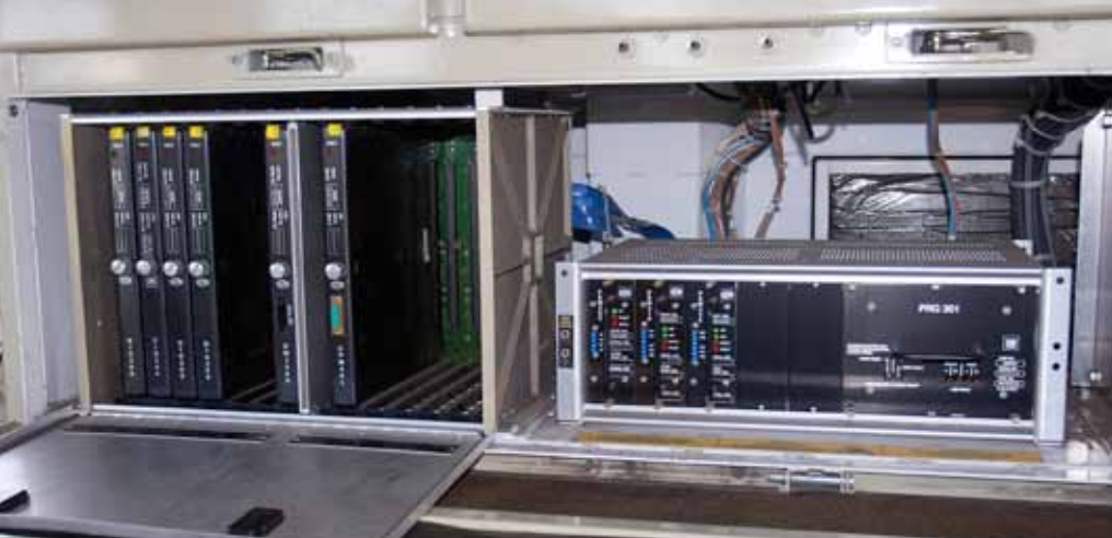
The brains of a typical EMD EM2000 Dash 3 upgrade: the large box on the upper right is the PRG301 and related modules that form the power supply regulation system. To its left are cards that monitor, operate, and control various functions of the locomotive. At right, is the EMD user interface with specific function keys and directional arrows for paging through the data displayed on the screen.
