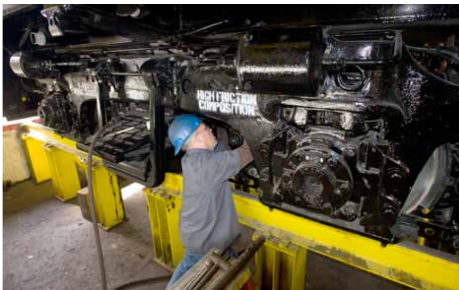
In the main locomotive shop, Jerry Strobel works on the reconditioned truck of a freshly overhauled and repainted Helm Financial GP38-2.
