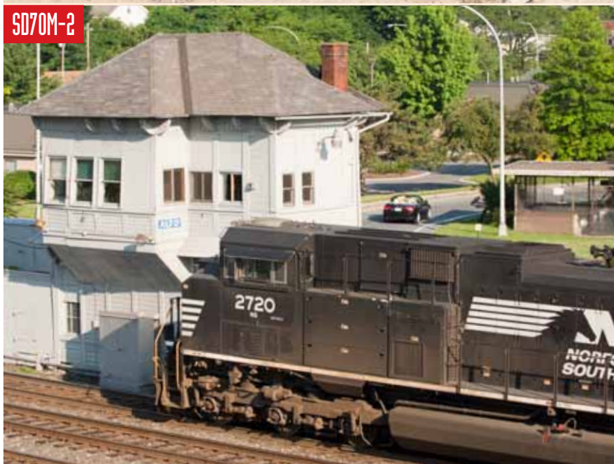
On Union Pacific SD70ACe No. 8451 (top), you can see air intakes on its equipment box behind the left-hand side of the cab. Norfolk Southern SD70M-2 No. 2720 doesn't have this feature. Two photos, Greg McDonnell
