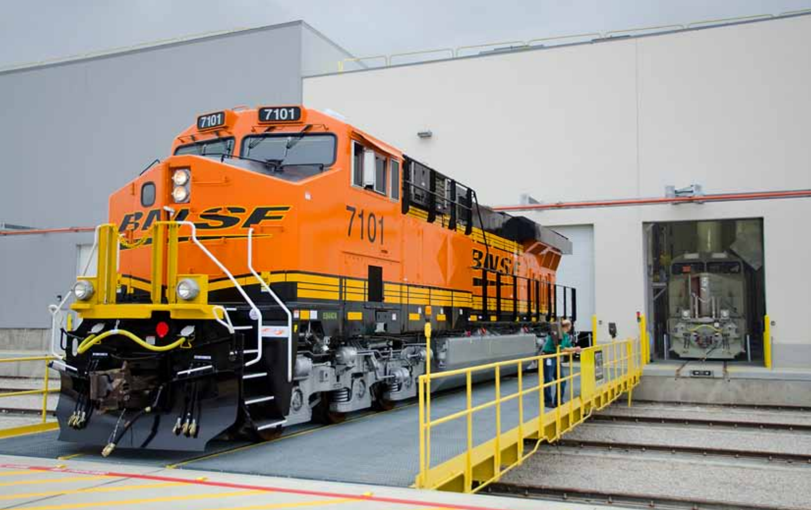
BNSF ES44C4s began rolling off the assembly line at GE Transportation's new locomotive plant in Fort Worth, Texas, in March 2013. One of the first to be completed, BNSF 7101 rides the transfer table. GE: Steve Gerbracht
