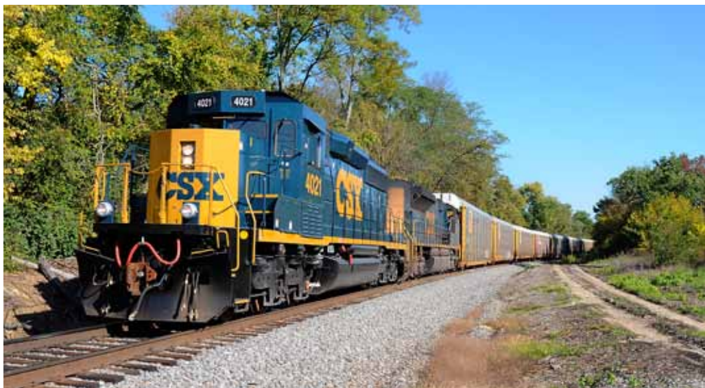
Customized nose and cab design gives CSX SD40-3 rebuilds an unmistakable look. No. 4021 leads an SD70MAC at Walton, Ky., in October 2011. Brian Schmidt
