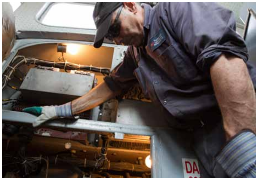
Chief Mechanical Officer Don Colangelo in the cab of Central Railroad of New Jersey 1554: manual transition, Amplidyne excitation, and components in common with Boeing B17 bombers of World War II.
