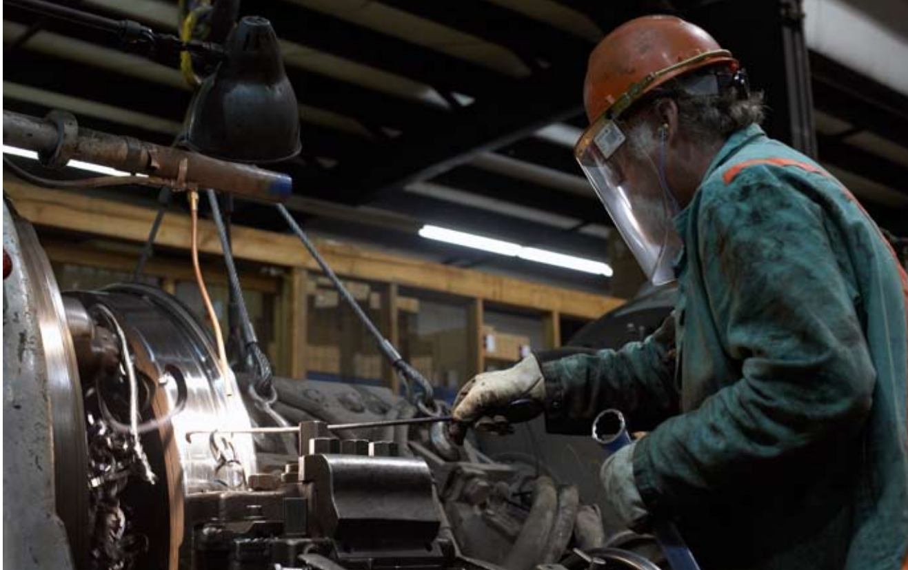
Re-profiling No. 3004's wheels, Richard Brown works on the steam-era lathe.
