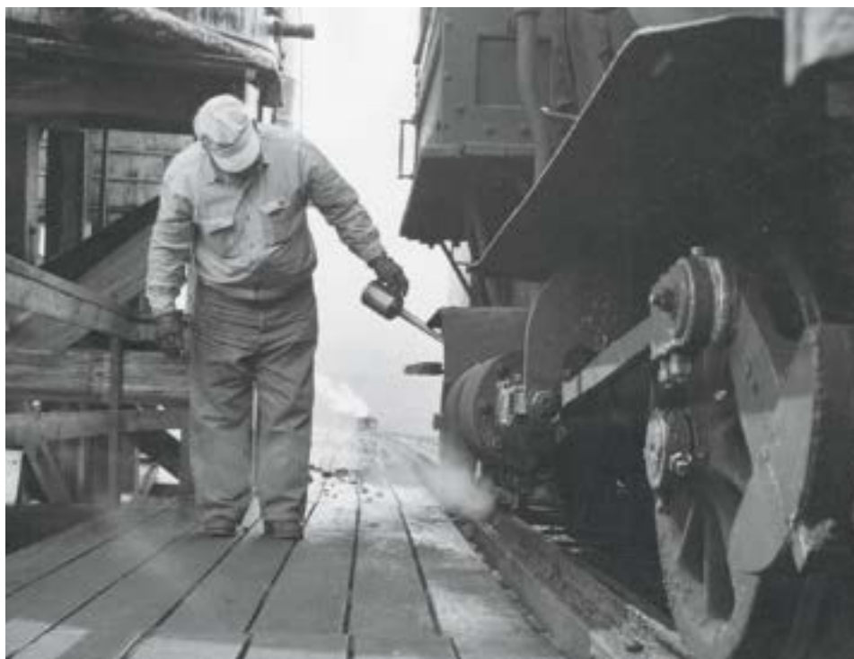
Engineer oils around Engine No. 4 after taking water at Waumbeck Tank, N.H. In the distance, another train climbs the mountain.
