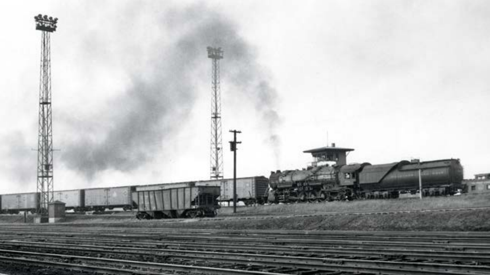
S-1 2-10-2 No. 6174 backs up the hump at Willard, O., with reefers — to B&O what Decapods were to the Pennsy.
