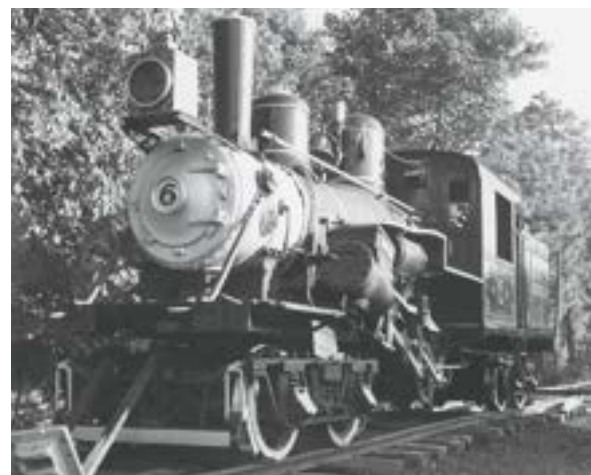
Climax geared locomotive No. 6 preserved at Clark's Trading Post — trundling along on interurban-type trucks.
