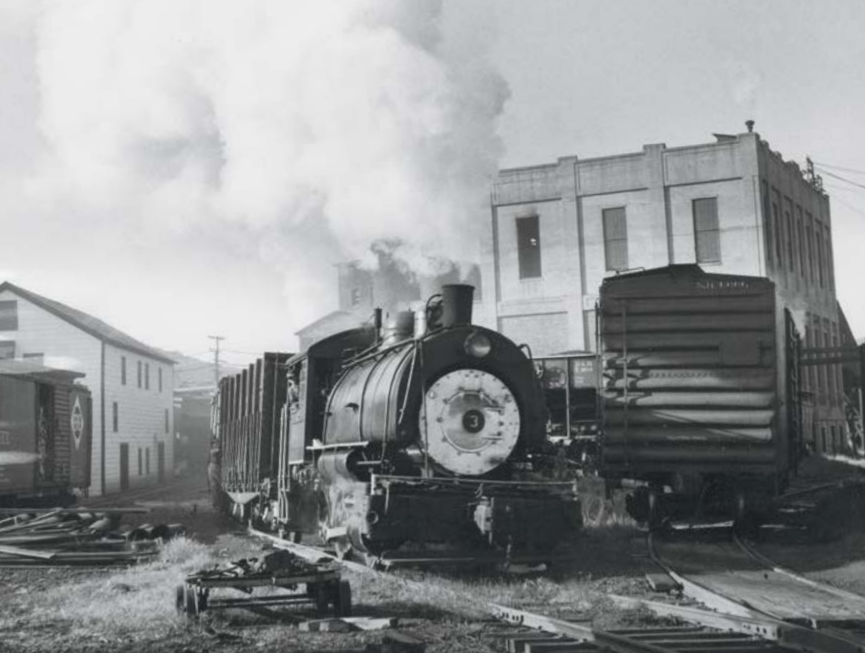
The kid is No. 3, a Porter 0-4-0T of 1917 which EB&L obtained from the Watertown (Mass.) Arsenal in 1945.
