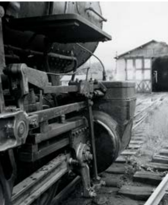
Valve motion of East Broad Top's Three-Spot — in deepest twilight ... for good.
