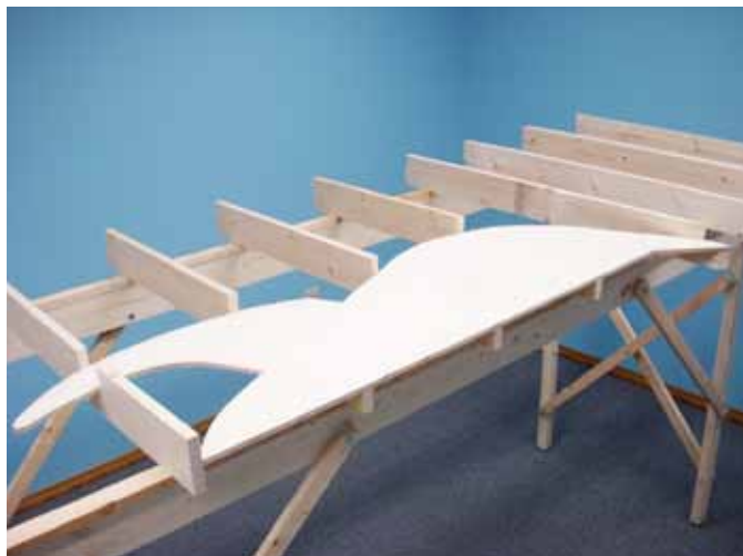
Here the grade-level plywood has been removed and the wash bed plywood put in place. A few additional supports were needed to keep the plywood from sagging between joists.
