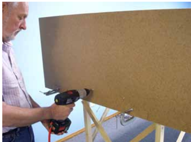
Stener attached large hardboard pieces to the ends of the layout with screws. He used clamps to hold the hardboard in place during this step. The scrap pieces of hardboard prevent the clamps from damaging the surface.
