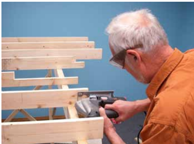
After marking the edge of the creek bed and wash on the joists, Stener measured down 2" and then used a saber saw to cut the joists. These slimmer, cut-down joists support the base for the plywood creek.
