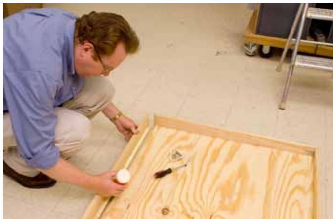
A frame of 1 x 4 lumber around a plywood panel provides a sturdy support for the foam board base of the layout.
