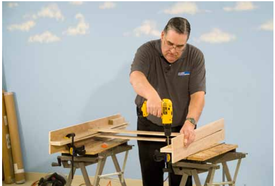
To make the leg sections interchangeable, Jim clamped them back to back and then drilled the holes for the bolts that will mount them to the tabletop. This way both legs will fit on either end of the table.
