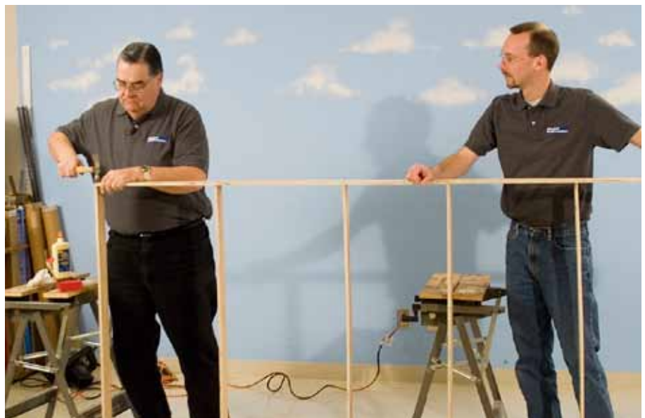
With David's help, Jim assembled the tabletop frame. He used carpenter's glue and trim nails to secure each joint. Before the glue set, Jim squared up the frame and added the \frac{1}{4} " birch-plywood top.
