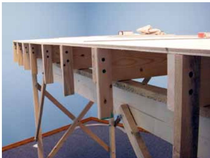
Dick and Stener used glue and screws to attach vertical 7" lengths of 1 x 2 to the side of the joists to support the layout's tempered hardboard fascia. They secured the fascia with screws.
