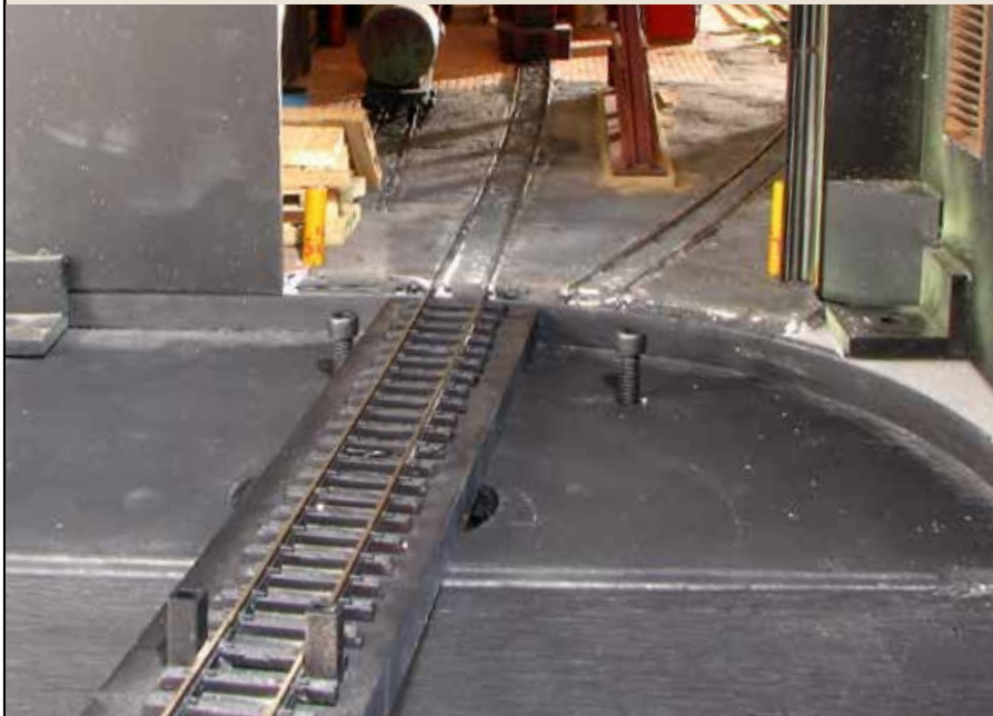
Brian uses two locator posts to align his sector plate with the track.
