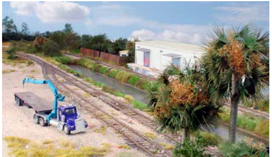
The two major features required at a team track are truck access and a means to load or unload cargo. Today, trucks are often equipped with unloading devices, as in this scene on the Lance's Florida-prototype HO East Rail layout.
