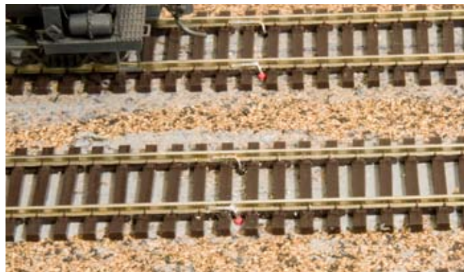
Fig. 2 Dog-leg feeder. Solder small-diameter solid wire to the base of the rail, as here on Model Railroader's Wisconsin & Southern HO layout. Solder neatly and it's safe to do this on the gauge side of the rail, so all feeders can be opposite the aisle or normal viewing position. MR staff photo
