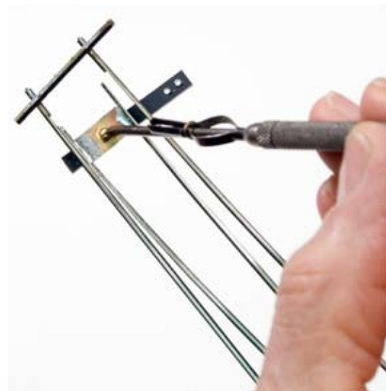
Fig. 11 Switch rod pivot. John uses a modified round-head screw as a pivot that passes through the point spacer and is threaded into the switch rod.
