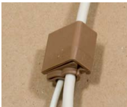
Fig. 7 Snapped shut. After the knife is pressed flush, the “suitcase lid” can be closed to cover the bare metal and safely insulate the connection. The brown no. 567 connector can handle wire sizes up to 10AWG on the through or run side, making it ideal for bus connections on many DCC layouts.
