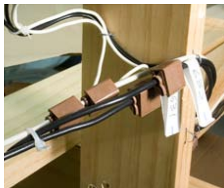
Fig. 9 Bus connections. Andy connects the 18AWG feeder extensions to 12AWG bus wires with no. 567 connectors. The white wire is the common rail bus and the black wires are separate buses for each signal block. The white tags identify the block buses by the signal number.
