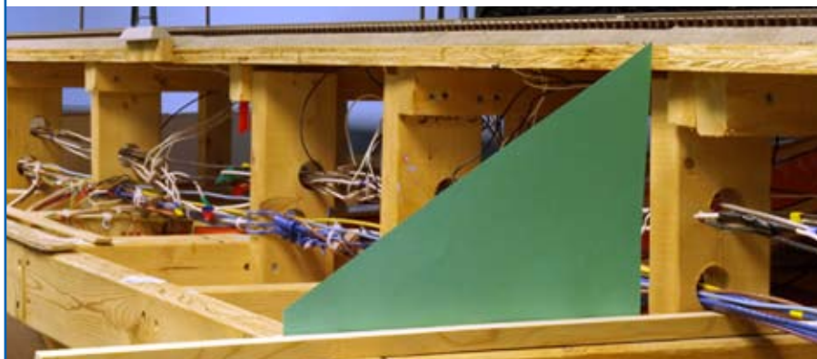
Neal cut a large piece of cardstock as a template for the 1 1/2:1 slope of a fill.
