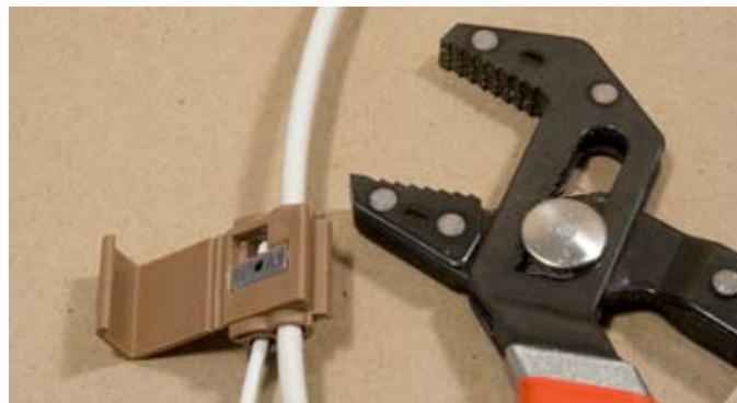
Fig. 6 Squeezing the knife. Andy uses Robo-Grip cam-action pliers to press the connector's knife flush with the body of the connector. The knife cuts through the insulation and into the metal conductors, bridging the two wires together.
