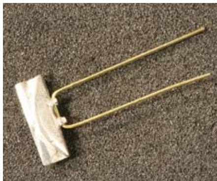
Fig. 4 Forming the hinge. Looping a wire through the holes and bending the ends down forms the hinge on which the derailing block will pivot.
