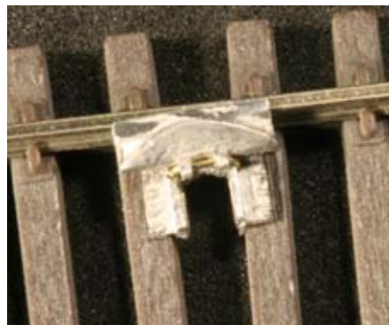
Fig. 5 Installation. To make the installation more secure, Matt glued the ends of the wire into holes drilled into the track and roadbed.
