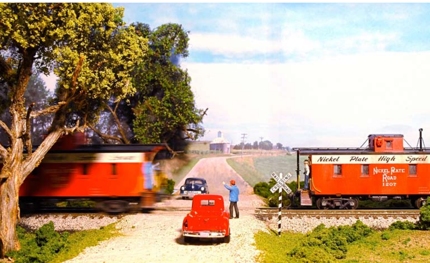
Fig. 3 High iron. Tony elevates his main track (foreground) \frac{1}{2} " above the subroadbed, which is high enough to allow for drainage ditches along the right-of-way. Passing tracks are elevated \frac{3}{8} ", or about a scale foot lower than the main.
