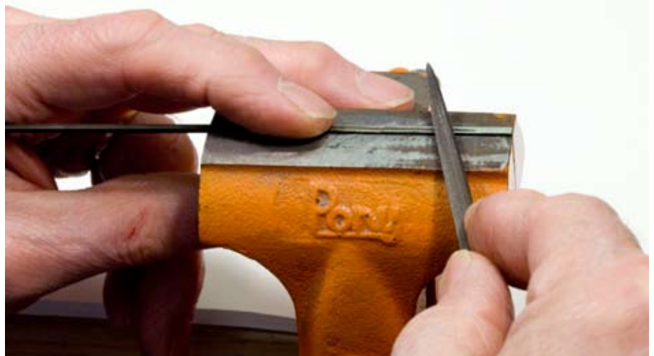
Fig. 4 Shaping rails. John clamped each point rail in a smooth-jaw vise so he could file it into the long, smoothly-tapered point needed for good performance.
