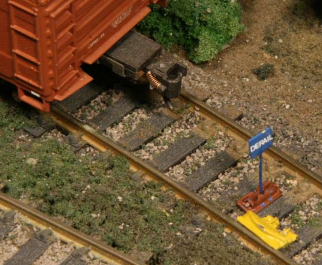
A hinged derail and folding marker sign protect the main line on Matt Snell's HO scale layout. If the boxcar rolls, the derail will stop it before it fouls the main.
