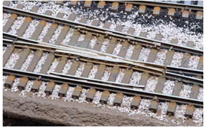
Fig. 4 Frog castings. Tony uses Details West code 70 no. 8 manganese-insert frog castings for mainline turnouts. They drop accurately into place on Central Valley tie strips. Cyanoacrylate adhesive (CA) and four spikes hold the new frog in place. The frog feeder wire is soldered into the outside crotch of the frog and connected to an SPDT toggle or slide switch or switch motor contacts.
