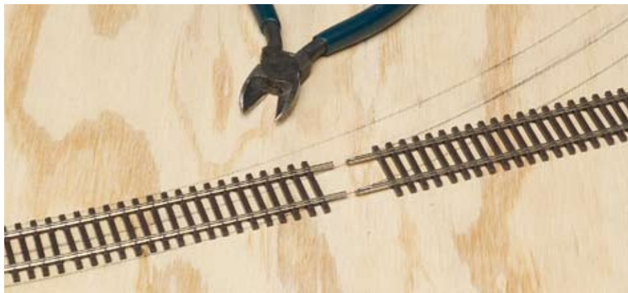
The Atlas code 83 HO flextrack at left is laid on a 26" radius, except for the last three inches. After trimming the rails on that section for a square joint, Andy Sperandeo is ready to add a new section that's still straight. Bill Zuback photos
