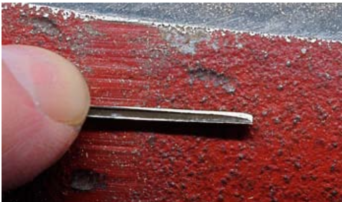
Fig. 7 Filing switch points. Tony makes his switch points by filing lengths of Micro Engineering code 70 rail. The gauge side of the tip of each point is tapered as well as chamfered to ensure it won't catch a passing wheel flange. The base of the point rail must be burnished to a bright sheen to ensure it will easily accept solder.
