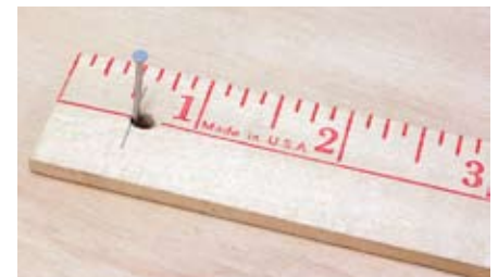
The radius center is near the zero end of the yardstick, but the exact position will depend upon width of the particular binder clip that you use. The left edge of the hole shown is equivalent to zero for the pencil location in the handle of the binder clip.
