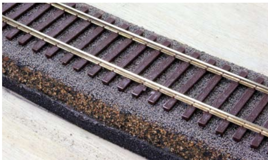
Bob found that ballasting the track had little effect on transmission of noise to the subroadbed, regardless of the roadbed material used.
