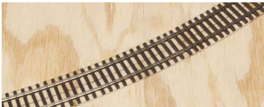
Now the joined sections are bent to the 26" radius with a smooth curve through the joint. Andy saves extra ties to fill gaps in the tie strip, and always cleans the joints with denatured alcohol to keep excess flux off wheels and railheads.
