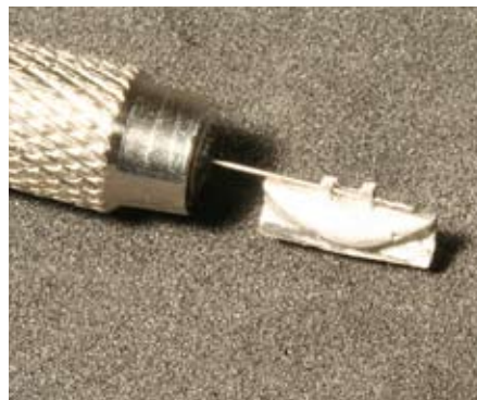
Fig. 3 Turning point. Matt drills a hole for the hinge through the "fingers" of the derailing block. The block will turn on a wire threaded through the holes.
