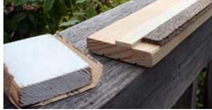
This simple fixture holds a strip of cork roadbed so the jagged corner can be sanded. Bob Kingsnorth photo
