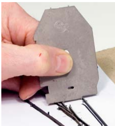
Fig. 6 Track gauge. John uses a National Model Railroad Association Standards gauge to check the spacing between the rails along both routes.
