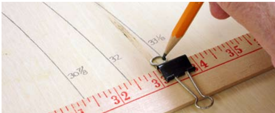
A binder clip instead of a hole drilled in the yardstick makes this oft-used tool more versatile. The left edge of the clip is set at the desired radius, and the clip handle guides the pencil point. Bob Kingsnorth photos
