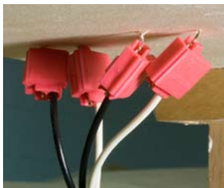
Fig. 8 Feeder extensions. The no. 22 bare feeder wires come through the bottom of the plywood subgrade, where Andy splices them to 18AWG feeder extensions. Before making the connections, he doubles the bare wire back on itself and twists it so the connector will get a solid grip.
