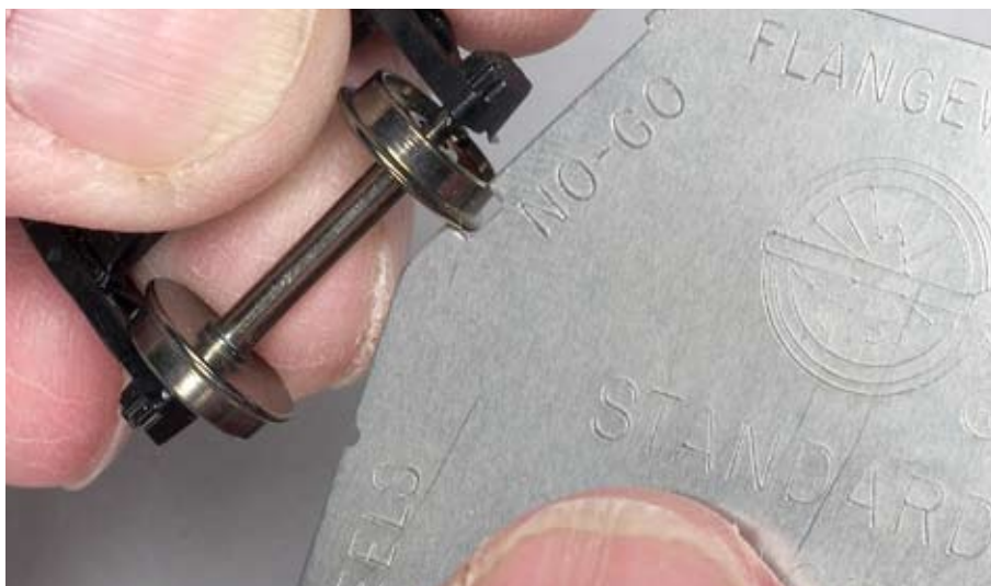
Fig. 3 Tread width. Narrow wheel treads may have problems passing smoothly over switch frogs, so this No-Go notch checks for the standard tread width.
