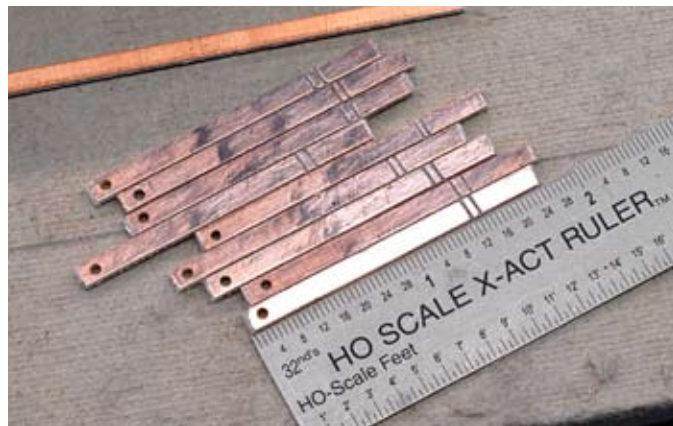
Fig. 10 Switch rods. Using printed-circuit board strips from Clover House, Tony cuts switch rods 13 scale feet long, so they reach the point-actuating wire from the switch motor outside the rails between the headblock ties. He drills a hole in one end to for the piano-wire actuating rod from a switch motor, and files gaps in the top surface to break the electrical path between the points.
