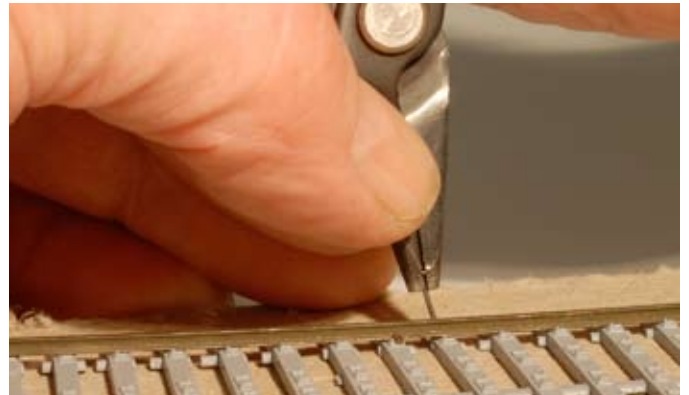
Fig. 6 Spiking rail. Spiking pliers, which have T-shaped grooves cut in the jaws to get a better hold on a track spike than needle-nose pliers, are handy tools for tracklaying. Spiking through the hollow plastic ties of the Central Valley tie strip requires a few seconds of steady pressure. Use your free hand to steady the the pliers near the tip or you'll risk bending a lot of track spikes.
