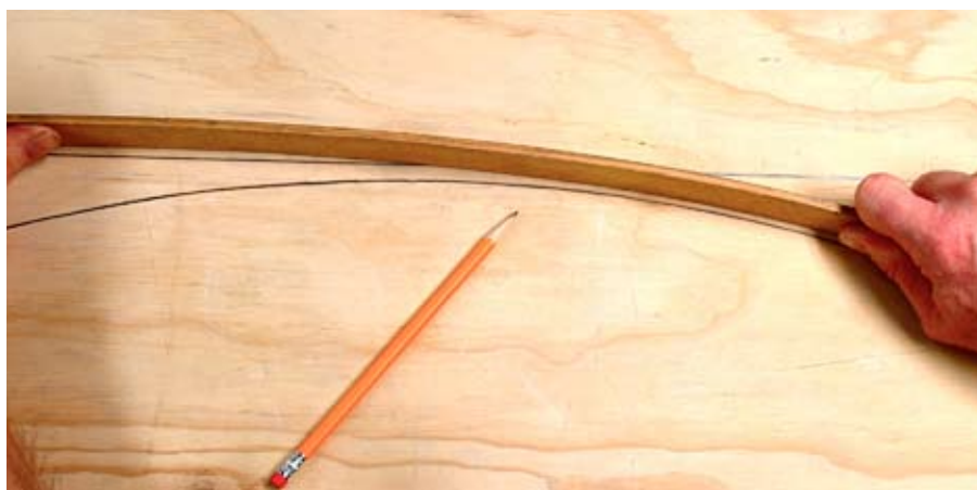
Fig. 7 Easy easements. A wooden batten strip's natural bend approximates a spiral easement between a tangent track that's offset about 3/8" from the curve radius and the circular arc. The easement should be at least as long as your longest car and maybe half a car-length longer.
