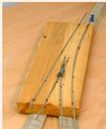
Curved to fit. To build a curved turnout for Curtis Junction, Paul used the HomaBed roadbed as a guide to draw the turnout plan on a block of wood. Then he took the block to his workbench to build the frog to fit the curve. You can see the finished turnout in the large photo on top of page 52.
