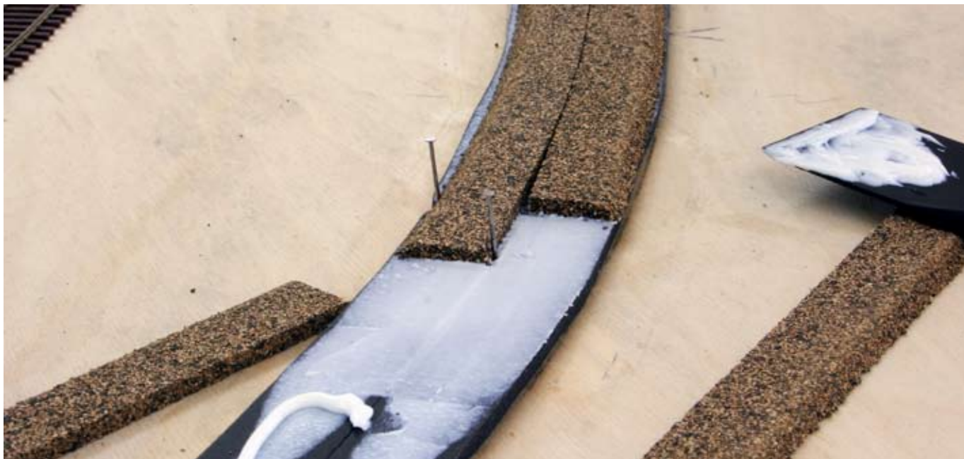
The tackiness of the caulk is sufficient to hold cork, Homabed, or Flexxbed on a curve, except at the ends. Even at a fairly gentle 32" radius, a couple nails or pins are needed to hold the roadbed in place until the caulk dries.
