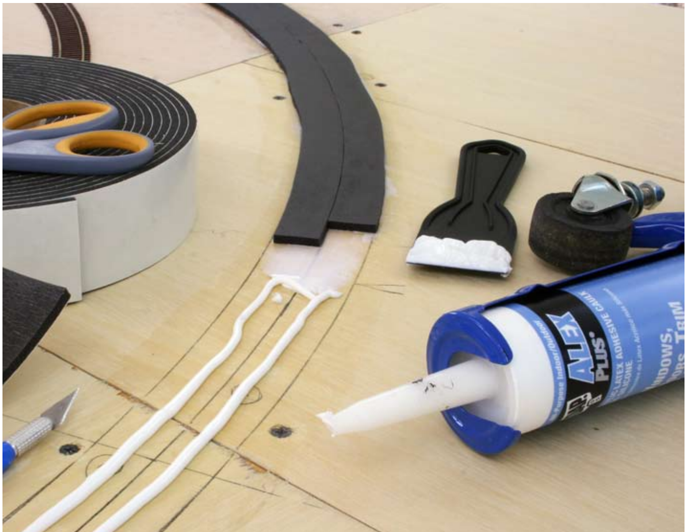
The camper tape's paper backing must be removed to allow it to be bent around curves. Bob cuts the tape into two narrow strips to make it easier to flex without kinks. He glues it to the plywood subroadbed with latex adhesive caulk.
