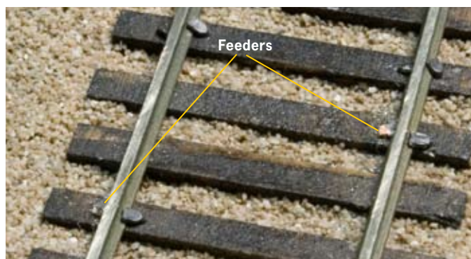
Fig. 4 Hard to find. Andy left one of his spike-head feeders unpainted so the bare metal would show up in the photo. It's inside the rail on the right. When painted, these feeders are hard to tell from track spikes, and Andy sometimes has trouble finding one when he wants to show them to visitors.
