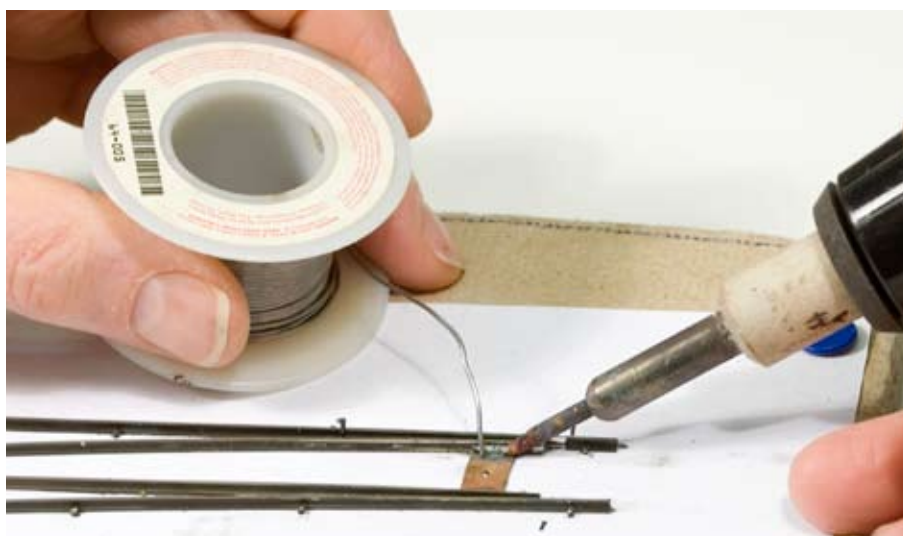
Fig. 9 Soldering the points. Installing the point spacer plate requires careful soldering to produce a clean, strong joint that clears the wheel flanges.
