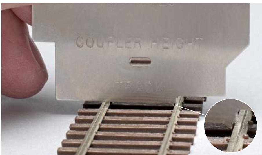
Fig. 4 Track gauge. A pair of pins check the spacing (gauge) of the rails, while a small step alongside the right-hand pin indicates if the gauge is too wide.
