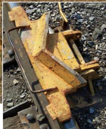
Fig. 1 The prototype. This hinged derail is double-ended and will derail cars from either direction.
