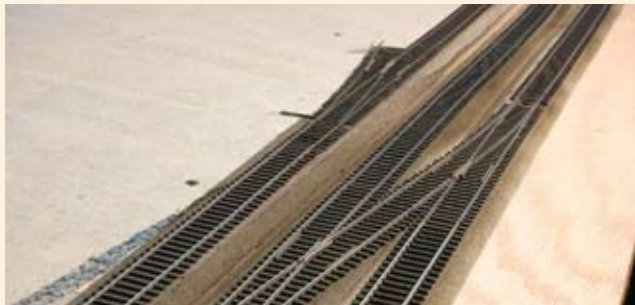
Varieties of track. This view at Highlandtown shows how Paul combines Atlas code 83 flextrack with Micro Engineering turnouts and code 70 flextrack.
