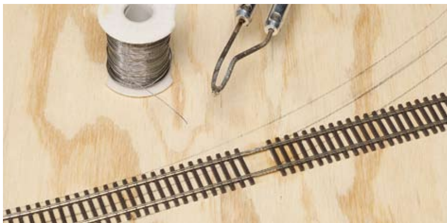
Andy has joined the two sections with rail joiners, and soldered the joiners with the rails still straight through the joint. Small-diameter rosin-core solder makes it easier to make a neat, strong joint without building up excess solder.
