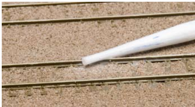
Fig. 8 A guiding rail. To prevent the pipette from dragging in the ballast, Cody propped it on the rail. He applied light pressure to the pipette so the matte medium would trickle out and not wash away the ballast.
