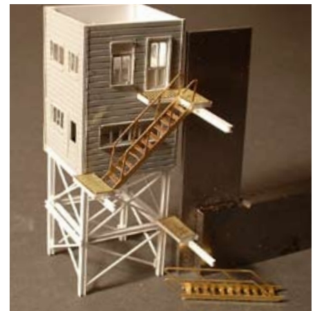
Fig. 7 Test-fitting platforms and stairs. After building the platforms and bending the stairways to shape, Jim test-fit the parts. He used the square to line up the high and low platforms.
