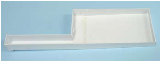
Fig. 6 Styrene mold. Lance built this styrene form to cast his model ramp from fine-grain anchor bolt cement. Using the actual material reproduces the look of real concrete.
