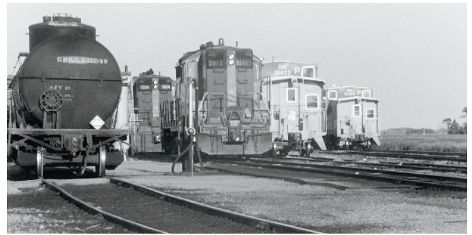
In the 1980s, locomotive servicing was done in the yard. The company-service tank car is loaded with diesel fuel. The sand column (partially obscured by the tank car) is in the background. Steve Grivno photo, Cody Grivno collection
