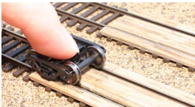
Fig. 4 Test flangeways. Here Jeff is using a freight car truck to check flangeway clearance. The top of the wood planking should be slightly below the railheads.
