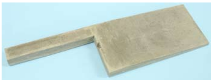
Fig. 8 Rough casting. Here's the rough casting as it comes from the mold. You can see the small recess Lance cast into the ramp to clear a flatcar's coupler.
