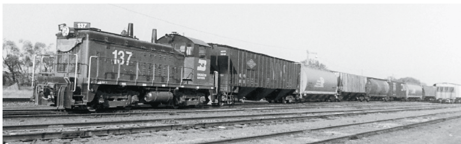
By the early 1970s, 50-foot hoppers and boxcars were the industry standard. To maintain capacity with the larger cars, BN added tracks five and six (foreground) to the Crookston yard. Steve Grivno photo, Cody Grivno collection
