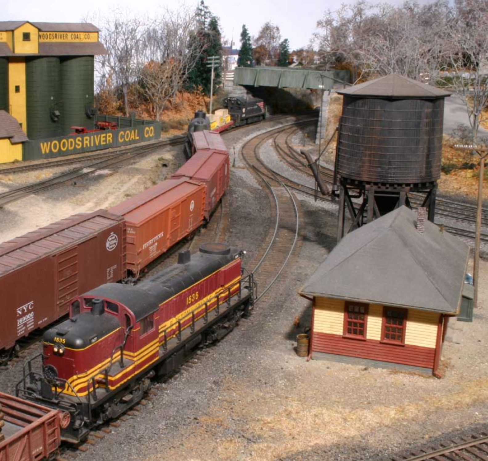
Fig. 3 Yard lead. The Woodsriver Yard lead is a separate track that runs parallel to the main line so switching can continue as other trains arrive and depart. The train in the foreground is departing to the south. Over the hood of the 1535 is the crossover connecting the lead and arrival/departure tracks. The yard office is also located along the lead.
