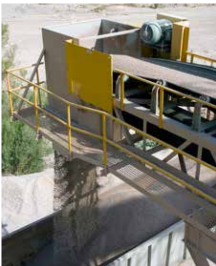
A conveyor shows crushed rock uniformity as it loads into a hopper at Capitol Aggregates' Marble Falls, Texas, quarry in 2008. Two photos, Forrest Becht
