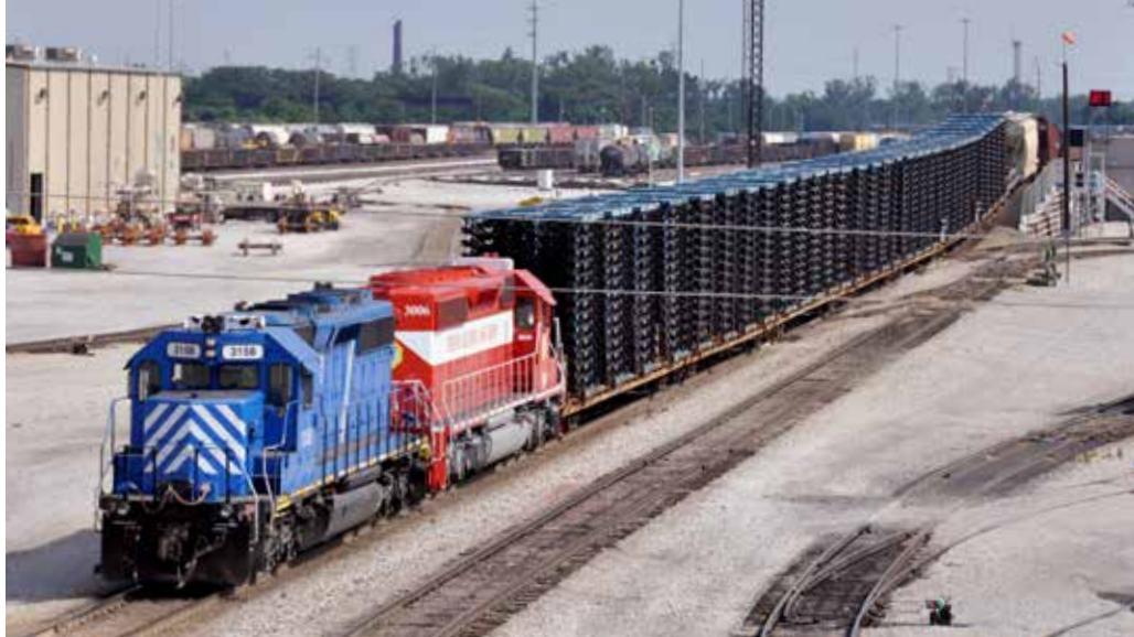
Two SD40-2s on the Terminal Railroad Association of St. Louis shove cars of vehicle frames over the hump at Madison Yard in Madison, Ill. Frames are just one example of the hundreds of auto parts that move by rail in containers, on flatcars, or in boxcars. Michael T. Burkhart
