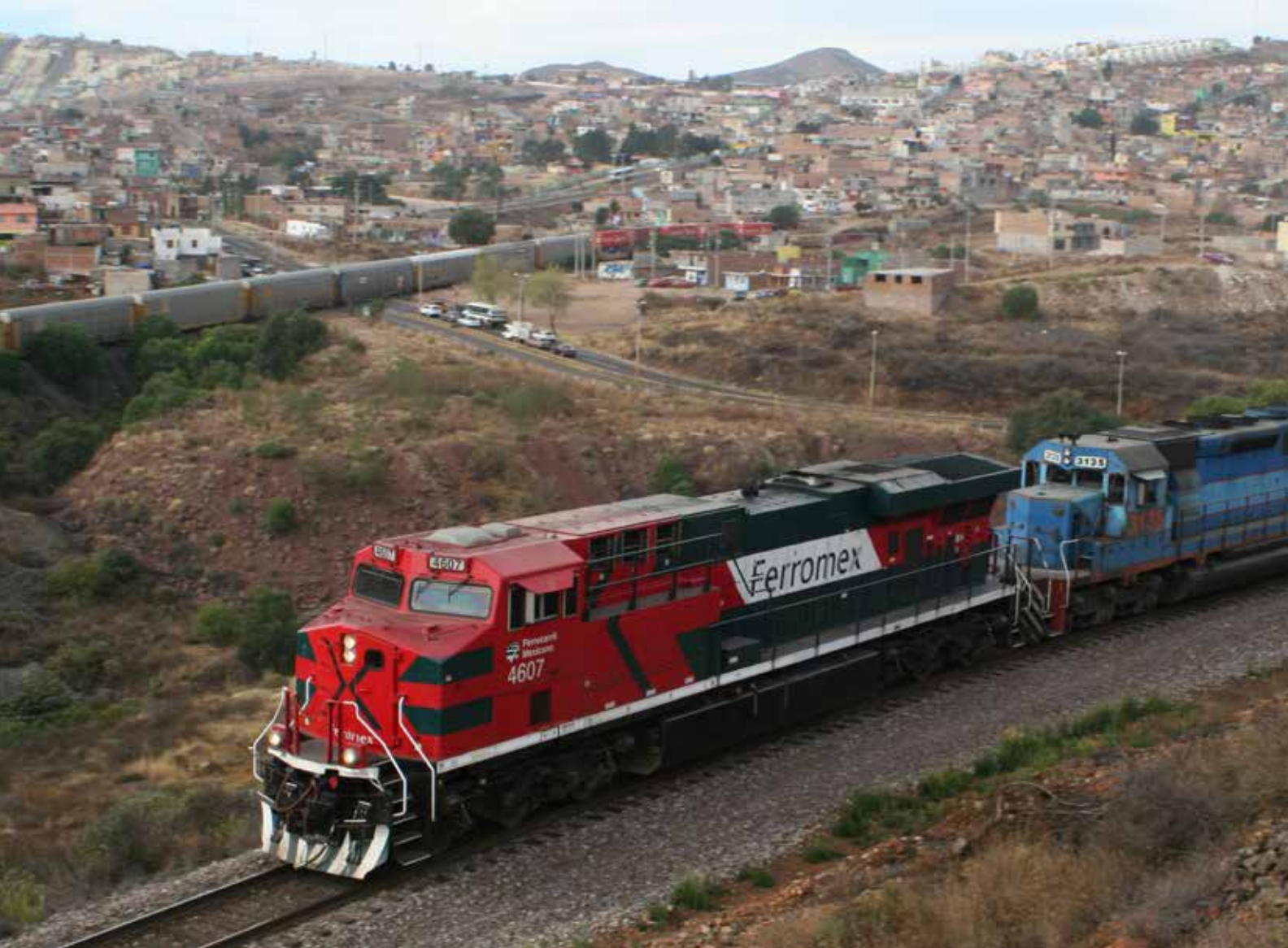
Ferromex ES44AC No. 4607 and SD40-2 No. 3135 lead a northbound Ferromex train of empty and loaded auto racks, auto parts box cars, and double-stack containers climbing the steep grade toward a summit in urban Zacatecas, Mexico. Nathan Muhlethaler
