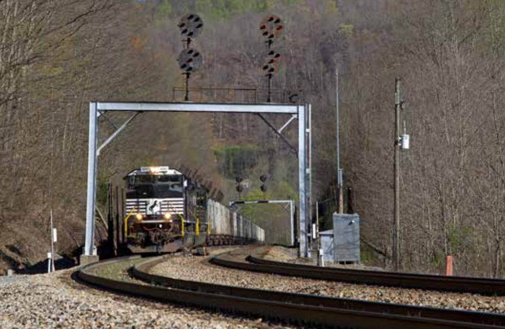
Running beneath classic Norfolk & Western color position light signals in the heart of coal country, a Norfolk Southern unit coal train rolls through Maybeury, W.Va. Samuel Phillips
