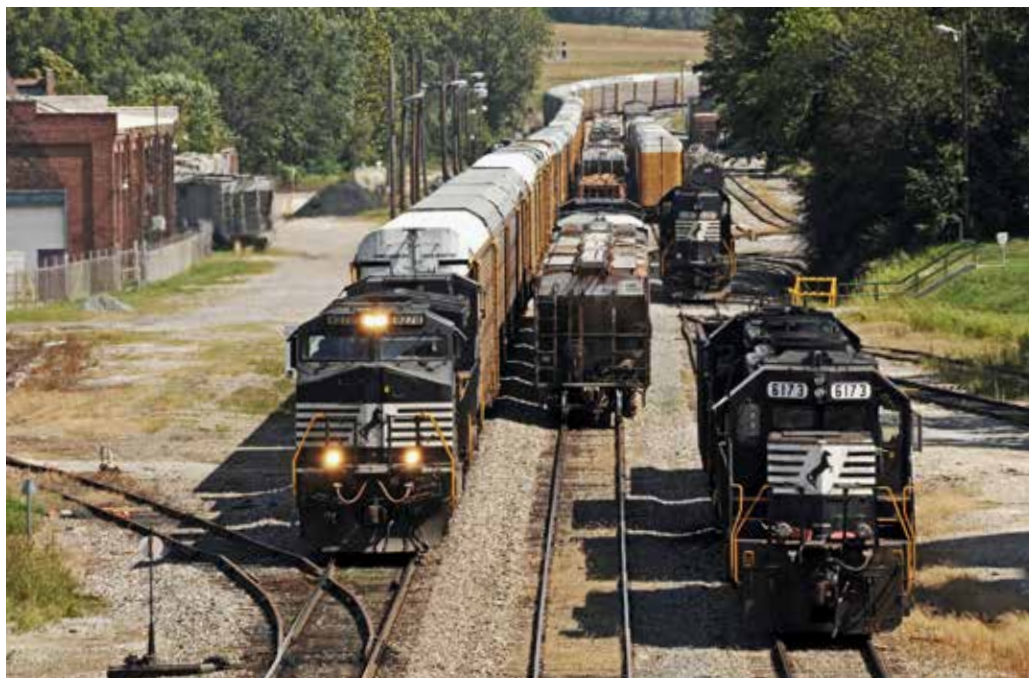
A Norfolk Southern auto rack train departs Princeton, Ind., on Sept. 13, 2008. The Toyota auto plant in Princeton ships out bilevel auto racks of minivans and SUVs. Most auto racks are limited to 55 mph to avoid damaging the vehicles inside. Michael S. Murray
