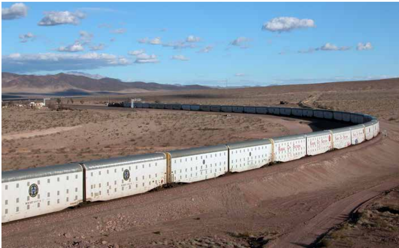
Articulated Auto-Max cars (seen heading east on BNSF at Ludlow, Calif., in 2004) are a common sight on BNSF vehicle trains moving to and from West Coast ports. These largest-of-the-large carriers can hold as many as 26 compact cars. Harold Riley
