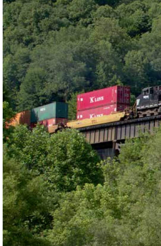
NS train No. 233 crosses the magnificent Coopers Trestle, near Bramwell, W.Va. Completion of the Heartland Corridor project allows double-stacks on the former Norfolk & Western main line. Samuel Phillips
