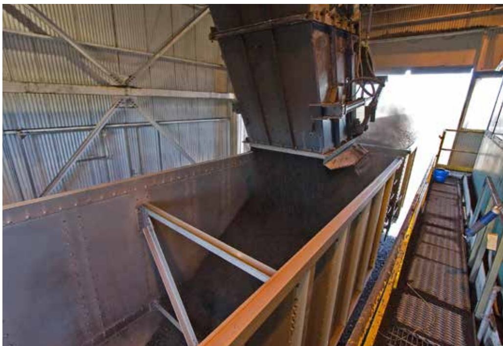
A wisp of dust materializes as coal pours into another Powder River Basin unit train. Mines have changed their loading patterns to mitigate coal dust flying off cars and settling on railroad tracks. Typical loaded unit coal trains weigh in at 15,000 tons. TRAINS: Mike Yuhes
