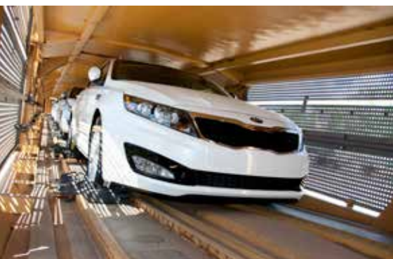
Kia Optimas will leave their Georgia birthplace by train in the lower level of a trilevel CSX auto rack. Special wheel chocks keep vehicles in place. Frank Orona
