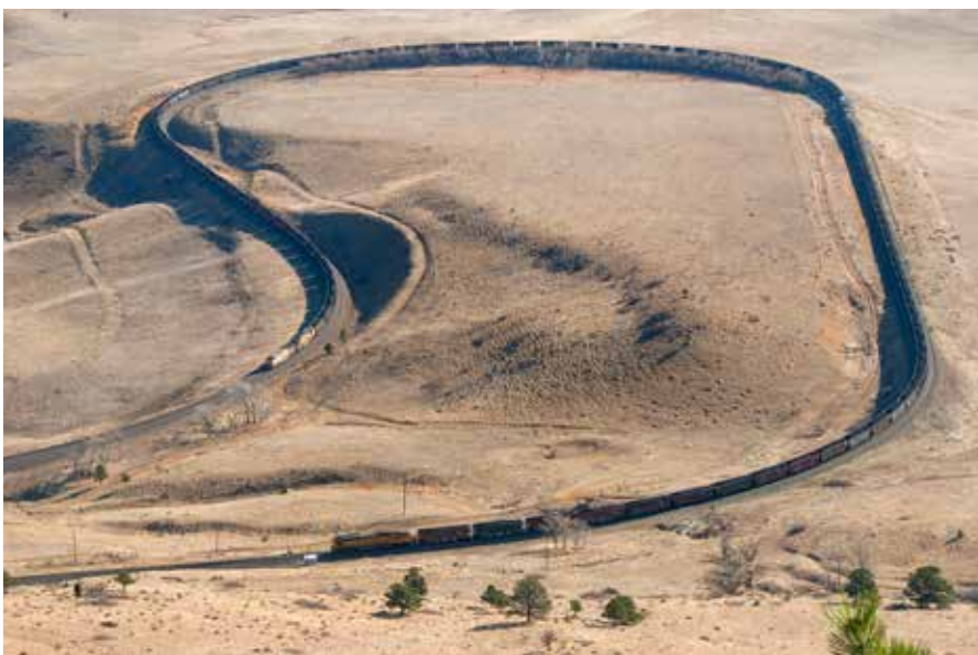
Second to BNSF in coal volumes, Union Pacific, shown here descending the Rockies at Clay siding on the famous Big Ten Curve near Denver, relies on distributed power to move its coal. Two units are up front, three are mid-train, and one is on the rear. Chip Sherman
