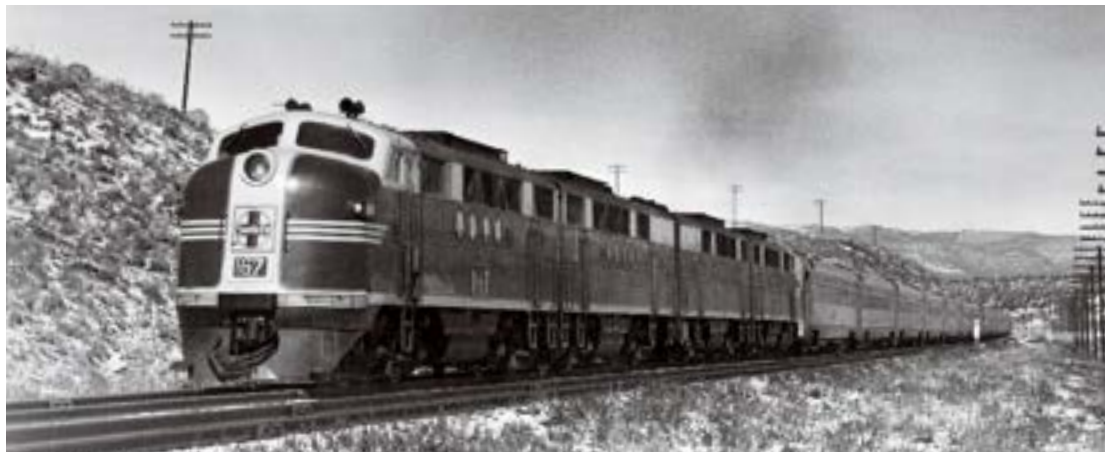
A four-unit FT set, still wearing blue-and-yellow freight colors, ascends Raton Pass with the El Cap on November 19, 1945. Previously, steam helped E units up this grade.
