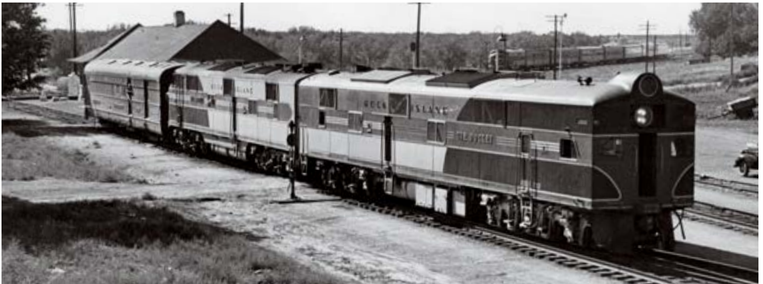
2 /// The Springs section's AB6 and E7A pull ahead with the mail-express car. EMD built only two AB6s, both for this service.
