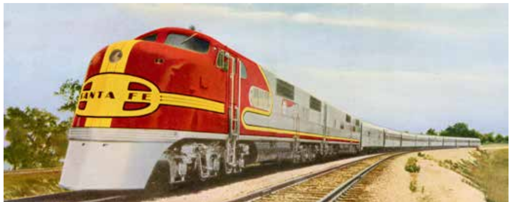
Diesel No. 2 missed the streamlined Super Chief 's debut, taking the reins a month later. Underneath their streamlined styling and Warbonnet livery, and above their A1A trucks, the E1A-E1B duo was internally similar to the original Super 's box-cabs.
