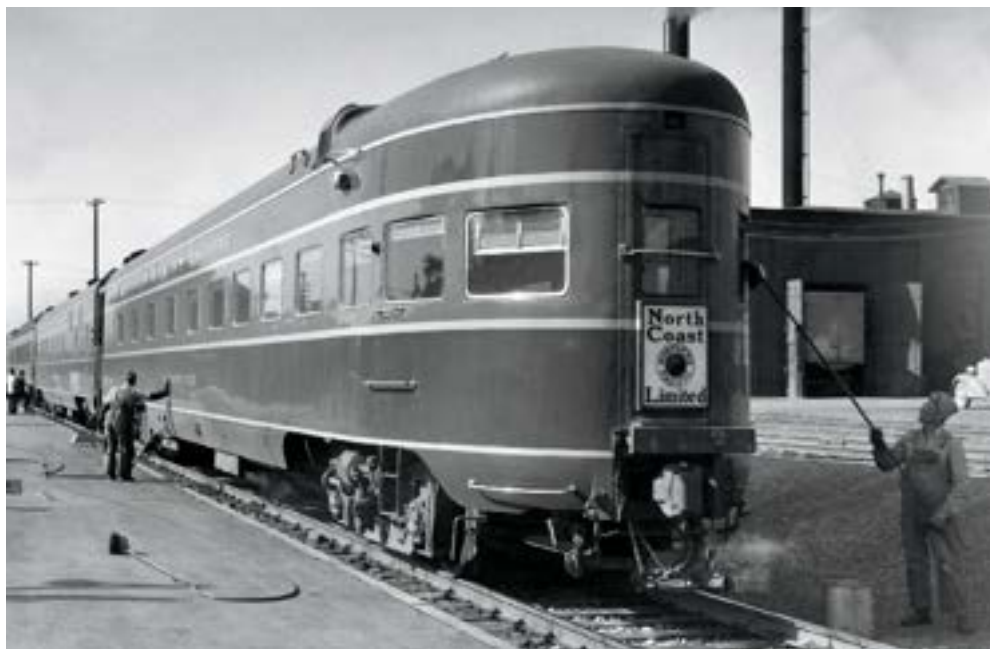
Workers at Butte service the westbound North Coast not long after the delivery of the train's streamlined Club-series observation cars, built in 1948 by Pullman-Standard.
