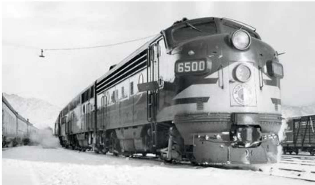
A metal blue flag hung on F3 6500 ensures that the train will not be moved while carmen work around and under the cars. This is Butte, one of several places the North Coast was delayed by the loading of sacks of Christmas mail on December 16, 1951.
