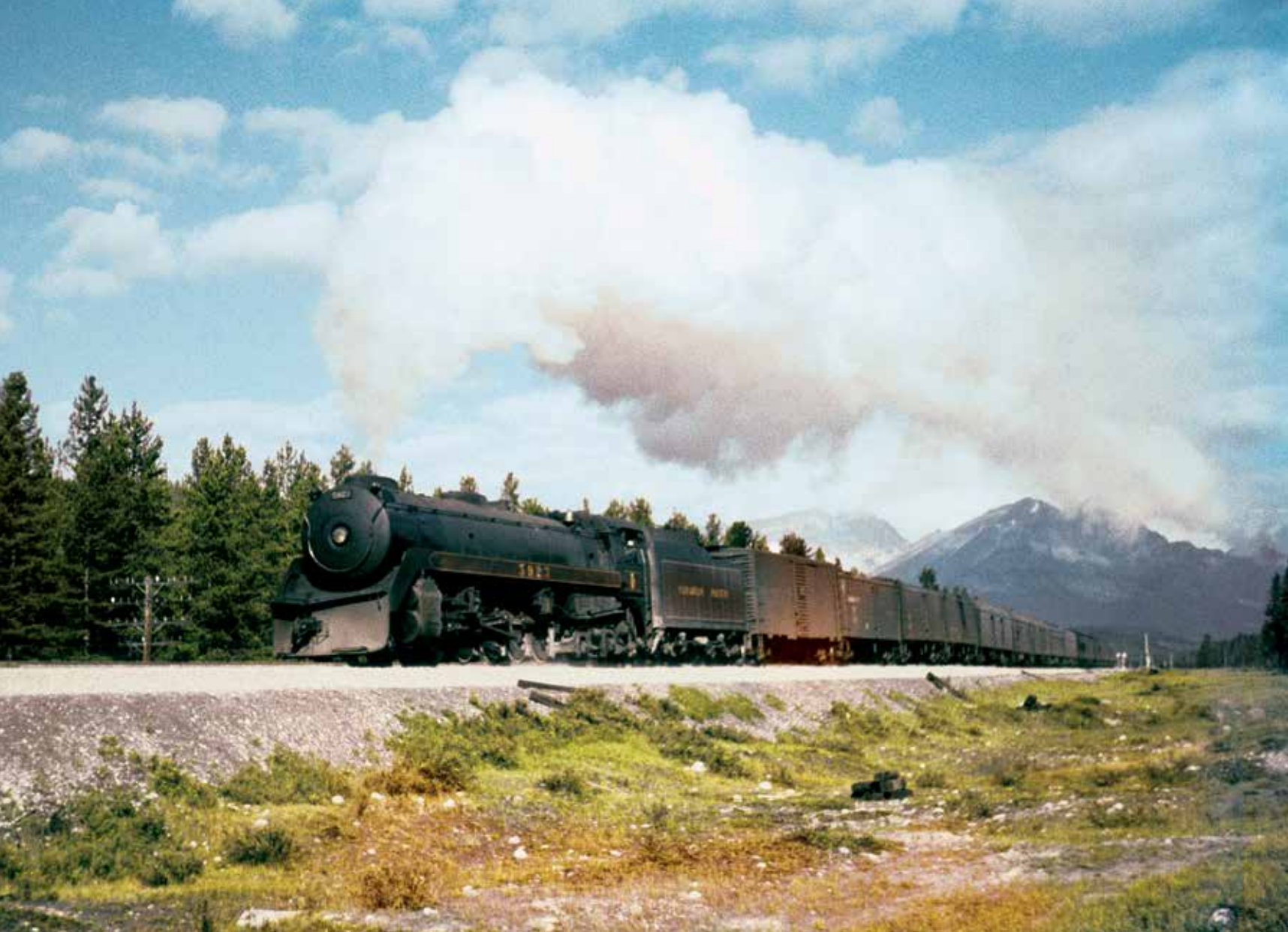
Selkirk 5923 accelerates a long Dominion west out of Banff in July 1948. CP's 16 semi-streamlined T1b and T1c 2-10-4s, built in 1938 and '49, were the largest steam locomotives in Canada.
