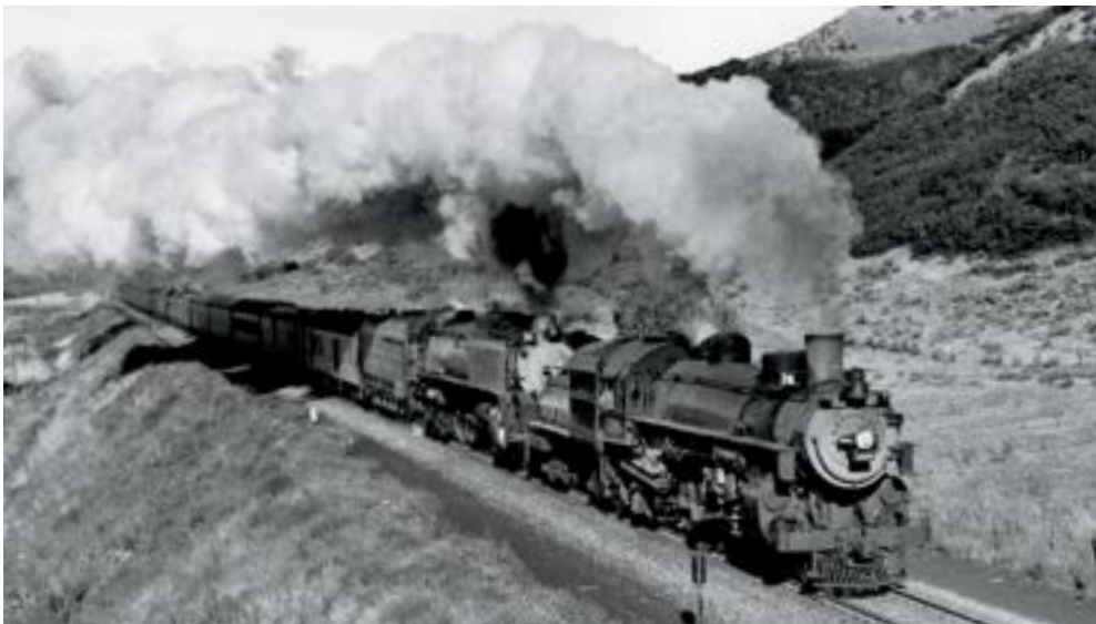
On October 10, 1946, the Overland's 4-8-4 has been given a 4-6-2 helper for the long climb from Ogden to Wahsatch. The pair rushes uphill at Uintah, 7 miles east of Ogden.
