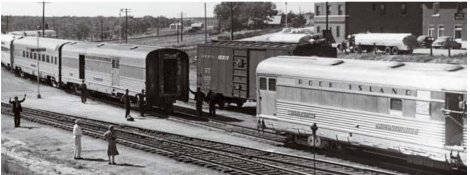
6 The mail-express car from the Springs is backed toward the Denver train's baggage car on hand signals from the conductor.
