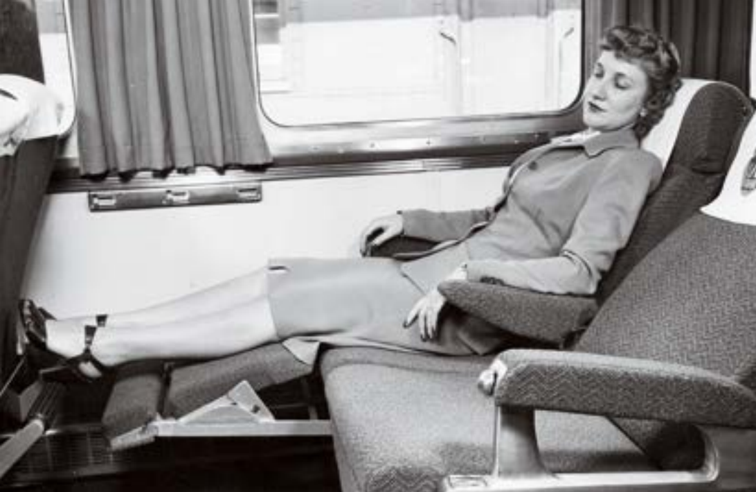
Chairs in the postwar El Cap 's roomy 44-seat coaches reclined, lined up with the windows, included leg rests, and accommodated a six-foot man in relative comfort.
