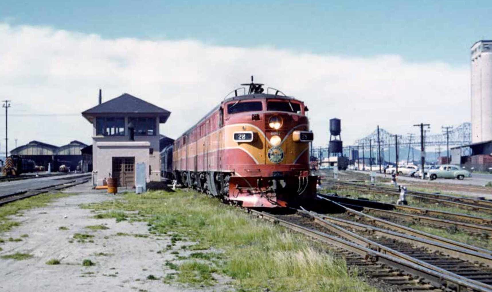
A three-unit set of 2,000 h.p. Alco-GE passenger units (a PA, PB, and PA in later parlance) awaits the San Francisco Overland's departure time at SP's Oakland Pier station in March 1958. Seven years previously, author Morgan's train also had PA-PB-PA power.
