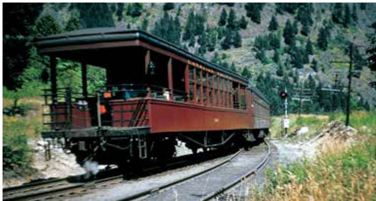
CP's 16 mountain obs cars in service during the 1920s–50s, like this example, were rebuilt from old wooden "colonist" sleepers. A final 3, converted from steel coaches, entered service in 1956.
