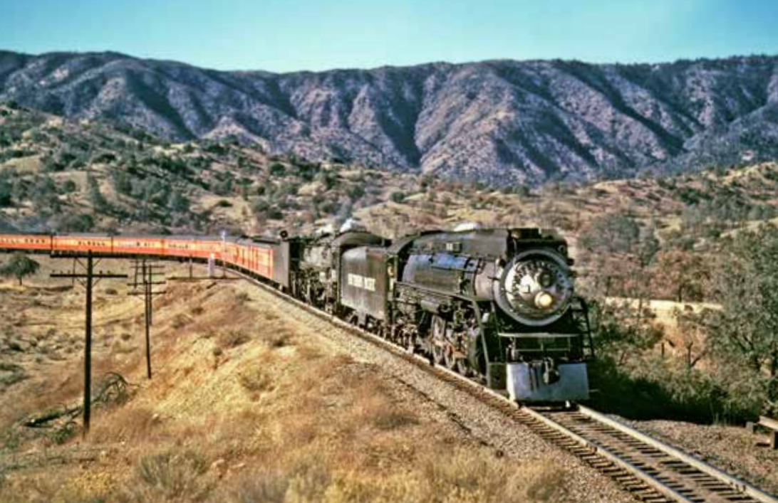
An unusual combination of a GS 4-8-4 and AC 4-8-8-2 heads the Los Angeles–Oakland San Joaquin Daylight through the Tehachapi Mountains in December 1952. Standard SJD power between L.A. and Bakersfield was two class Mt 4-8-2s or a 4-8-2/4-8-4 pair.
