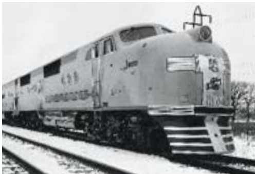
The E2 diesels (left) for the 1937 City of San Francisco and City of Los Angeles were a big step away from the custom power of the early streamliners, although their bulbous noses were unique. In 1941 the two California trains received standard E6 units (right). Above two photos, CLASSIC TRAINS collection; below, Joe Welsh collection
