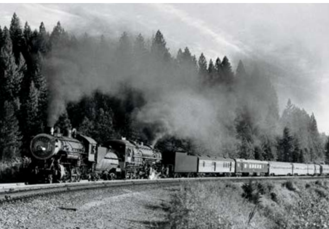
In the late 1940s, shortly before diesels took over on the SP portion of the run, 2-8-0 2519 helps cab-forward 4-8-8-2 4268 lift the eastbound San Francisco Overland up Donner Pass. A green ex-Army hospital car clashes with the train's two-tone gray livery.
