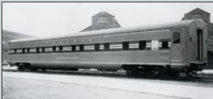
WESTCHESTER COUNTY: 13 double bedroom sleeper; one per typical consist; 8 built; County -series names.
