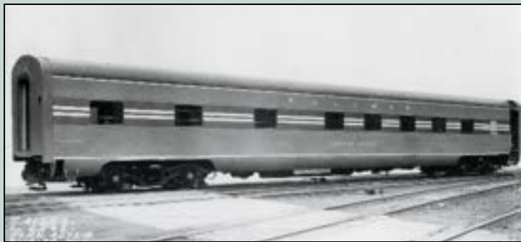
CASCADE VALLEY: 10-roomette/5-double-bedroom sleeper; two per typical consist; 12 built; Cascade-series names.
