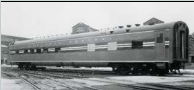
NO. 680: Dining car with kitchen and 38 seats; two per typical consist, coupled with dining areas adjacent; 6 built; Nos. 680–685.
