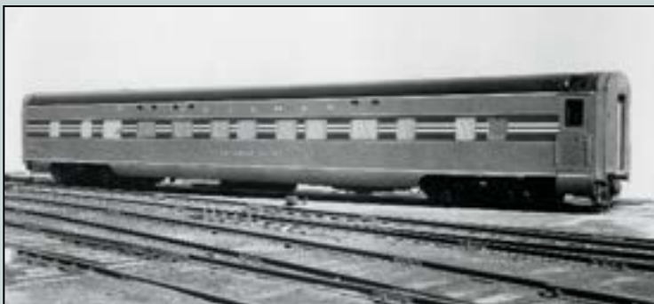
IMPERIAL COURT: 4-compartment/4-double-bedroom/2-drawing room sleeper; three per typical consist; 14 built; Imperial-series .
