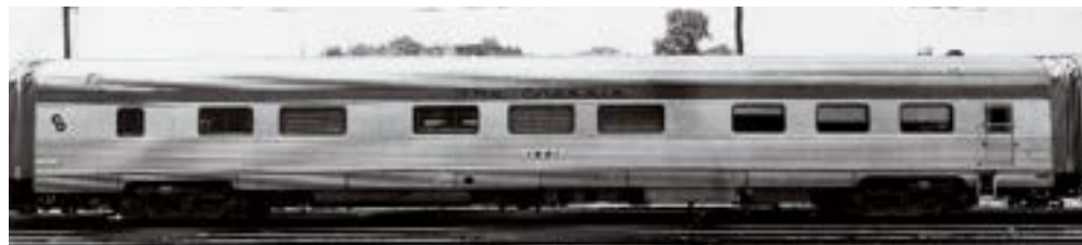
The Chessie's cars were standard Budd stainless steel, topped by yellow letterboards with the train's name in blue script. This is tavern-lounge-lunch counter car 1901.
