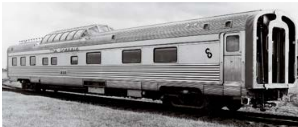
The Chessie's three "cabin-domes" were built with 6 roomettes for train personnel, 3 larger rooms ("cabins") of two sizes for passengers, and an operations center.
