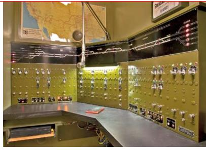
Here's the finished Centralized Traffic Contol machine Jay built for his HO scale P&SF, using panel fronts and other components salvaged from the prototype machine that once controlled the same P&SF line that he models.
