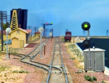
The "OS section" at the east end of Black is a typical remote-controlled interlocking in CTC. Including a powered turnout and three absolute signals, it's represented on the machine by a column of controls and indicator lights.
