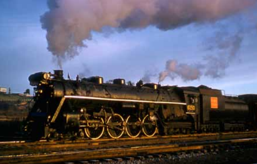
Canadian National was the first road to acquire 4-8-4's for dual (i.e., freight and passenger) service. U-2-c 6150, from CN's third (1929) group, catches morning light at Montreal in November '57.
