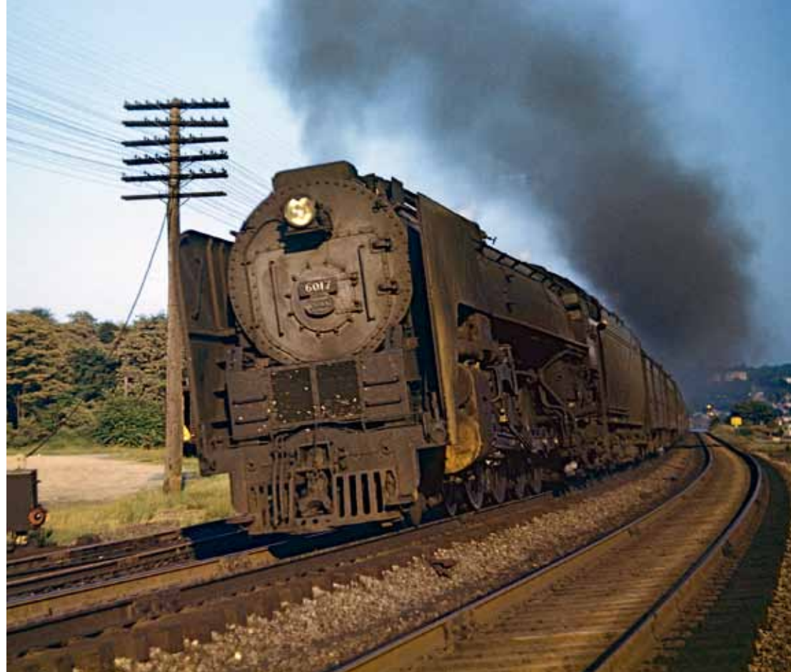
NYC S-1b Niagara 6017 (above) represents the ultimate in North American 4-8-4 development as it rushes up the Hudson River valley near Poughkeepsie, N.Y., with the Chicago-bound Pacemaker on October 8, 1946. The Central's first 4-8-4, HS-1a No. 800 of 1931 (right), was a complex experiment that didn't pan out.
