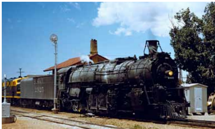
The Santa Fe 2900's were the heaviest of all 4-8-4's. Built to haul mile-long freights or 90-mph passenger trains, No. 2925 has been relegated to helper service as it arrives at Mountainair, N.Mex., after assisting F3 diesels up from Belen on July 1, 1956.
