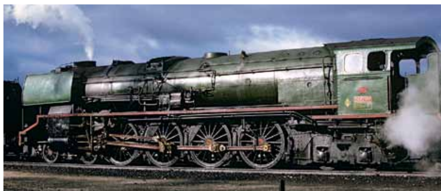
Spanish beauty: Like the Soviet P36, Spain's 10 4-8-4's were designed and built domestically. The 5-foot 6-inch-gauge oil-burners worked top passenger trains from 1955 until the early 1970s. Lanky No. 242F2007, doubleheading behind a 4-8-2 on a Madrid express, stands at Burgos in November 1966.
