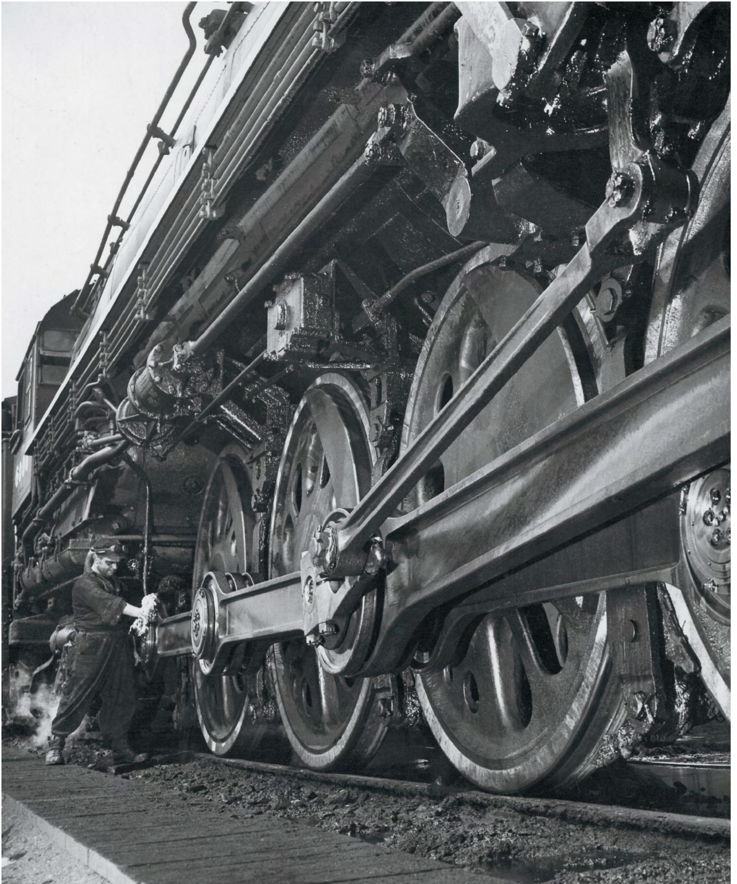
Rubdown for a Niagara: In a dramatic study of man and machine, a hostler polishes the manganese-vanadium side rods of New York Central No. 6000—the first Niagara. NYC's 26 S-1's, plus one poppet-valve S-2a, rank among the greatest of all 4-8-4 families.
