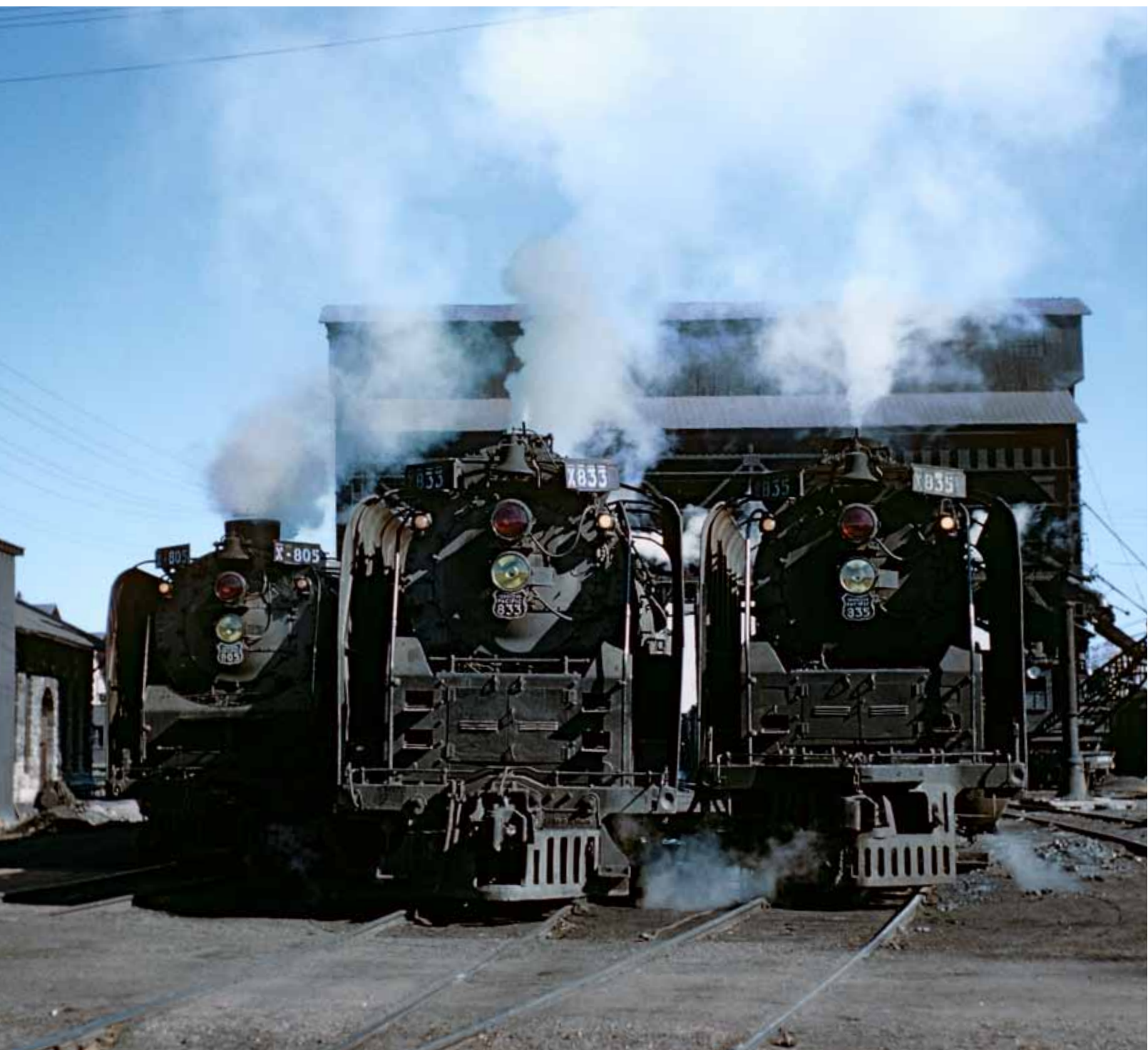
One of each: All three classes of Union Pacific 4-8-4's are represented in this October 29, 1958, lineup at Grand Island, Nebr. From left, we have FEF-1 No. 805, FEF-2 No. 833 (now displayed in Ogden, Utah), and FEF-3 No. 835. UP had dieselized its Nebraska main line and retired this coal dock, but, in a 1958 traffic surge, reactivated the oil-fired 800's for Council Bluffs–North Platte freight work.
