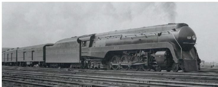
Norfolk & Western 613, the final 4-8-4 built in North America, departs Cincinnati with the Cavalier for Norfolk, Va., in May 1952. Like NYC's Niagaras, N&W's J's could top 5,000 drawbar h.p.
