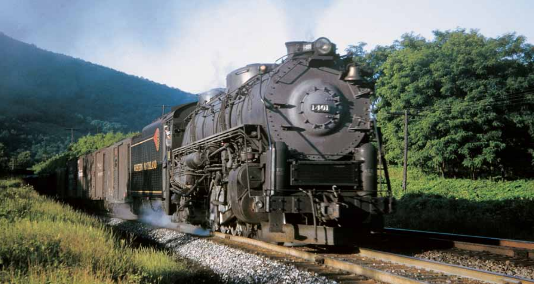
The great girth of the boilers on Western Maryland's 4-8-4's is apparent in this view of No. 1401 making time with a hotshot at Cumberland Narrows, Md., in 1952. The low-driven Potomacs were ideally suited for their duties, but led unfortunately short lives.
