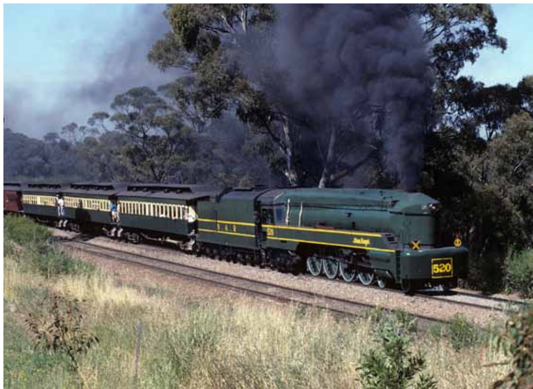
PRR Down Under: South Australian Railways' dozen class 520's, homebuilt in 1943–47, borrowed the styling of the Pennsylvania's T1 4-4-4-4 of 1942. The 520's worked SAR's 5-foot 3-inch-gauge lines until late 1966; two survive, including the class leader, pictured on a 1993 fantrip.
