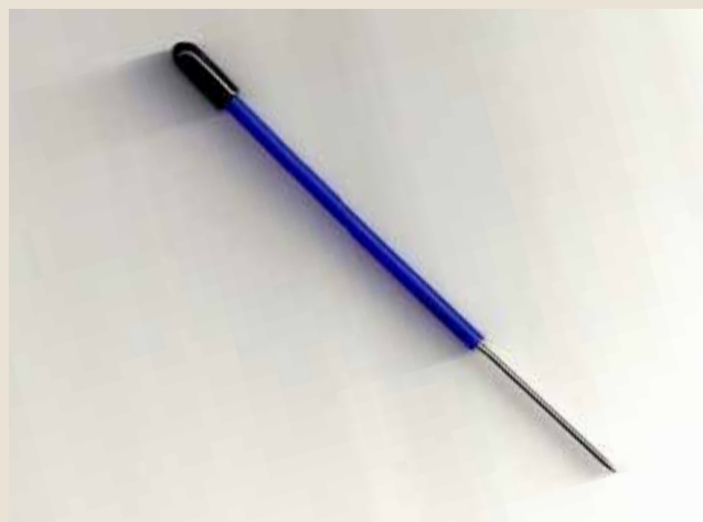
Russ removes the trip pins from his Kadee knuckle couplers, since he doesn't use magnets. Instead he uncouples cars with this tool, made from a tapestry needle inserted into a grip made from a length of plastic tubing. Tony Koester photo
