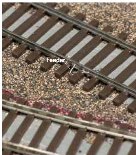
Fig. 8 Soldered feeder. The small diameter feeder wires solder easily to model railroad track. Once this section is painted and ballasted, the feeder will be hard to notice.
