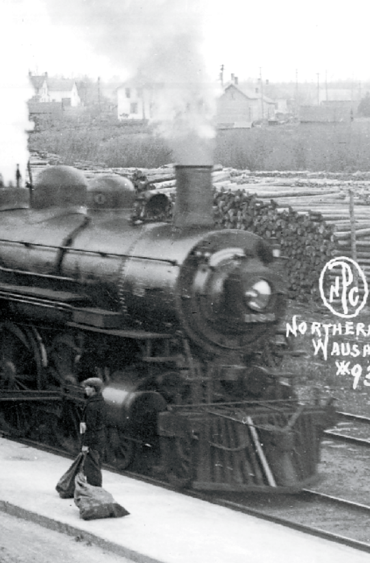
One of the C&NW's high-drivered class D Atlantics (4-4-2s) pauses briefly at Wittenberg, Wis. This is the sort of compact but glamorous motive power Iain had in mind when designing this track plan. Photo courtesy Chicago & North Western Historical Society
