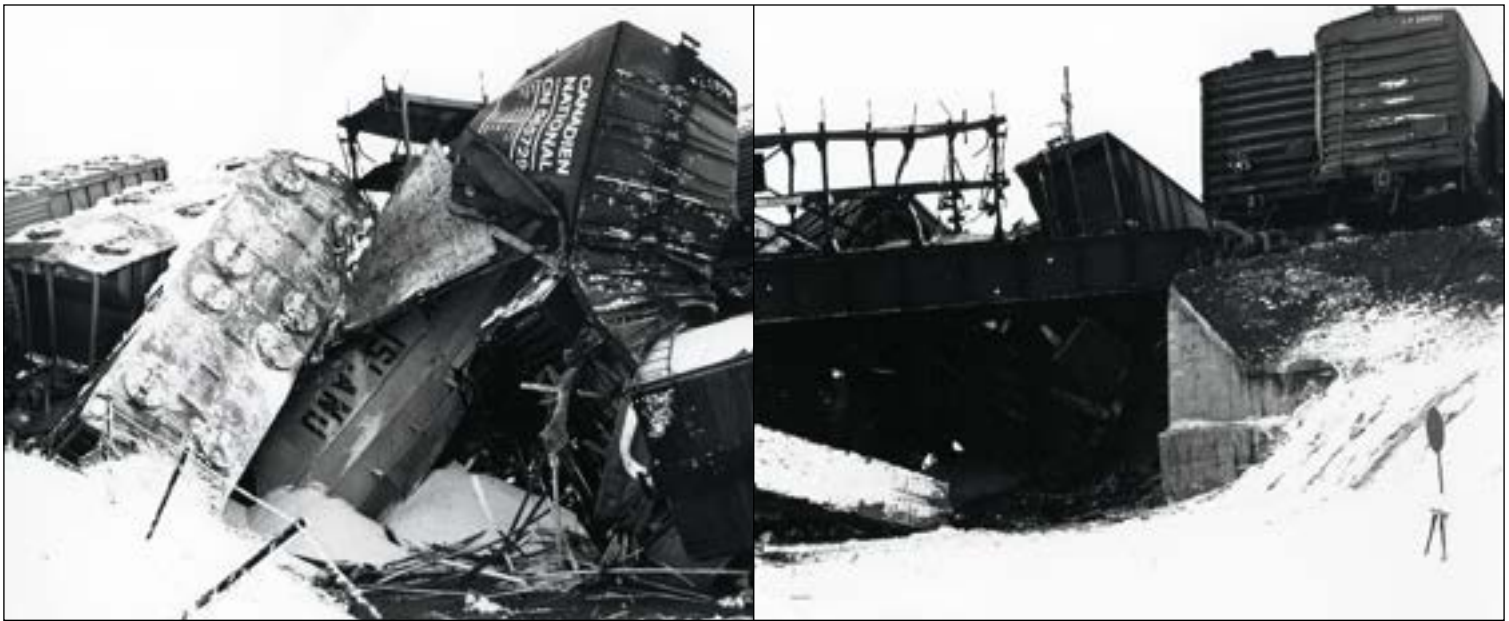
The wreck resulted from the second car on 812 derailling and striking the deck girder bridge over GTW's Cass City Sub ("PO&N") in Imlay City. Viewed from the PO&N track, we look south (left) at 7 of the 41 derailed cars filling the cut; the photo above looks north.
