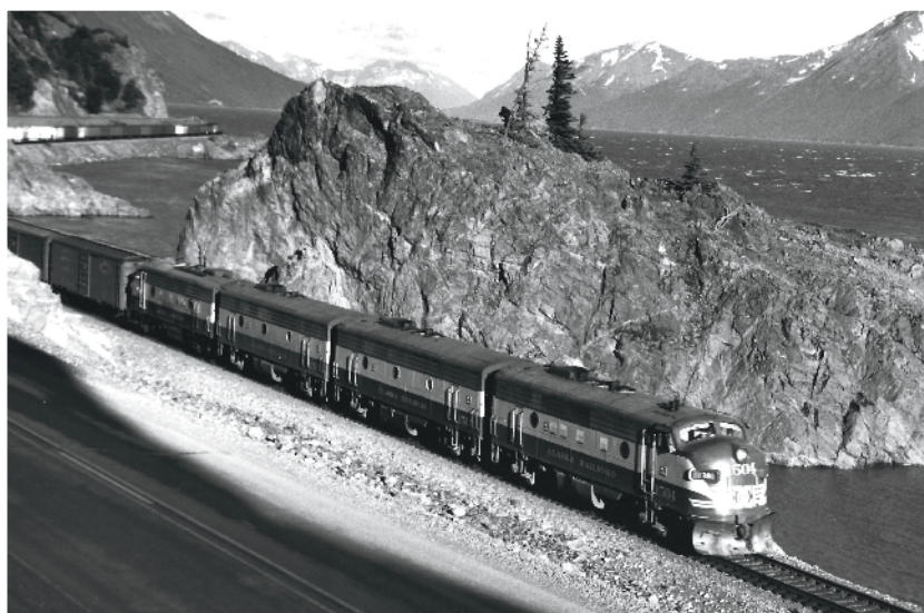
A typical 1960's freight train at Turnagain Arm between Seward and Anchorage. Four A-B-B-A units would be a typical example of head-end power. Usually there were a lot of SeaLand containers on flatcars in the consist. Mac's Foto
