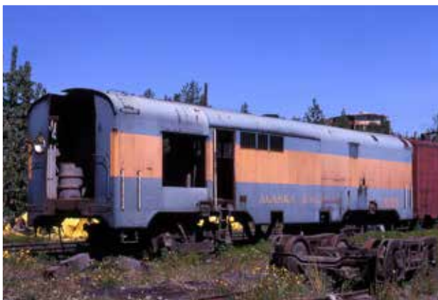
The carcass of an RF1B. The Alco RSD1 road switchers were rebuilt as A and cableless B units for a more streamlined look when coupled together. The shrouding protected the operating crews.
