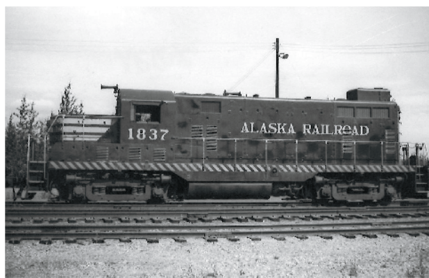
Alaska picked up a batch of U.S. Army EMD GP7s to supplement the RF1s in road service. They came with a homemade chop nose and AAR trucks. This one is at Fairbanks in July 1966. Carl P. Munck
