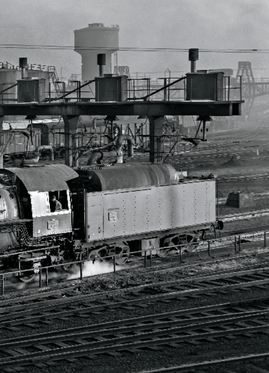
Baldwin-built 141R-797 shows off a Boxpox main driver on the service tracks at the huge Le Mans engine terminal on Aug. 19, 1964. The 141Rs shared freight duties with French-built 141Ps west of Le Mans.
