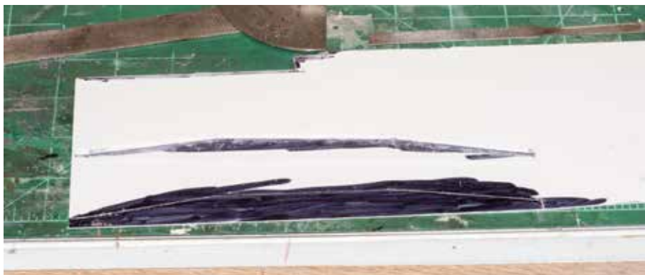
2 Center sills. Charles used a black marker to color the .060" plain styrene sheet used to make the masters for the center sills. The scribed outlines are easier to see against the black background.
