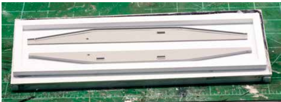
3 Building the mold. Next, Charles glued the finished center sills to a piece of .100" plain styrene sheet. He made the walls for the model from pieces of 1/4" square styrene strip.
