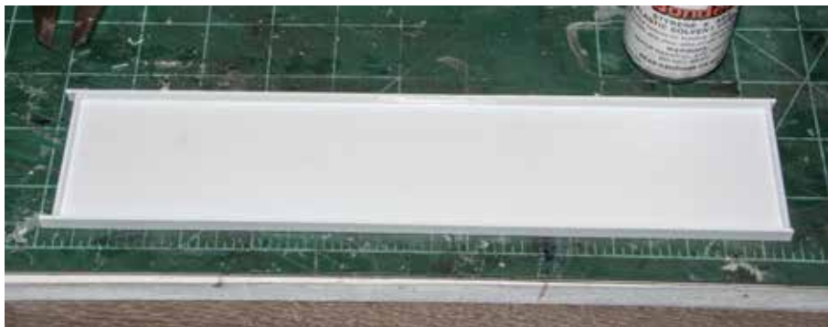
1 Taking shape. Charles used .060" plain styrene sheet for the sub deck and .100" x .250" styrene strip for the side and end sills. After the styrene cement dried, he cut the sides flush with the ends.
