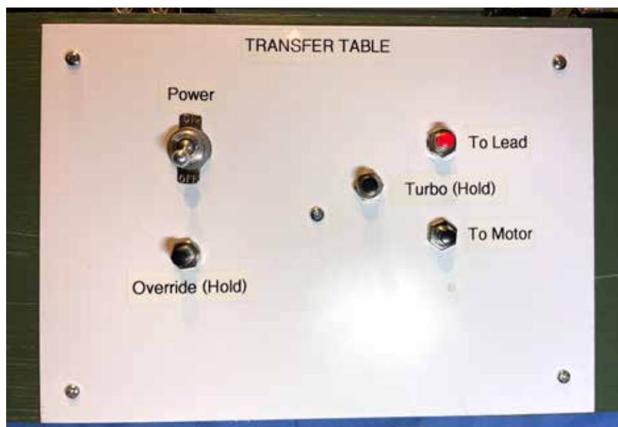
6 The control panel gives operators several options when controlling the transfer table. The “turbo” option moves the table at double normal speed when the button is held down.
