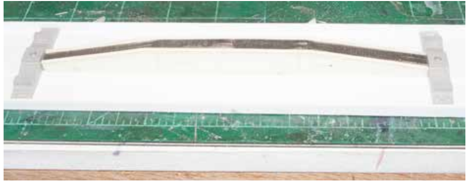
④ Attaching the sills. Weights from Scale City Designs are concealed between the cast-resin center sills. Charles attached the resin sills to the metal weights with cyanoacrylate adhesive.
