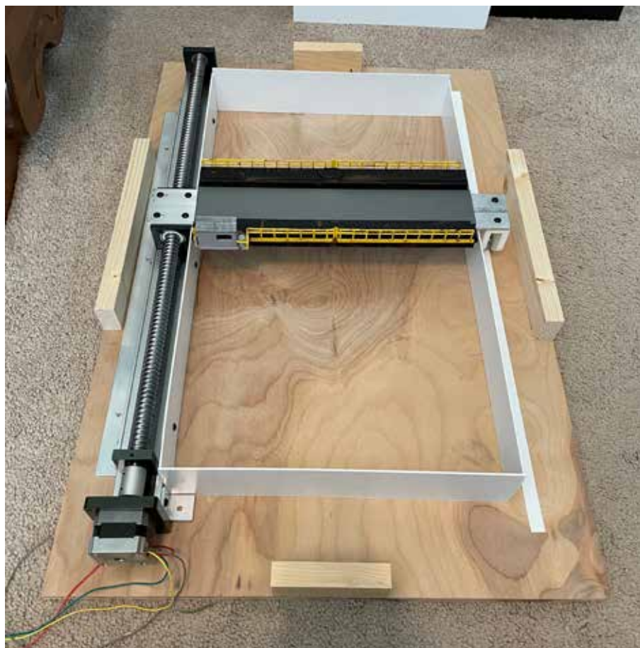
(2) The stepper motor and slide rail mechanism that moves the transfer table is shown mounted to 1/2"-thick furniture-grade plywood.
