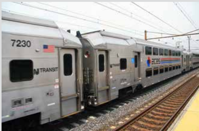
NJ Transit commuter cars feature two levels despite restrictive tunnel clearances. This equipment was modified for an express service to Atlantic City, N.J., in 2009.
